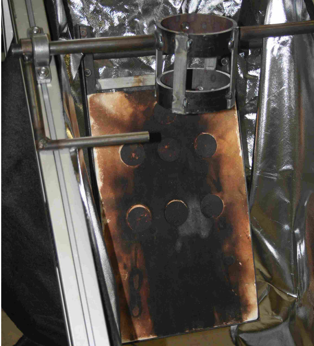
Figure 2-3: Test apparatus used for obtaining data in accordance to ASTM 955 test for assessing the performance of fabrics subject to hot liquid splashes.
