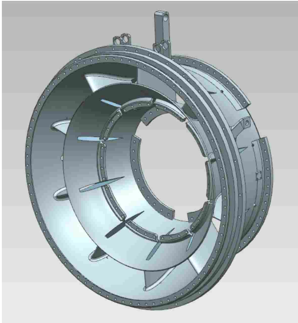
Figure A.2: An intermediate case for a jet engine modeled in NXConnect
