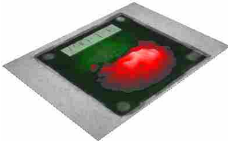
Figure 2-6: Operational mode shape of blower face at 6.75 kHz
