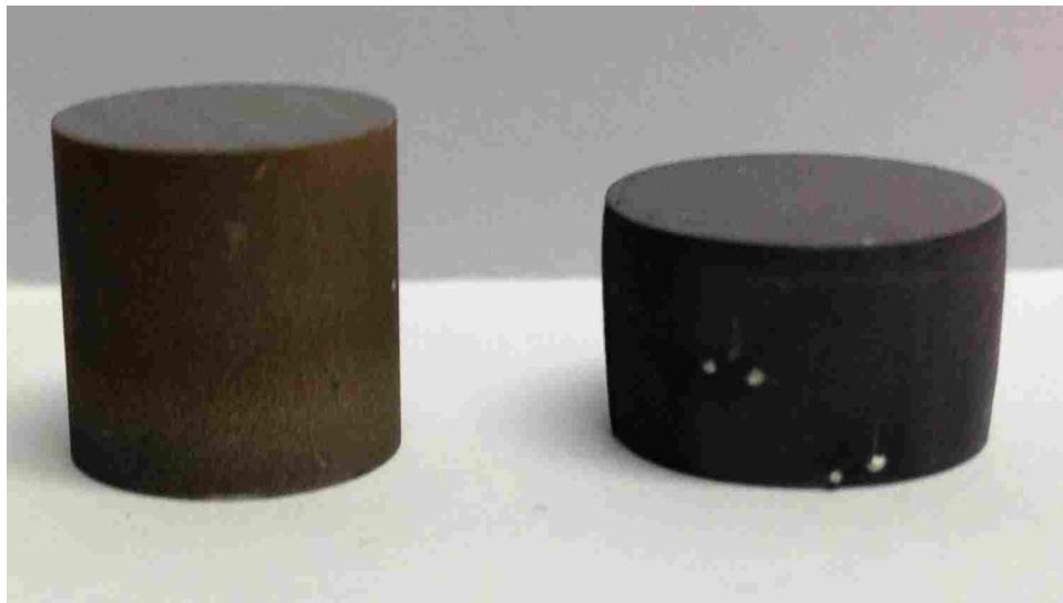
Figure 3.1: Picture of two high temperature compression test samples. The one on the left has not been tested. The right sample has been compressed 30% as part of the hot temperature compression test.
