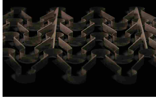
Figure 2.4: Sample mesh example after KOH release and rinse
