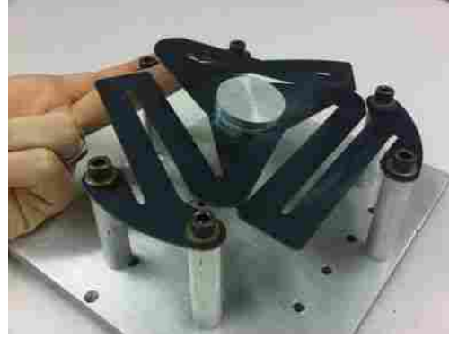
(b) Ortho-planar spring with central pointing platform. The platform can be tilted at each corner for three DOF (two rotations and extension).
