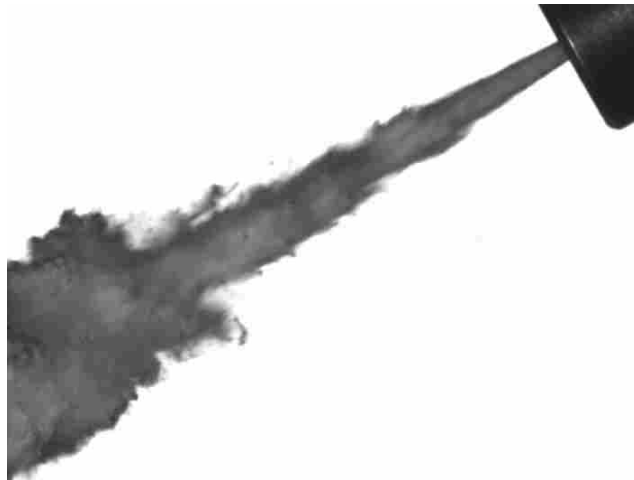
(a) Cavitating water jet: 1.0 mm nozzle, 20.7 MPa
