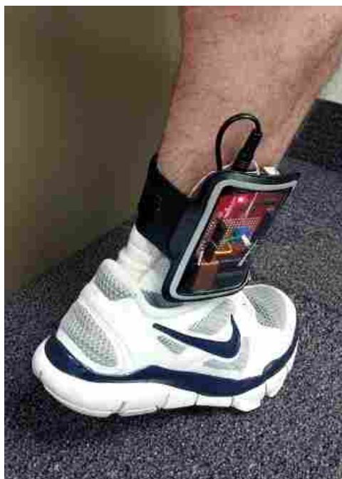
Figure 3.5: The sensing insole system attached to the leg of a subject.
