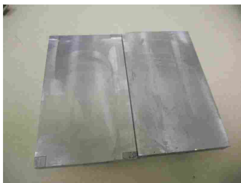
Figure 1.10: The flat plate mold has legs approximately 0.34 mm tall.
