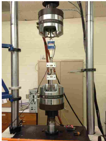
Figure 1.23: The microcontroller is attached to the Instron to measure NCSG response to displacements.
