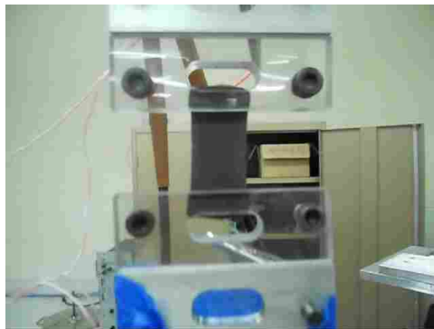
Figure 1.17: The NCSG is placed in the Instron in plastic non-conductive grippers.
