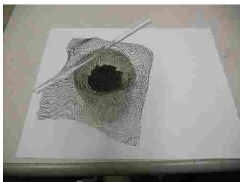
Figure 1.4: The screen mesh with a glass rod and cup to hold the screened NiNs
