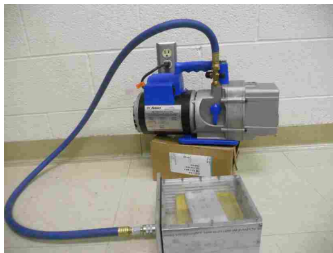
Figure 1.7: The vacuum and vacuum chamber configured to vacuum extra air out of the composite material
