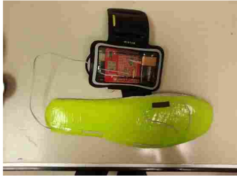
Figure 3.6: The sensing insole system with one strain gauge.
