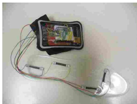
Figure 3.4: The sensing insole is depicted with wiring and the Arduino Uno microcontroller.
