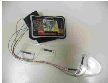
Figure 1.16: The insole system with four gauges embedded into the silicone base. The microcontroller is attached to the embedded gauges.
