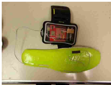
Figure 1.14: The insole with a NCSG duct taped to the bottom to gather data.
