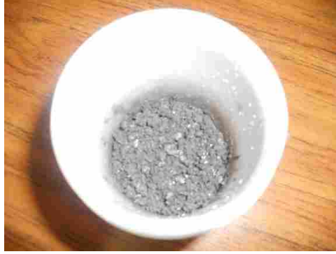
Figure 1.6: A plastic cup holding Silicone, NiNs, and NCCF that are to be placed in the Thinky.
