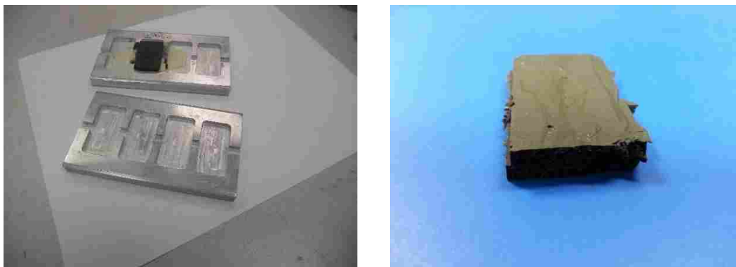
Figure B.1: The two female molds after the foam is expanded and the molds are separated (left). The conductive foam made from using two female molds pressed together (right).
