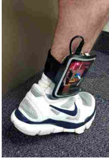
Figure 1.15: The microcontroller is attached to the ankle of the subject with wires traveling under the insole.
