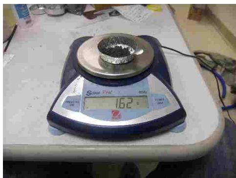
Figure 1.5: 500g scale with an Aluminum cup and screened NiNs.
