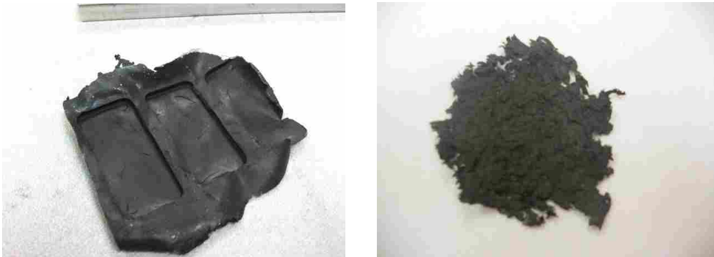
Figure 1.9: The gauge formed by the mold process (left) and the scraped method (right).
