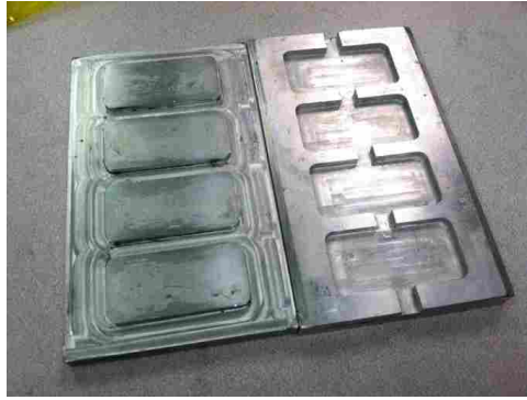
Figure 1.8: The Aluminum mold with the female portion of the mold on the left and the male portion on the right.
