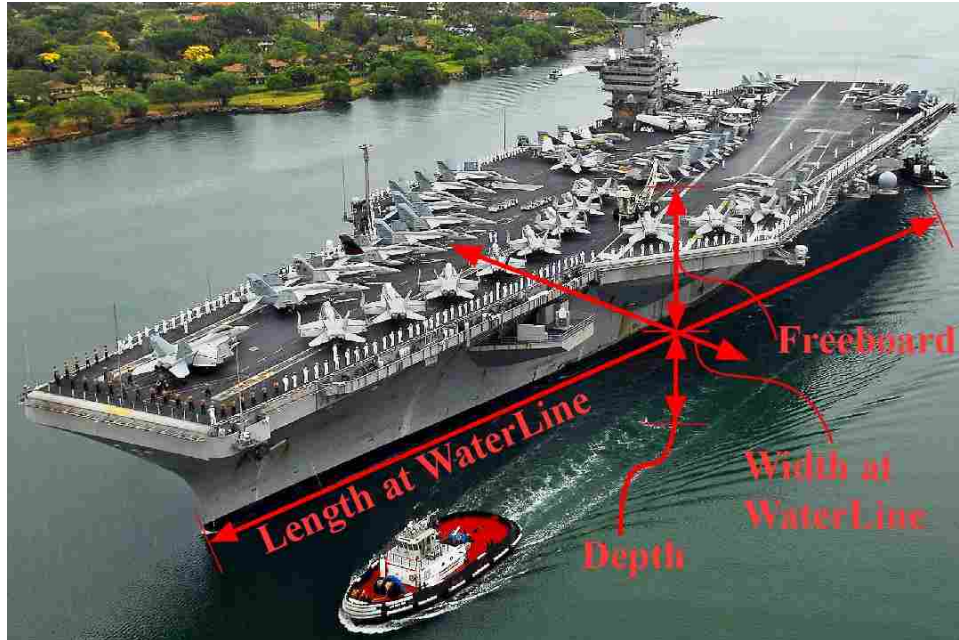
Figure B.1: Display of hull dimension of nuclear aircraft carriers (USS John C. Stennis [1])
