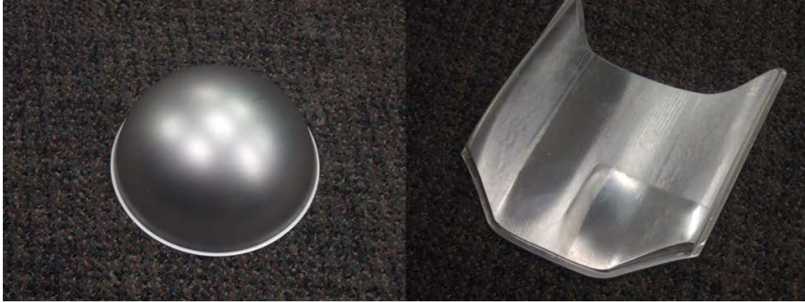
Figure 5-1: 6 Inch Hemisphere and Scale Dodge Viper Hood Molds
