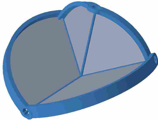
Figure 3.1: Origami vertex (shown in grey) with an equivalent rigid-body spherical mechanism and the axes of its revolute joints (shown in blue).
