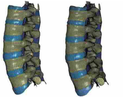
Figure 3-3: Mesh and Double Mesh for Stress Convergence
