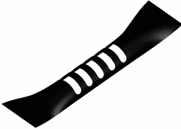
Figure 2.12: The Torsional U-form Flexure.
