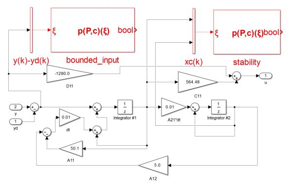
Figure 22: Control system annotated with open-loop stability
