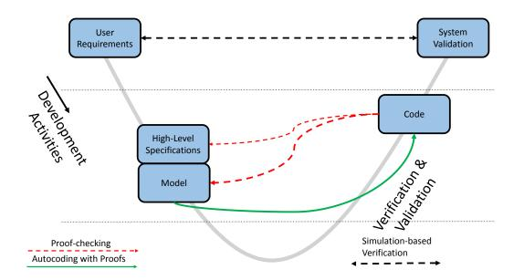
Figure 10: Safety-critical software development process with credible autocoding
