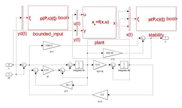
Figure 13: Control system model annotated with control semantics
