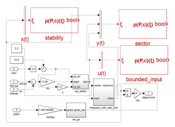
Figure 14: Sector-bound condition for saturation operators in an altitude controller
