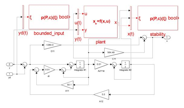
Figure 21: Control system annotated with closed-loop stability
