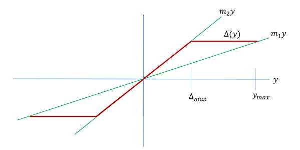
Figure 1: Approximating saturation function with a sector-bound inequality
