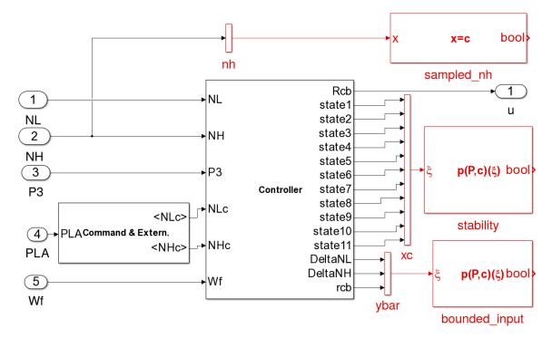
Figure 12: Simulink Model with annotation blocks
