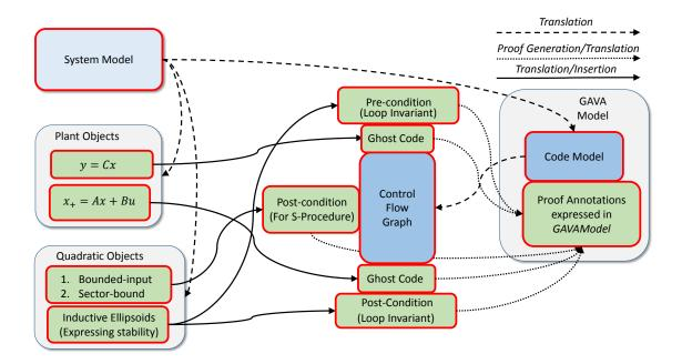
Figure 24: Transformation of control semantics from GASystemModel to GAVAModel
