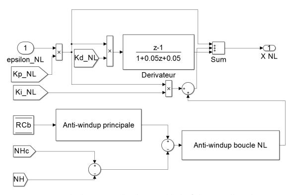
Figure 39: Inside the "PID NL" subsystem block of the controller subsystem
