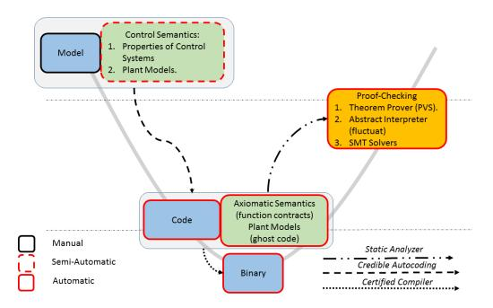
Figure 11: Automated Credible Autocoding/Compilation Chain for Control Systems
