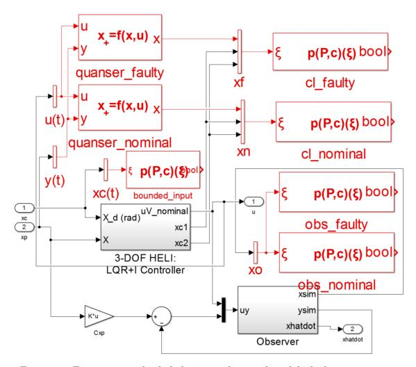
Figure 15: Expressing multiple behaviors: observer-based fault-detection system
