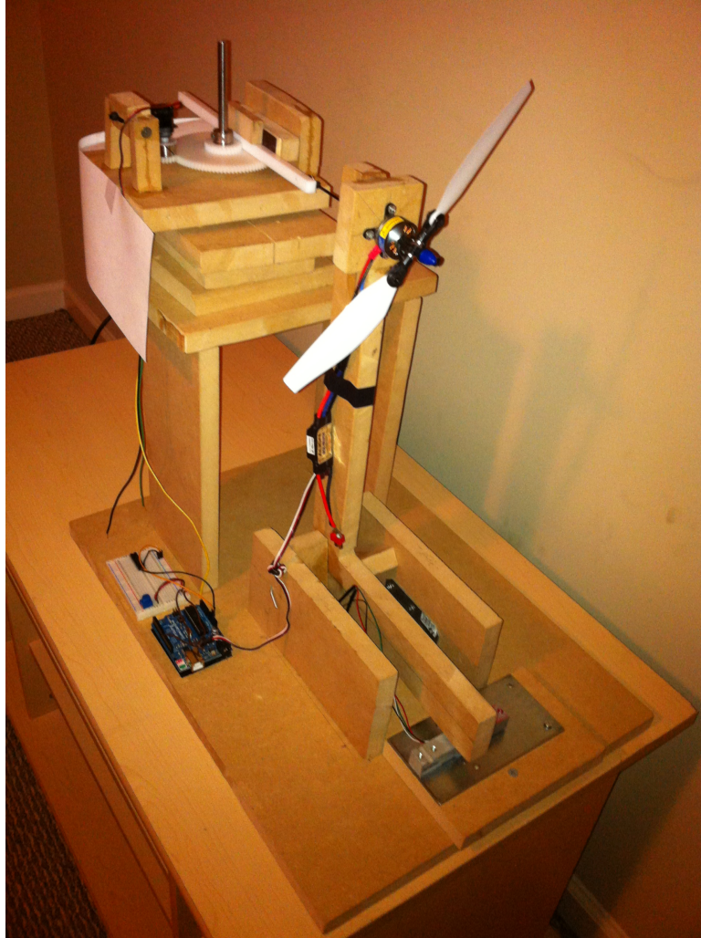
Figure 16: DC motor with variable pitch system hardware
