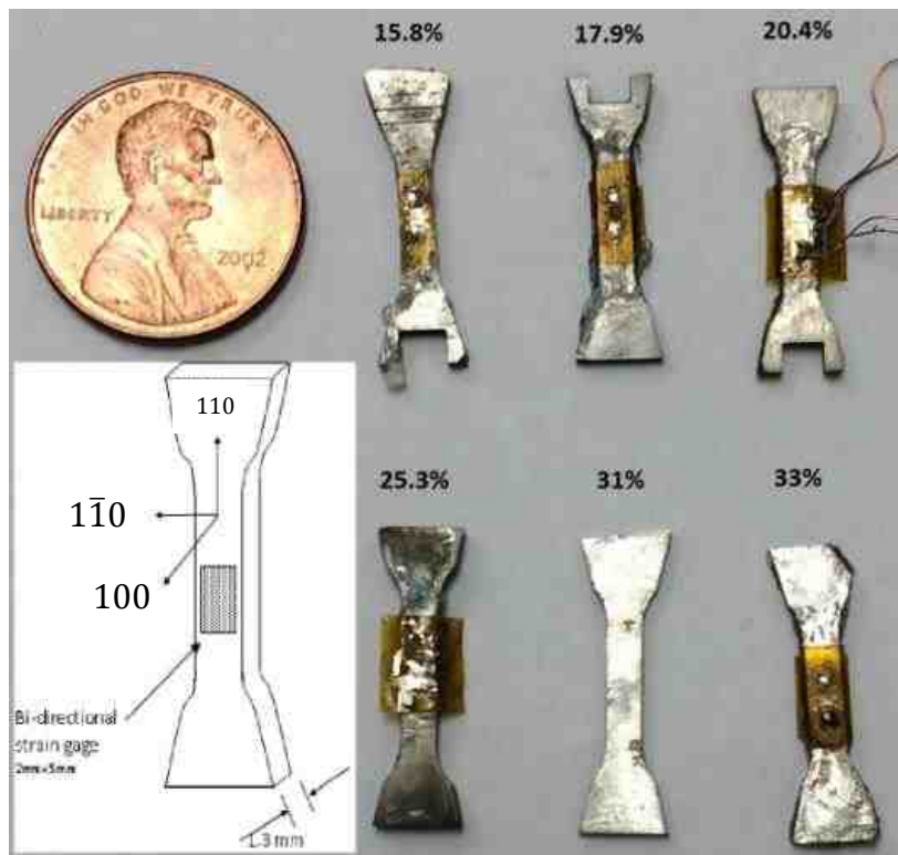
Figure 3.2: Photo of typical Fe-Ga dogbone samples and a sketch depicting crystallographic axes and strain gauge placement on a sample.
