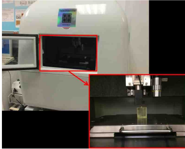
Figure 4.39: Experimental setup of the nano-indenter experiment. Inset: Sample mounted on epoxy offset (without permanent magnet).
