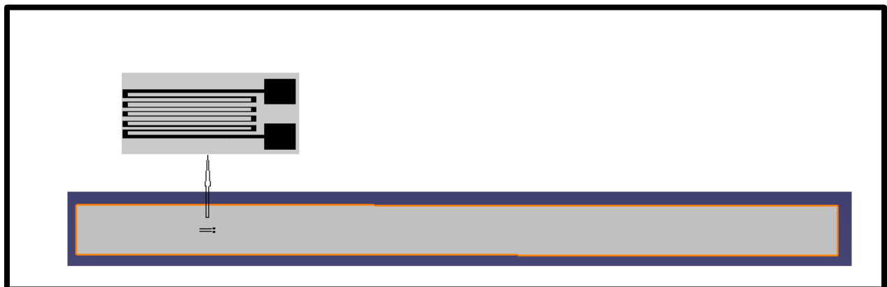
Figure 50: Schematic of strain gauge placed on cantilever beam. Exploded view of the sensor is shown in the inset
