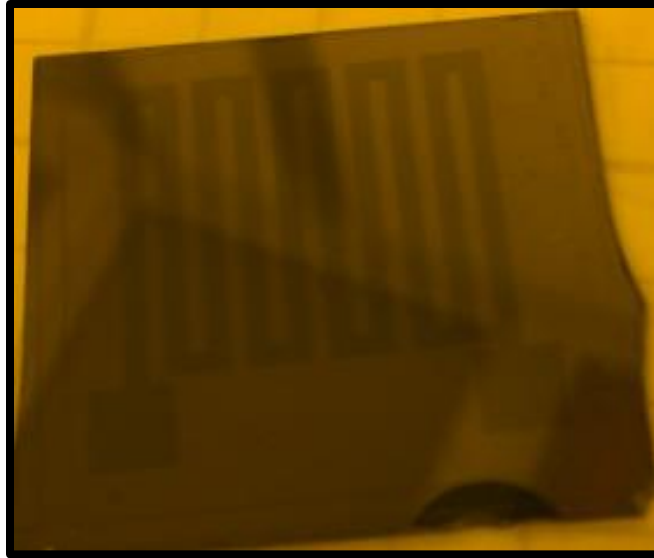
Figure 44: Schematic of SiO 2 substrate after etching photoresist
