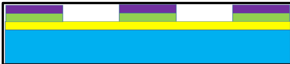
Figure 41: Cross sectional view after etching Nickel
