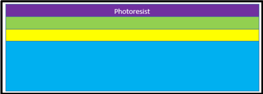
Figure 33: Cross-sectional layout of Silicon substrate with photoresist
