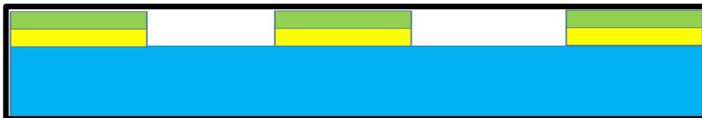
Figure 43: Cross sectional view after etching Photoresist (second time)
