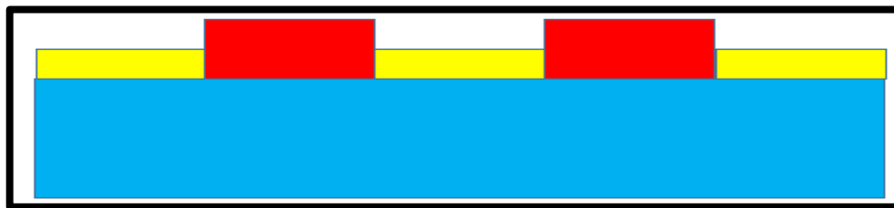
Figure 46: Cross-sectional view after etching nickel (second time)
