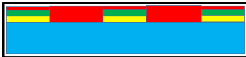
Figure 45: Cross-sectional view after spin coating with CNT-polymer composite
