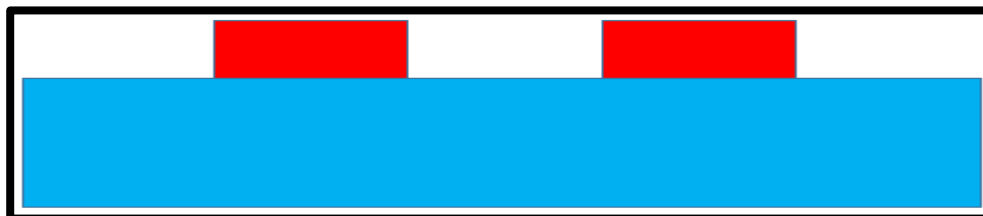
Figure 47: Cross-sectional view after etching titanium (second time)
