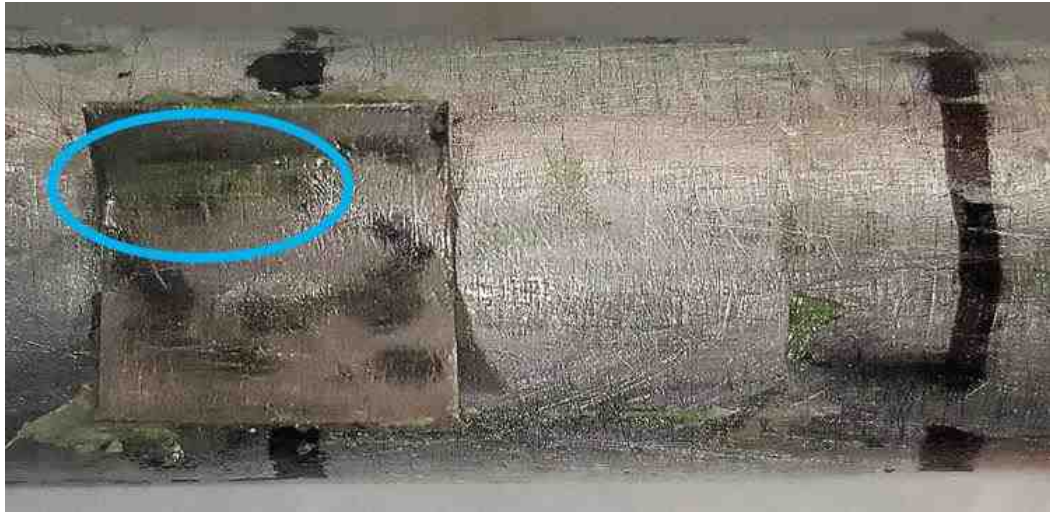
Figure 3.16: Repeatability test case 9 demonstrated a pooling of adhesive in a structural deformation present in the shim patch.
