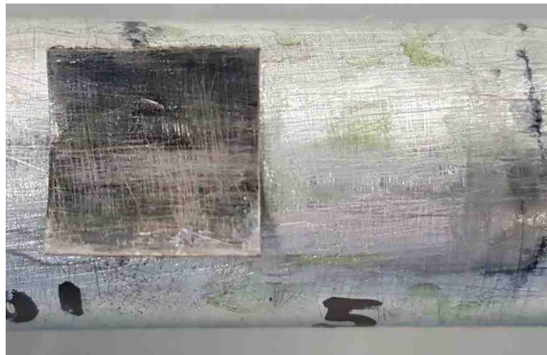
Figure 3.15: This image shows the steel shim after debonding to examine bond layer thickness. A uniform bond layer formed around the edges of the shim when sanded with 60 grit sandpaper, using a 15 in-lb applied torque with 0.05 mL of Loctite 648 applied evenly to the bottom surface of the shim.
