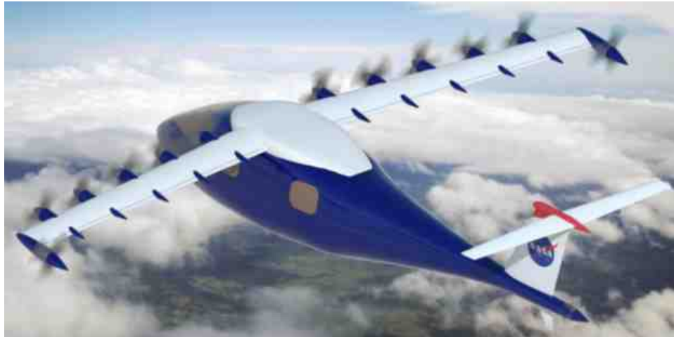
Figure 2.1: NASA Leading Edge Asynchronous Propellers Technology (LEAPTech) DEP concept 1
