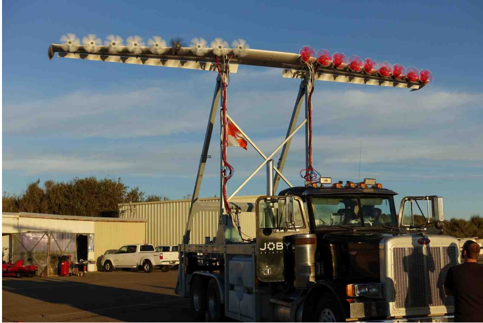
Figure 2.5: The LEAPTech aircraft wing under truck test. Credit: Joby Aviation
