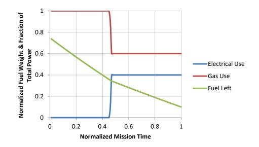
Figure 13: Notional Mission Using Battery at End
