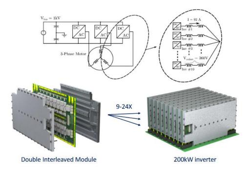
Figure 15: Scalable Inverter Module from UIUC[60]
