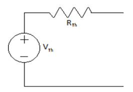
Figure 30: Thévenin Equivalent Circuit Battery Model
