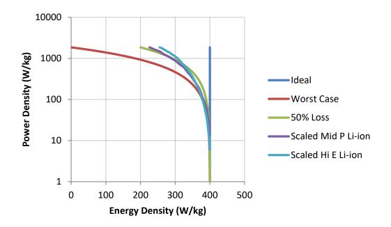
Figure 32: Alternative Ragone Curves for Lithium-Sulfur Batteries 78
