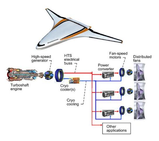
Figure 7: NASA N3-X Concept and Subset of Propulsion System[8, 31]
