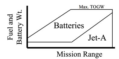
Figure 5: Battery and Fuel Weight Vs. Range[19]
