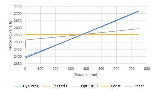
Figure 40: Experiment #1 750 nmi. 35,000 lb. Payload, 20,914 lb. Battery, .7 Mach, 37,700 ft.
