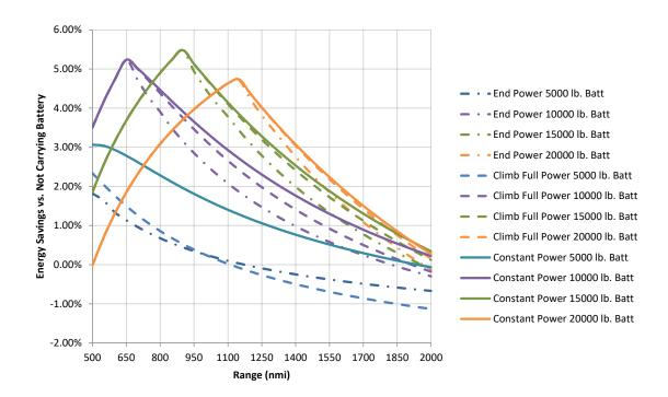
Figure 68: Energy Savings Carrying 25,000 lb. Payload with Different Battery Sizes and Baseline Schedules, 2000 Hp Motor
