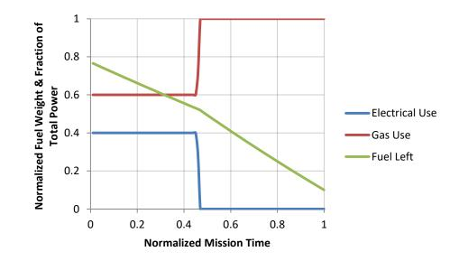
Figure 14: Notional Mission Using Battery at Start
