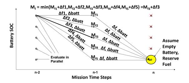
Figure 37: Parallelization in Dynamic Programming
