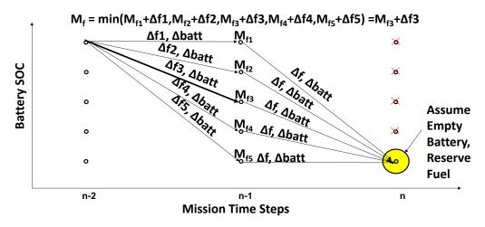
Figure 18: Optimal Path from Charge State 1, Time Step n-2, to End
