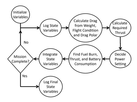
Figure 33: Mission Simulation Procedure
