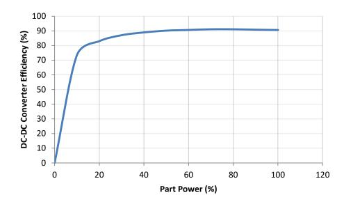
Figure 28: DC-DC Converter Efficiency Map[59]
