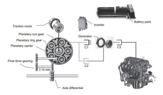
Figure 9: Voltec Electric Drive System from Chevrolet Volt [11]
