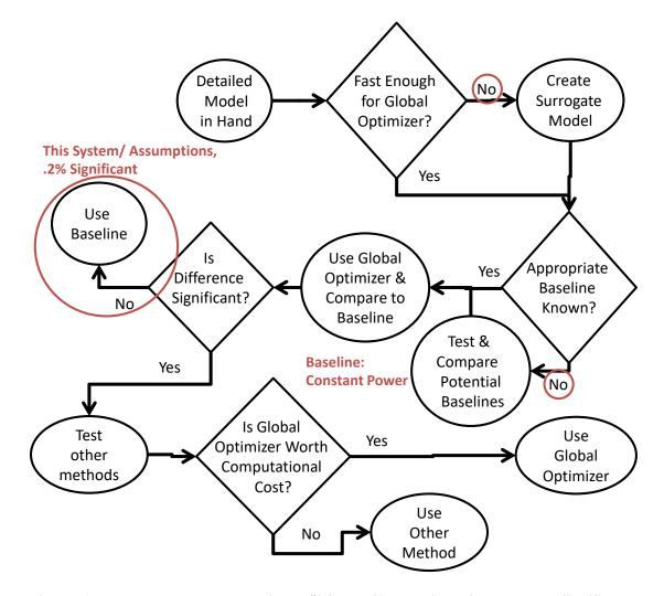
Figure 71: Procedure Example, Experiment #2 System/Assumptions, .2% Fuel Burn Significant
