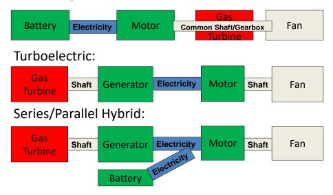
Figure 2: Hybrid Definition Diagram
