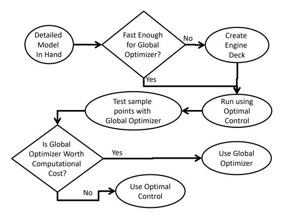
Figure 24: Procedure for Selecting Power Schedule Optimizer
