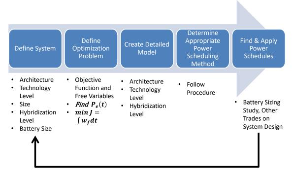
Figure 69: Systematic Hybrid Aircraft Power Schedule Optimizer (SHAPSO)
