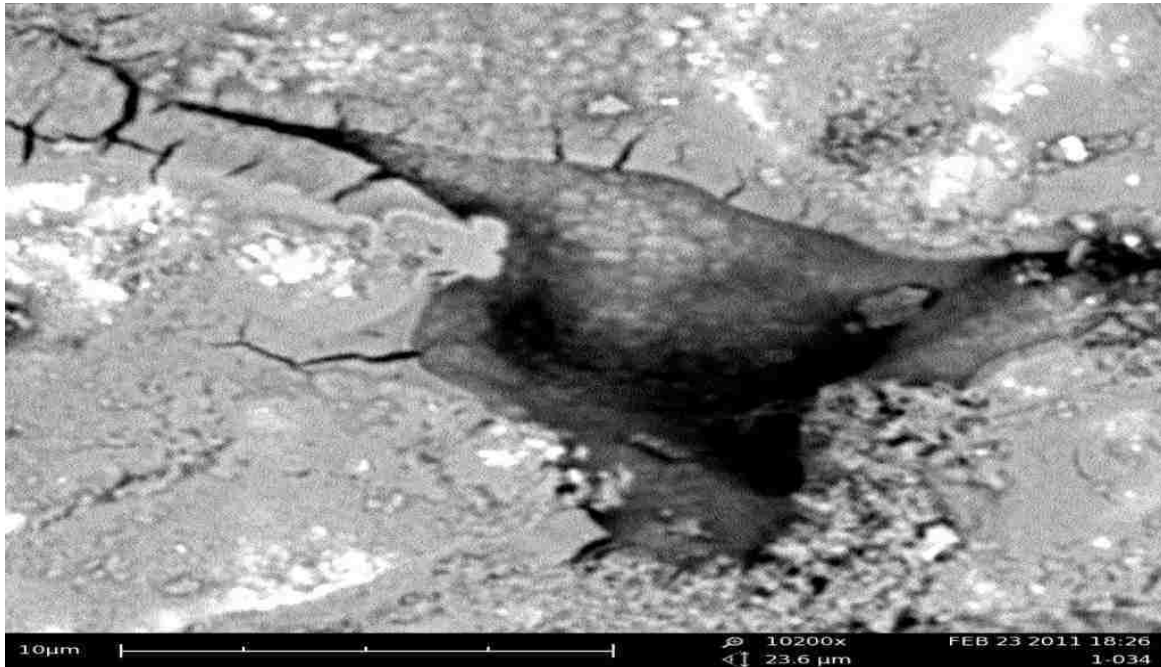
a.. Experiment 1-34 2 µm MOTT filter disc 10µm alumina particle Treated twice SnCl 2 / PdCl 2 seeded 3 times Figure 4.1.1.1.5: Close up of experiment 34 showing coral like formations with secondary fill on select edges.
