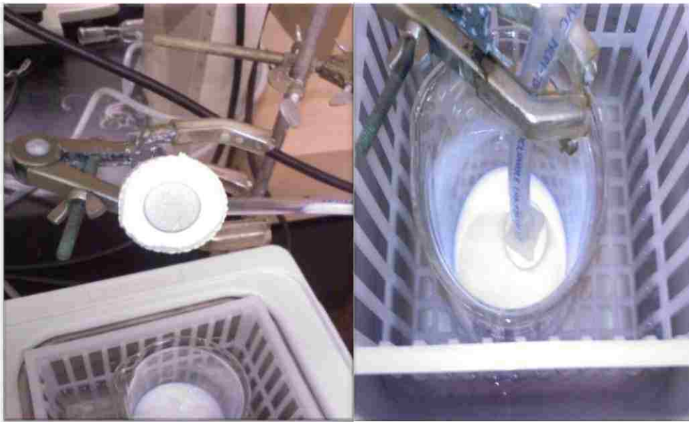
a. MOTT disc under suction on septa b. MOTT disc under suction in zirconia solution
