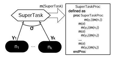
Figure 4.13. The CASL mapping of a complex task decomposition.
