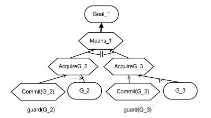
Figure 4.32. The fully detailed iASR diagram for the AND-decomposition of goals.
