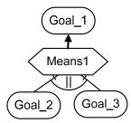
Figure 4.19b. Task decomposition with the concurrent composition annotation is used to model AND-decomposition of goals.
