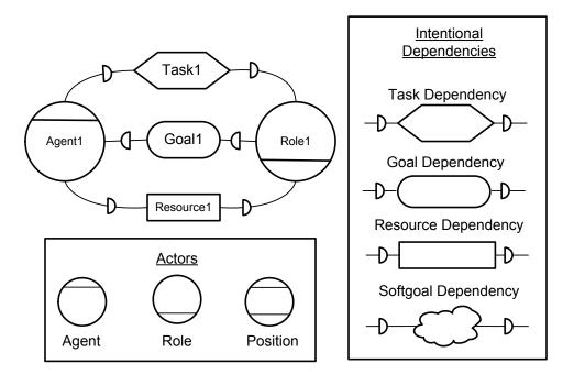
Figure 3.1. The SD diagram notation.
