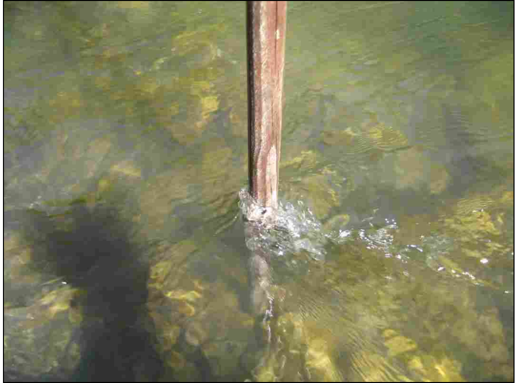
Figure 4-7: Critical Flow Wave Action on Wading Staff
