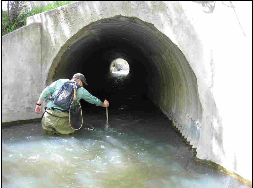
Figure 4-5: Correct Posture/Orientation for Determining Outlet Flow With a Wading Staff
