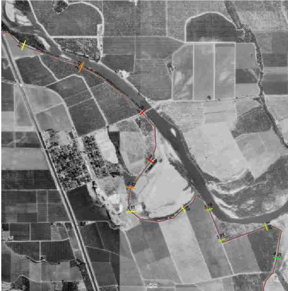
Figure 6-9 Cross sections displayed with graduated colors based on the factor of safety, labels also added for the factors of safety
