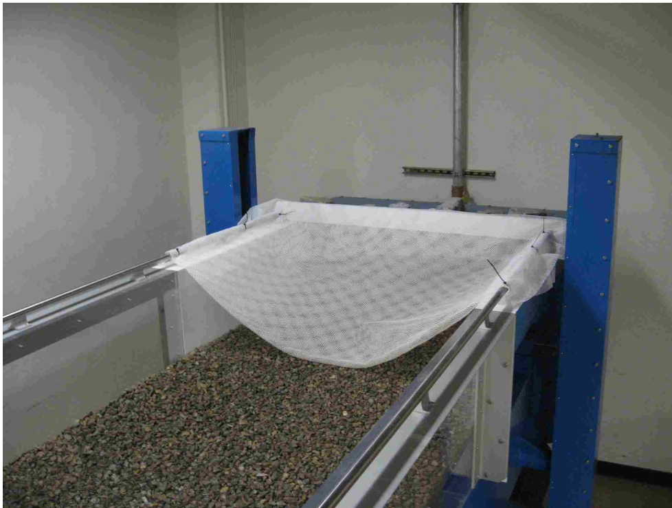
Figure B.2: Net placed at inlet of flume to prevent surface waves
