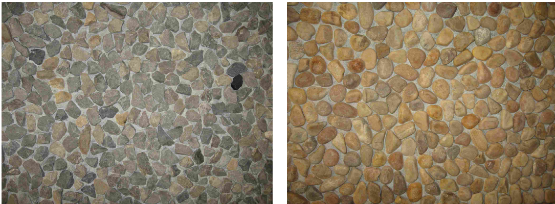
Figure B.7: Finished surface of angular and rounded gravel panels
