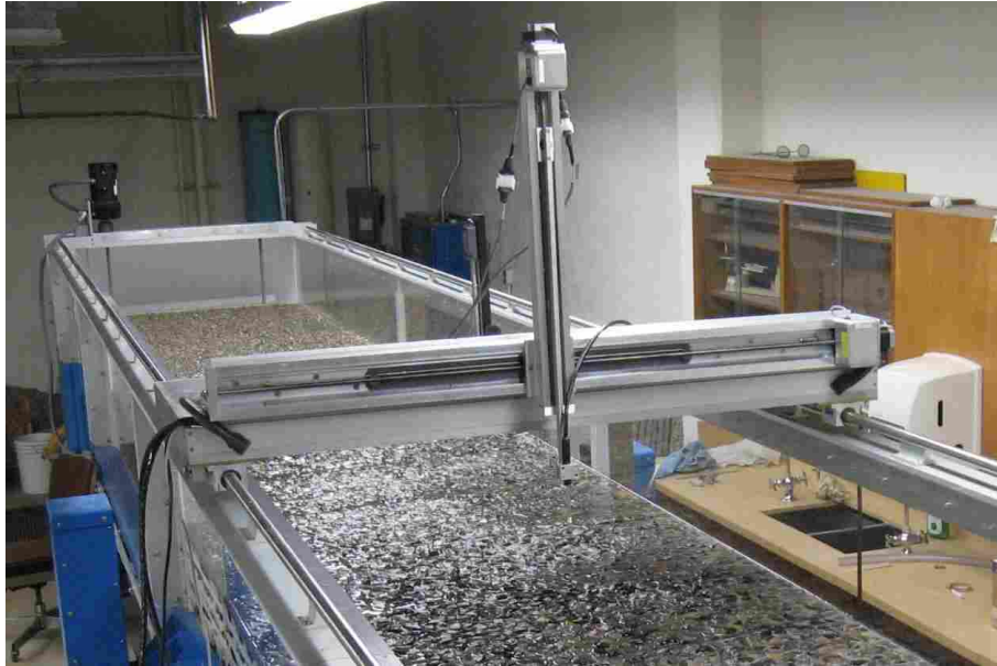
Figure 2.4: Trolley containing the ADV
