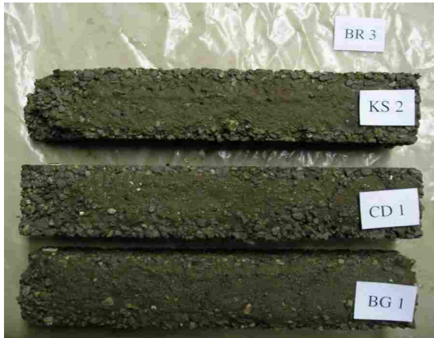
Figure E.7 Clogged, saturated specimens after 28-day cure and 141 freeze-thaw cycles.
