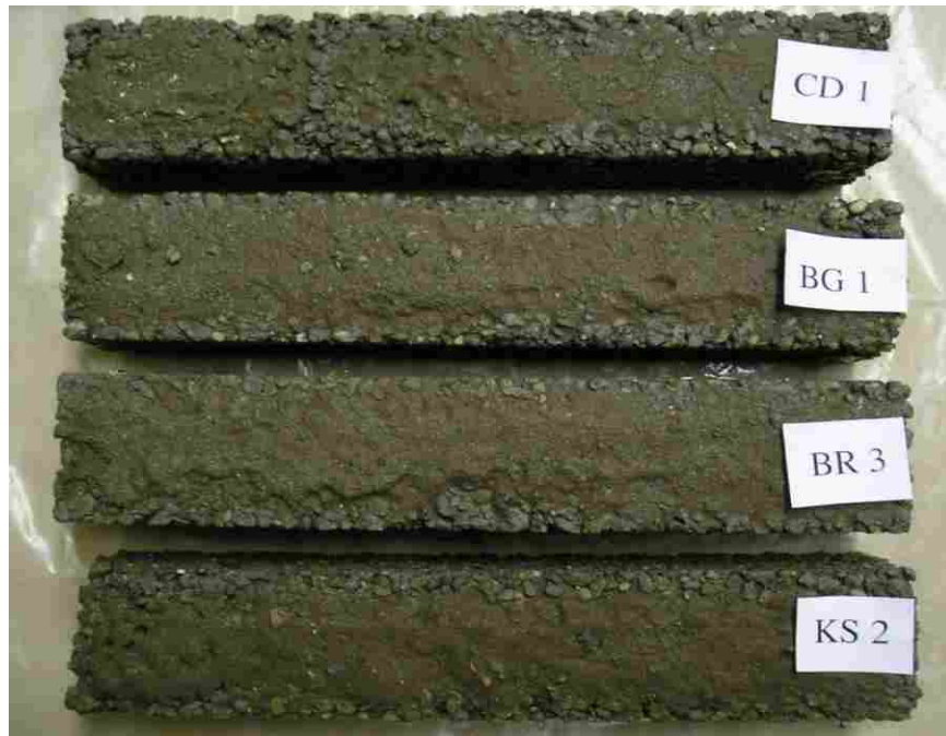
Figure E.5 Clogged, saturated specimens after 28-day cure and 101 freeze-thaw cycles.
