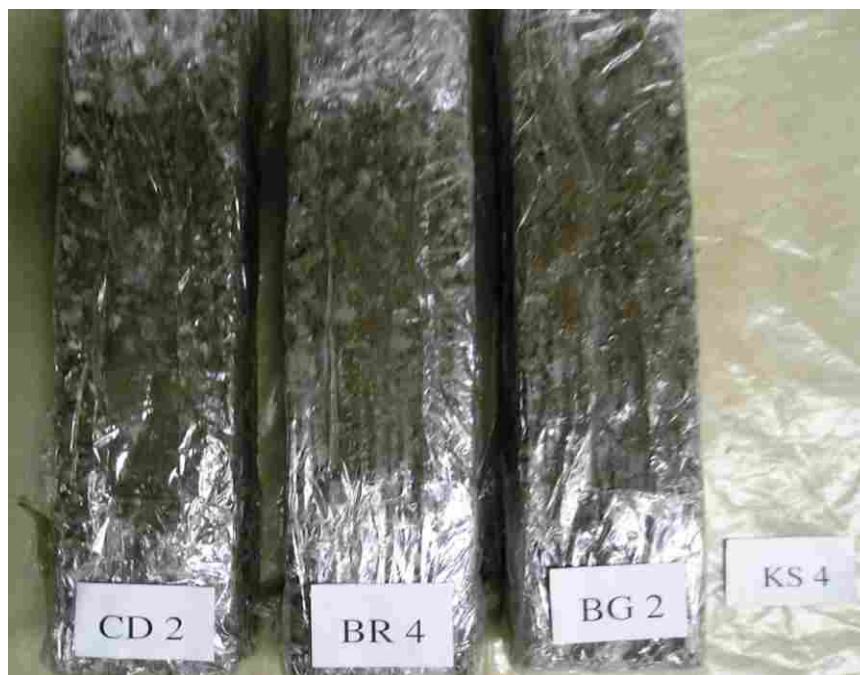
Figure F.10 Unsaturated, clogged specimens after 28-day cure and 200 freeze-thaw cycles.
