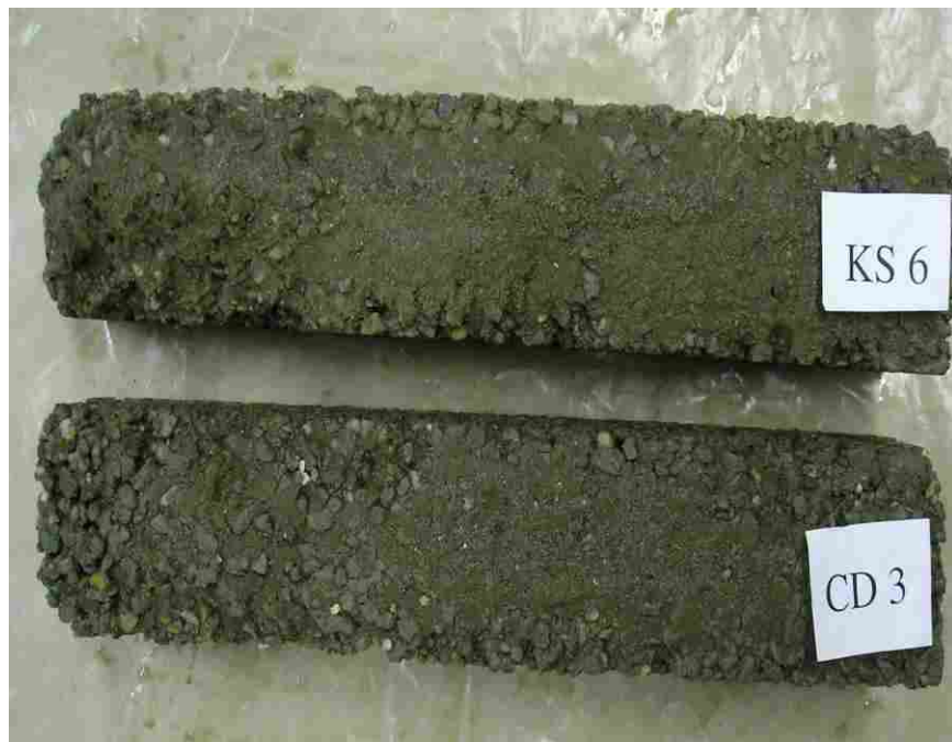
Figure I.10 Clogged, saturated specimens after 90-day cure and 200 freeze-thaw cycles.
