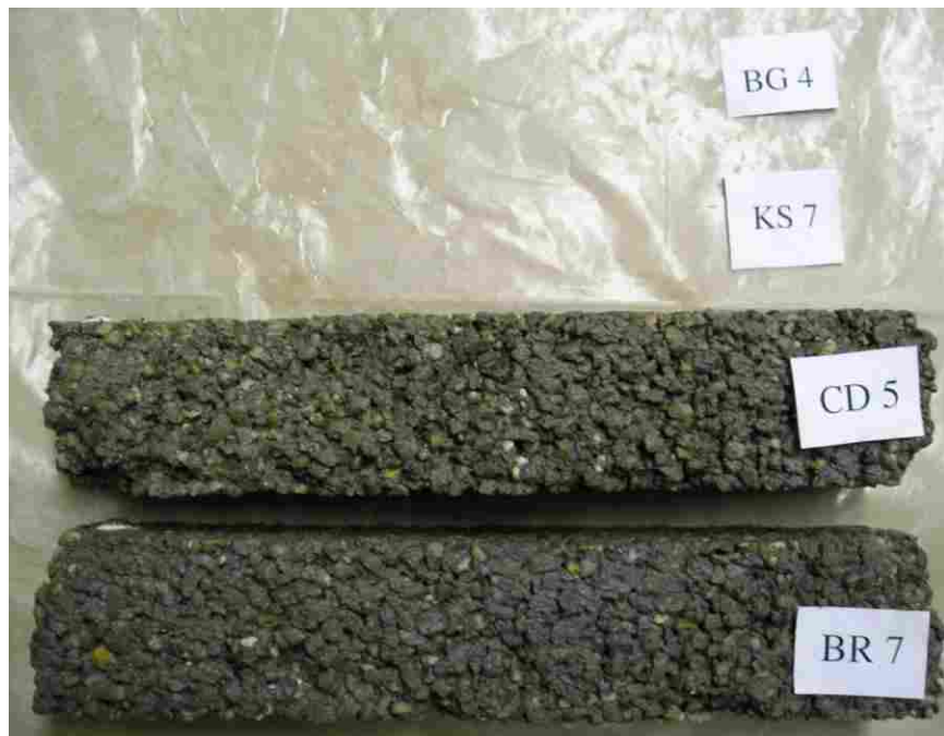
Figure G.10 Unclogged, saturated specimens after 28-day cure and 200 freeze-thaw cycles.
