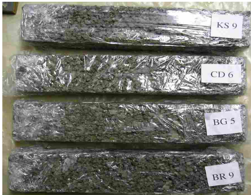
Figure H.8 Unclogged, unsaturated specimens after 28-day cure and 161 freeze-thaw cycles.
