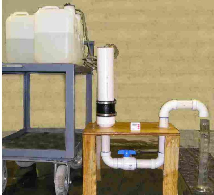
FIGURE 3.5 Laboratory permeability testing setup.
