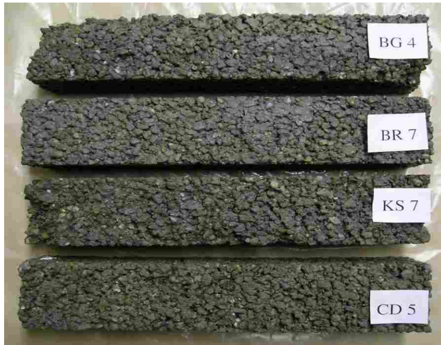
Figure G.5 Unclogged, saturated specimens after 28-day cure and 101 freeze-thaw cycles.
