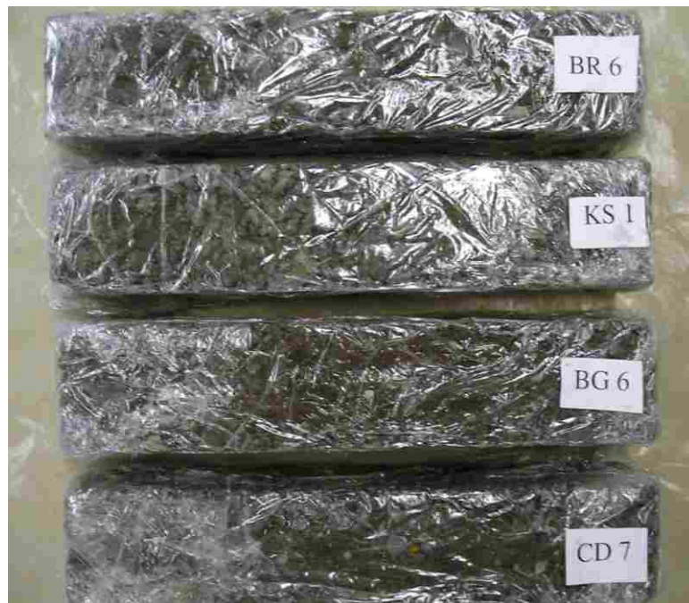
Figure J.10 Clogged, unsaturated specimens after 90-day cure and 200 freeze-thaw cycles.
