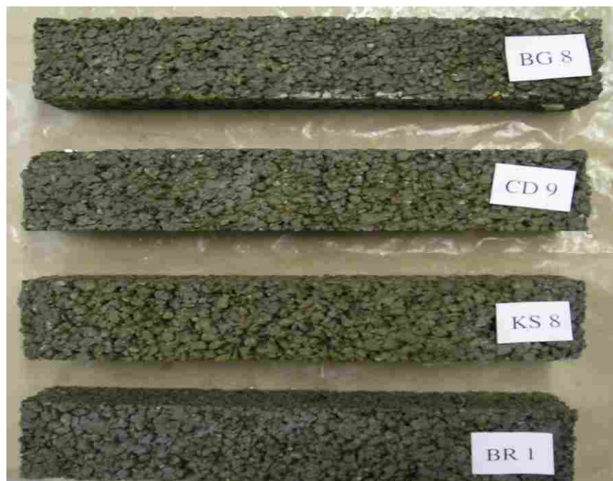
Figure K.2 Unclogged, saturated specimens after 90-day cure and 40 freeze-thaw cycles.
