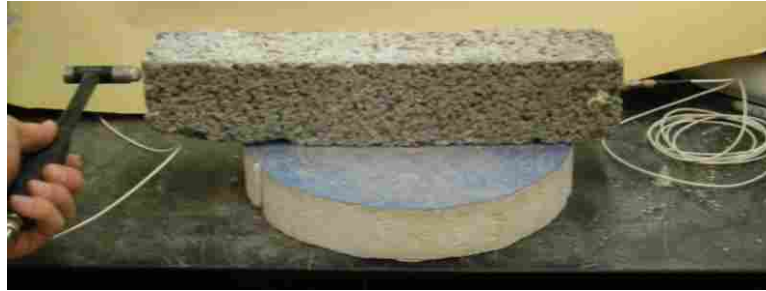
FIGURE 2.3 Longitudinal frequency testing setup.
