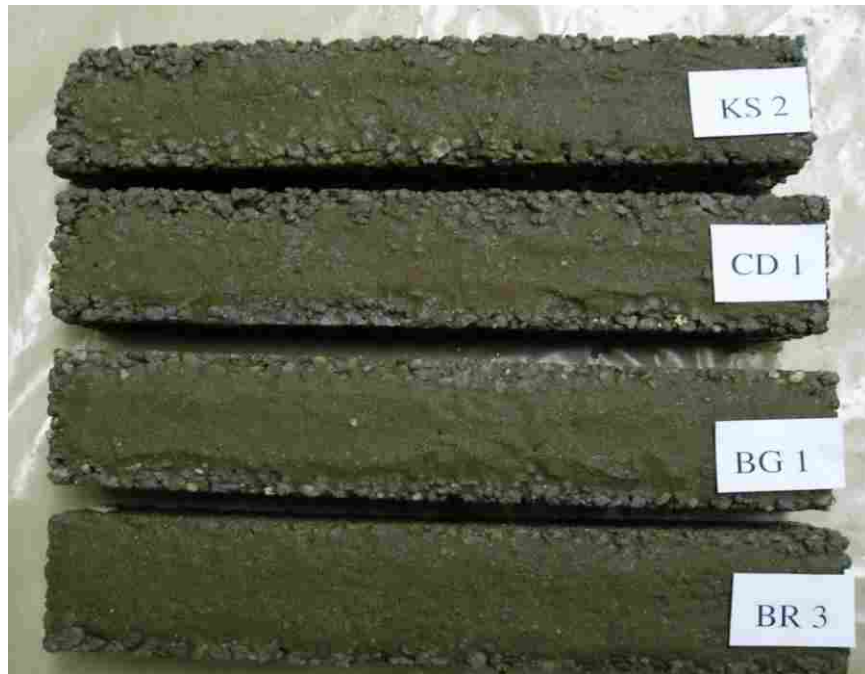
Figure E.3 Clogged, saturated specimens after 28-day cure and 60 freeze-thaw cycles.
