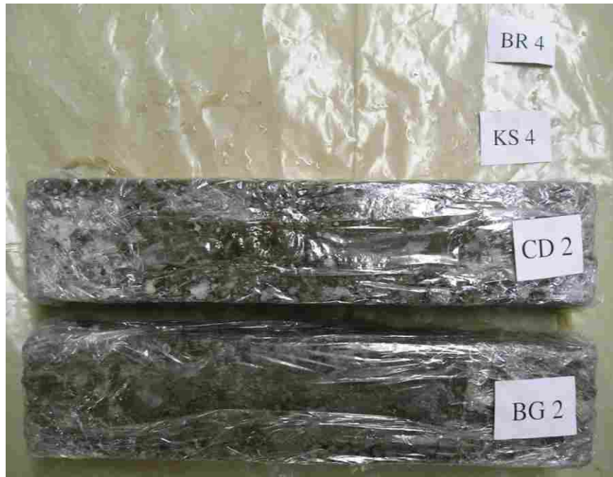
Figure F.13 Unsaturated, clogged specimens after 28-day cure and 260 freeze-thaw cycles.
