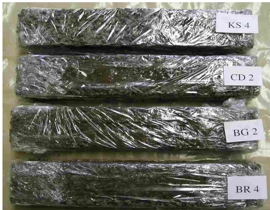
Figure F.2 Unsaturated, clogged specimens after 28-day cure and 40 freeze-thaw cycles.
