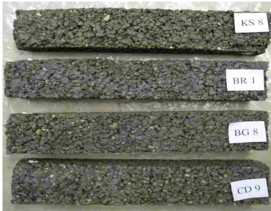
Figure K.5 Unclogged, saturated specimens after 90-day cure and 100 freeze-thaw cycles.
