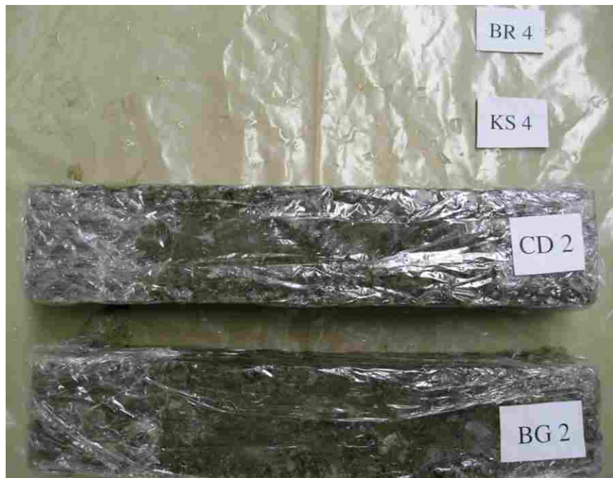
Figure F.12 Unsaturated, clogged specimens after 28-day cure and 240 freeze-thaw cycles.
