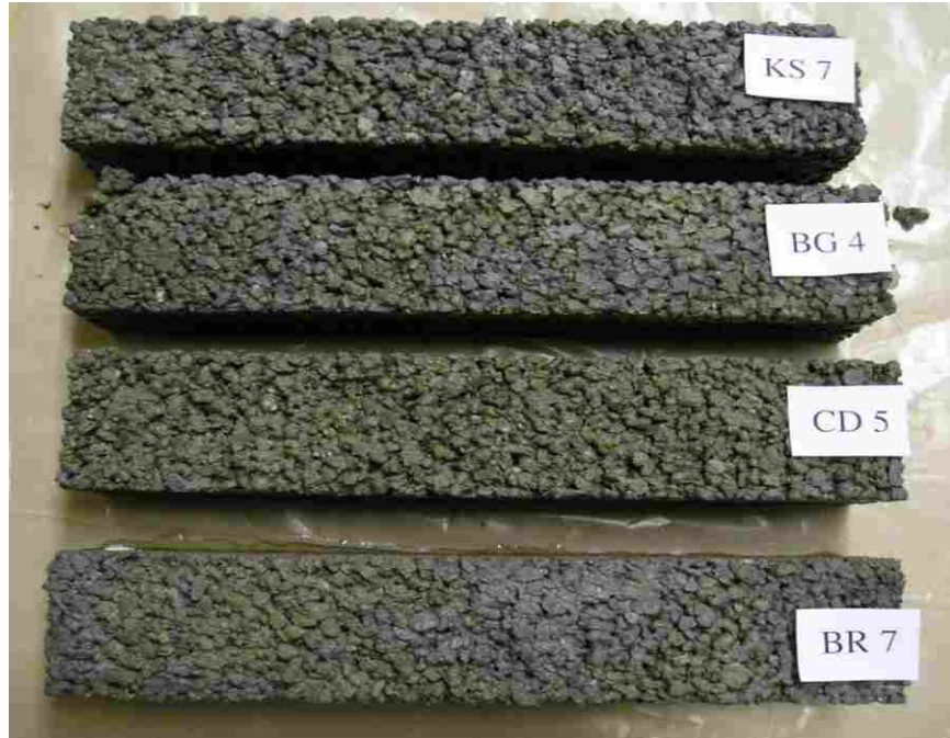
Figure G.1 Unclogged, saturated specimens after 28-day cure and 20 freeze-thaw cycles.
