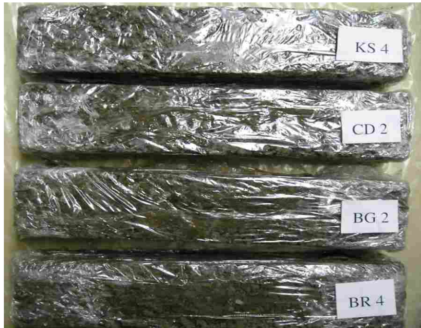
Figure F.7 Unsaturated, clogged specimens after 28-day cure and 141 freeze-thaw cycles.
