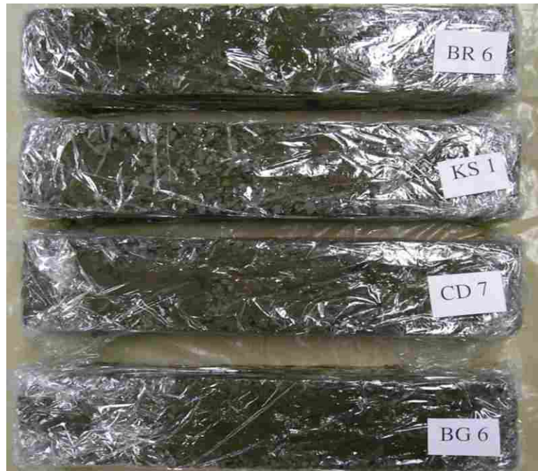
Figure J.1 Clogged, unsaturated specimens after 90-day cure and 20 freeze-thaw cycles.
