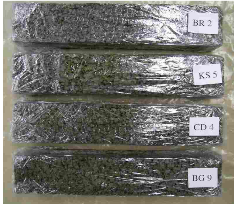
Figure L.1 Unclogged, unsaturated specimens after 90-day cure and 20 freeze-thaw cycles.
