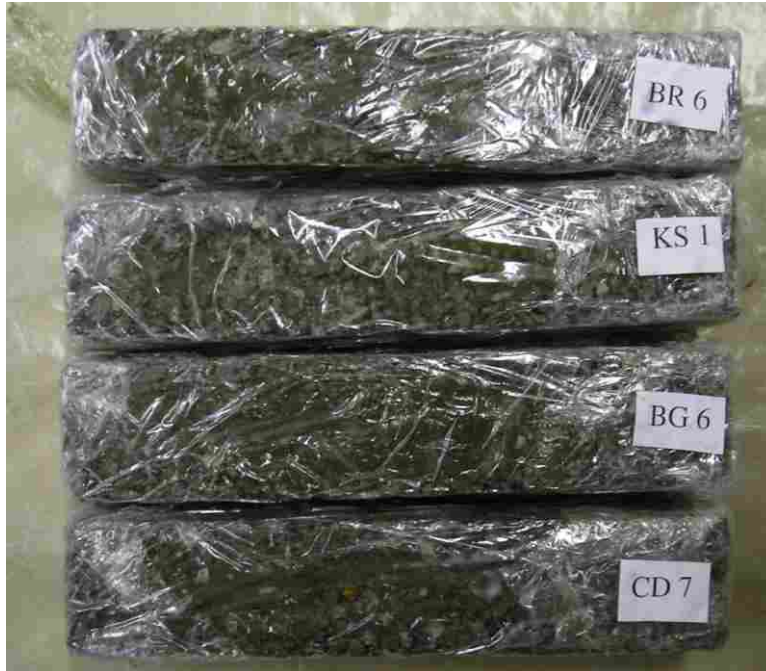
Figure J.11 Clogged, unsaturated specimens after 90-day cure and 220 freeze-thaw cycles.
