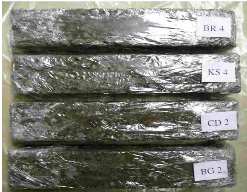
Figure F.6 Unsaturated, clogged specimens after 28-day cure and 121 freeze-thaw cycles.
