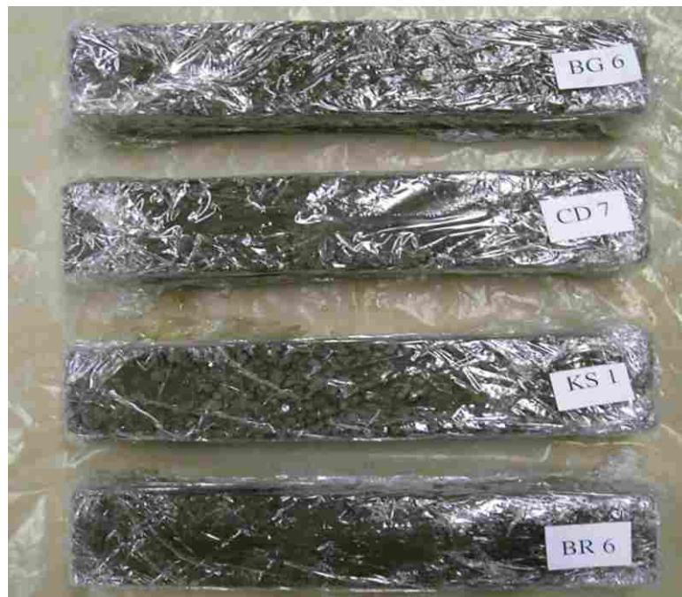
Figure J.2 Clogged, unsaturated specimens after 90-day cure and 40 freeze-thaw cycles.
