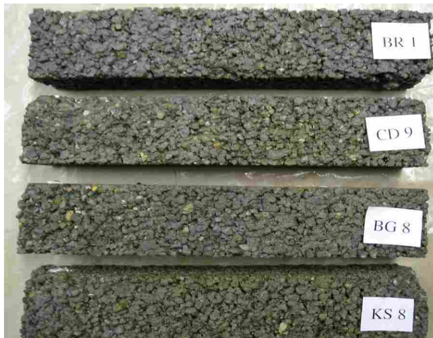
Figure K.4 Unclogged, saturated specimens after 90-day cure and 80 freeze-thaw cycles.
