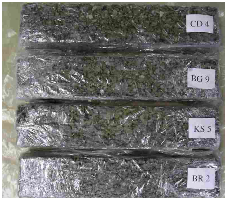
Figure L.12 Unclogged, unsaturated specimens after 90-day cure and 240 freeze-thaw cycles.
