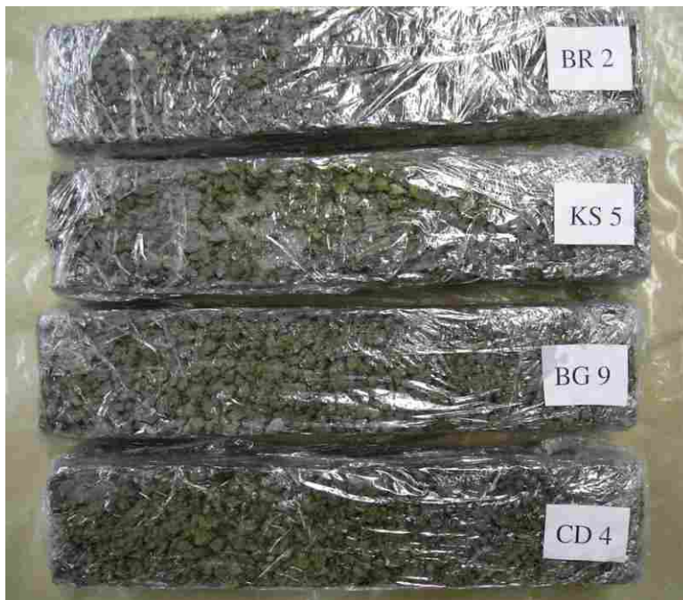
Figure L.8 Unclogged, unsaturated specimens after 90-day cure and 160 freeze-thaw cycles.
