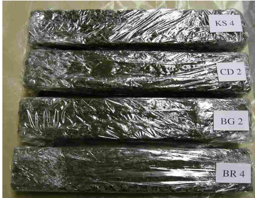
Figure F.1 Unsaturated, clogged specimens after 28-day cure and 20 freeze-thaw cycles.
