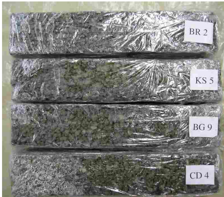
Figure L.11 Unclogged, unsaturated specimens after 90-day cure and 220 freeze-thaw cycles.
