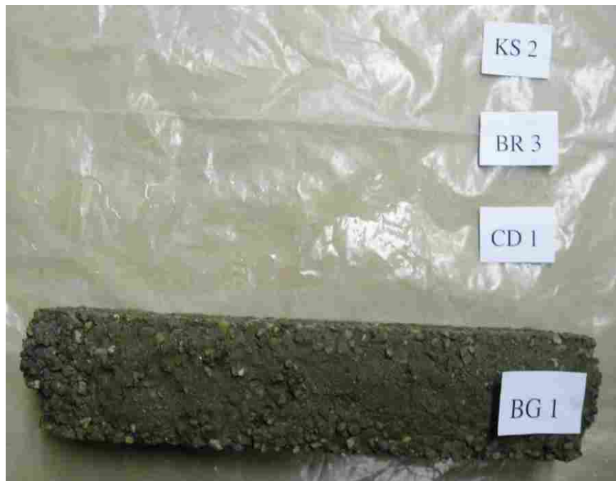
Figure E.8 Clogged, saturated specimens after 28-day cure and 161 freeze-thaw cycles.
