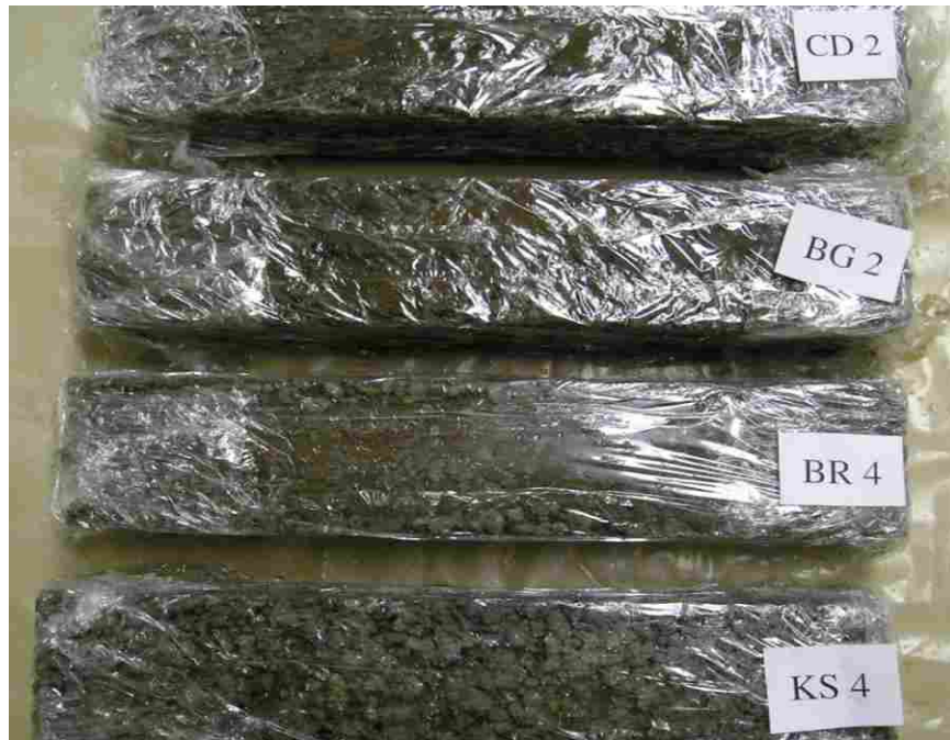
Figure F.3 Unsaturated, clogged specimens after 28-day cure and 60 freeze-thaw cycles.
