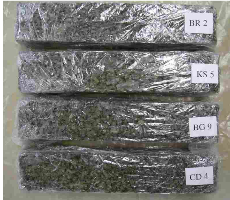
Figure L.9 Unclogged, unsaturated specimens after 90-day cure and 180 freeze-thaw cycles.
