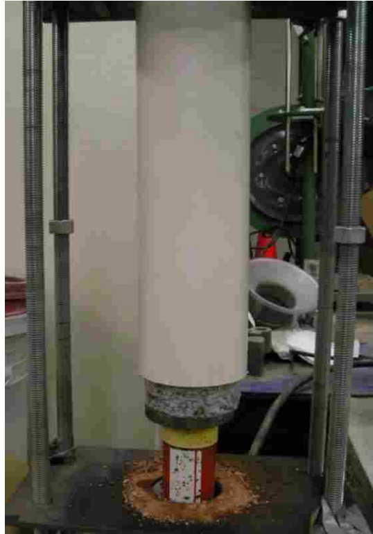
FIGURE 3.8 Use of hydraulic ram to seat laboratory permeability test specimen into pipe.
