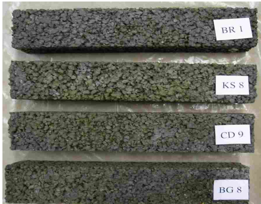
Figure K.1 Unclogged, saturated specimens after 90-day cure and 20 freeze-thaw cycles.
