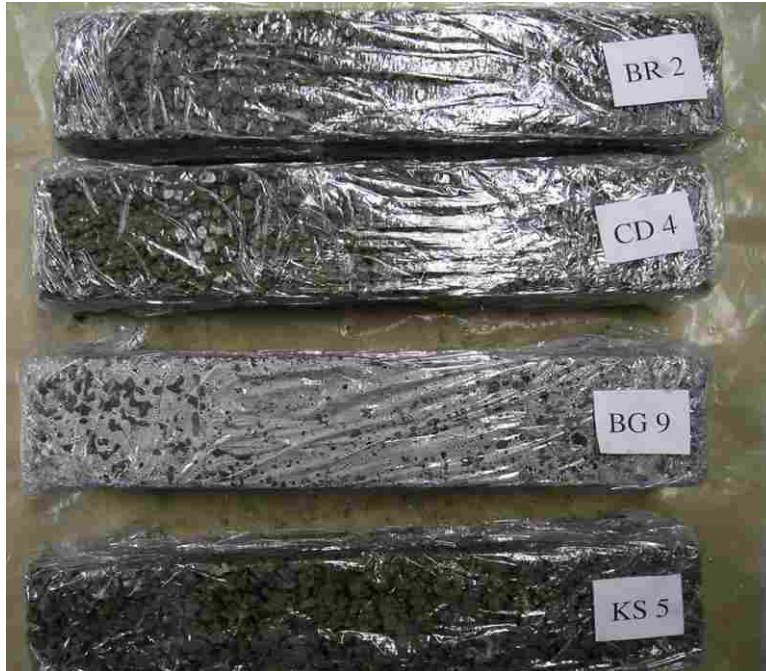
Figure L.3 Unclogged, unsaturated specimens after 90-day cure and 60 freeze-thaw cycles.
