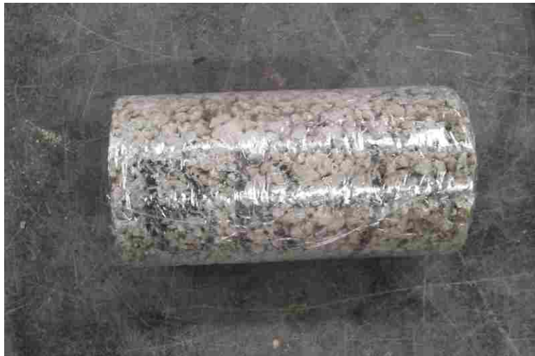
FIGURE 3.6 Use of plastic wrap to seal sides of laboratory permeability test specimen.
