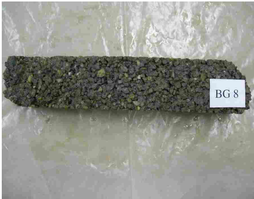
Figure K.9 Unclogged, saturated specimens after 90-day cure and 180 freeze-thaw cycles.
