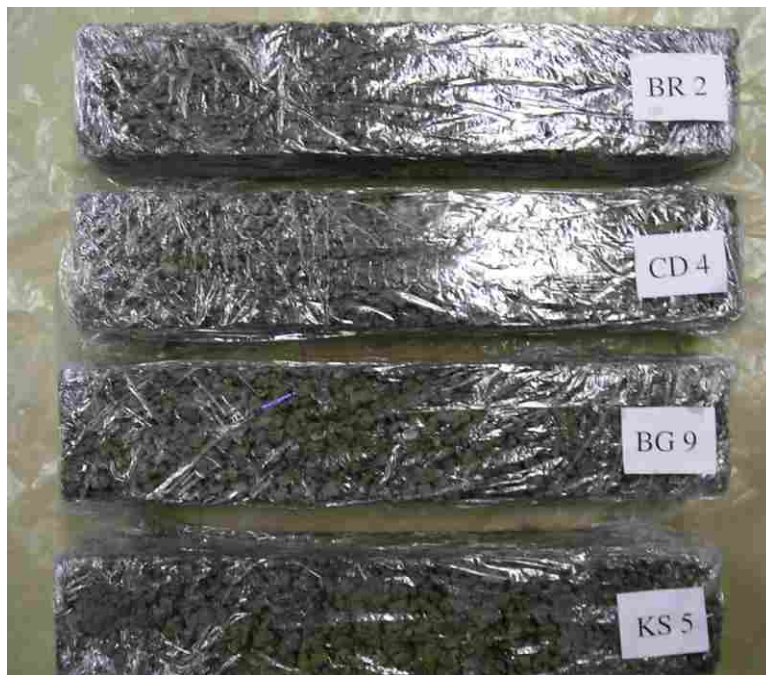
Figure L.4 Unclogged, unsaturated specimens after 90-day cure and 80 freeze-thaw cycles.
