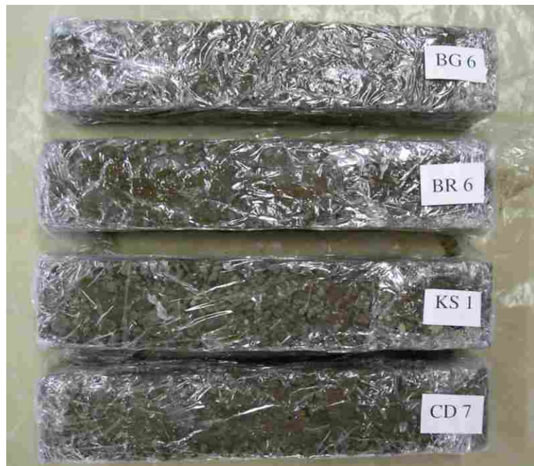
Figure J.6 Clogged, unsaturated specimens after 90-day cure and 120 freeze-thaw cycles.
