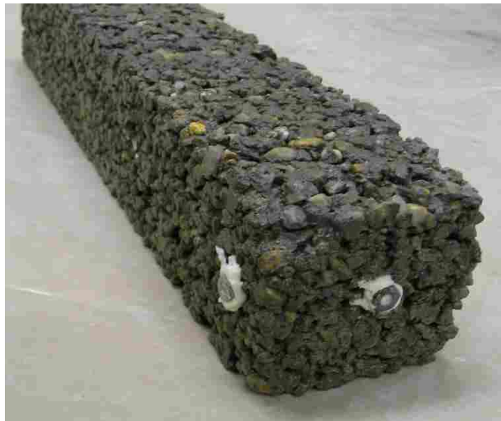
FIGURE 3.3 Steel nut configurations on laboratory beam specimen.
