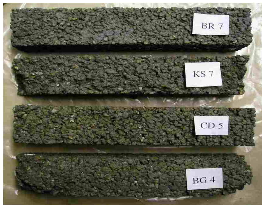
Figure G.6 Unclogged, saturated specimens after 28-day cure and 121 freeze-thaw cycles.
