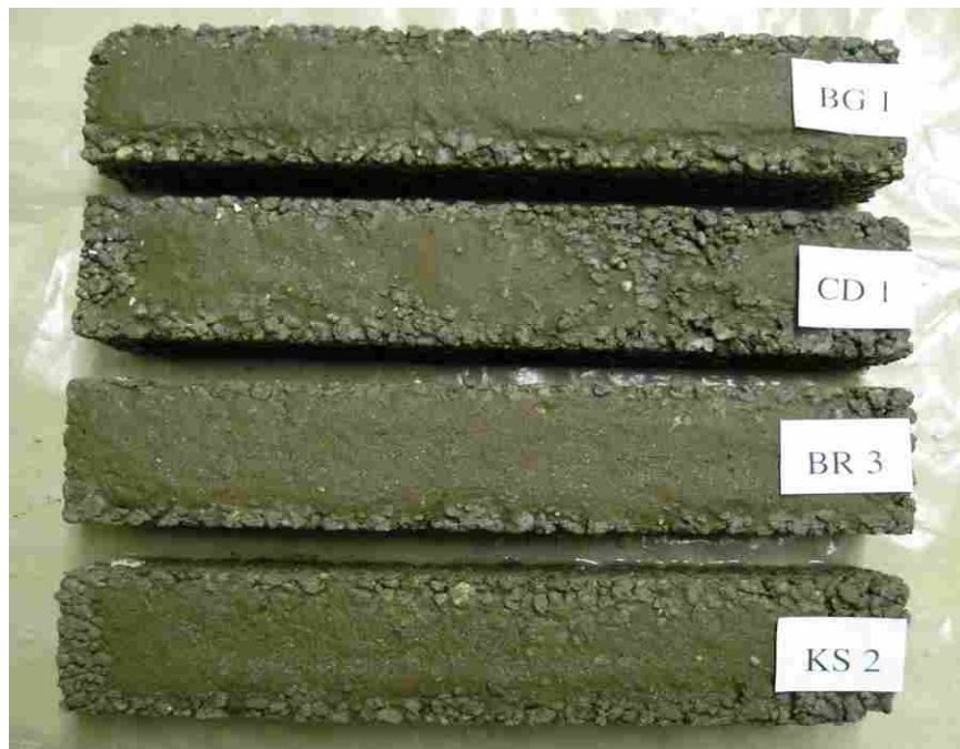
Figure E.4 Clogged, saturated specimens after 28-day cure and 81 freeze-thaw cycles.
