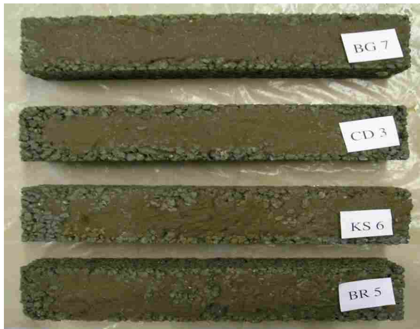
Figure I.2 Clogged, saturated specimens after 90-day cure and 40 freeze-thaw cycles.
