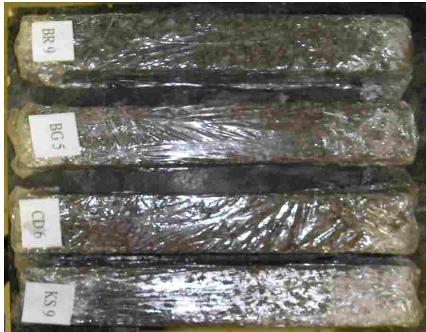
Figure H.14 Unclogged, unsaturated specimens after 28-day cure and 280 freeze-thaw cycles.
