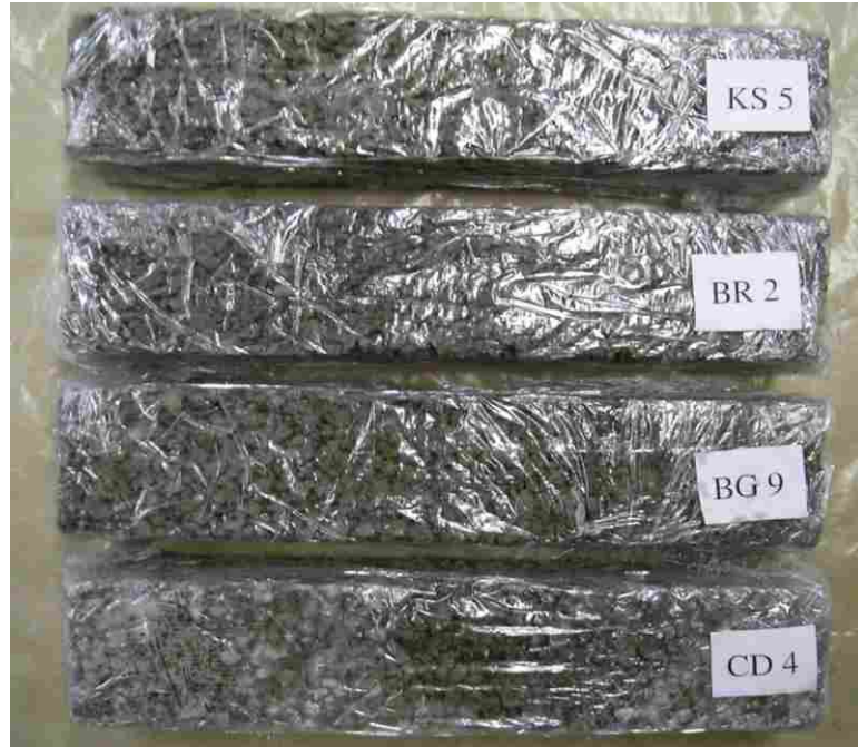
Figure L.5 Unclogged, unsaturated specimens after 90-day cure and 100 freeze-thaw cycles.
