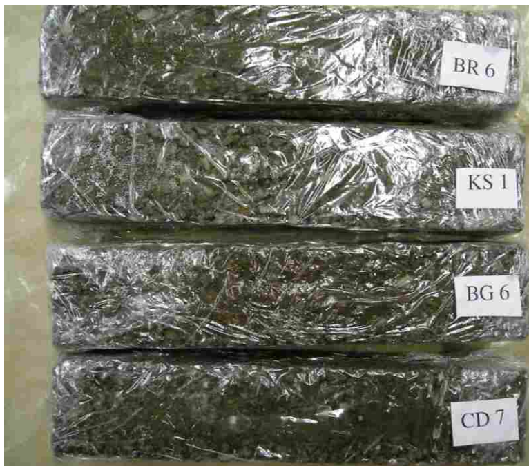
Figure J.8 Clogged, unsaturated specimens after 90-day cure and 160 freeze-thaw cycles.
