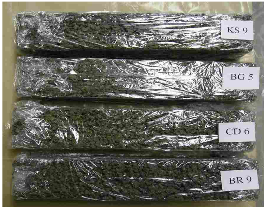
Figure H.1 Unclogged, unsaturated specimens after 28-day cure and 20 freeze-thaw cycles.
