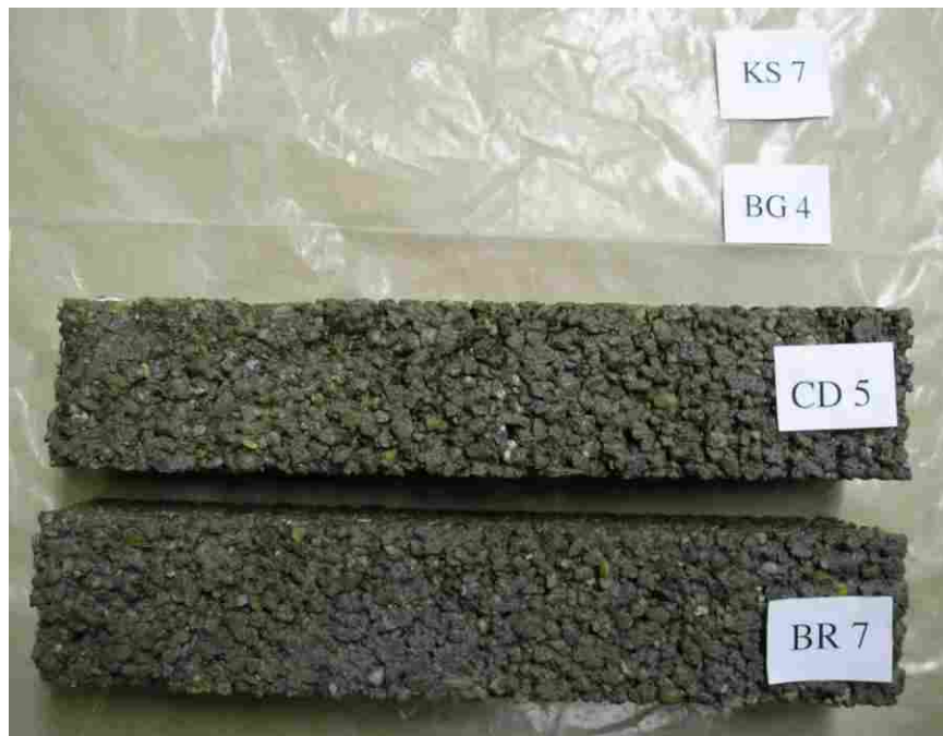
Figure G.8 Unclogged, saturated specimens after 28-day cure and 161 freeze-thaw cycles.
