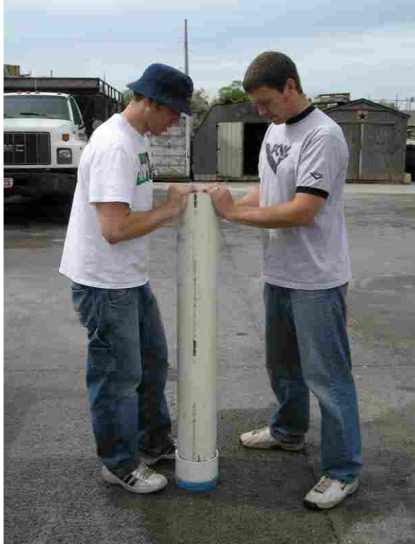
FIGURE 3.12 Field permeability testing setup.
