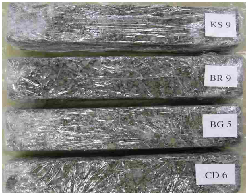
Figure H.15 Unclogged, unsaturated specimens after 28-day cure and 300 freeze-thaw cycles.
