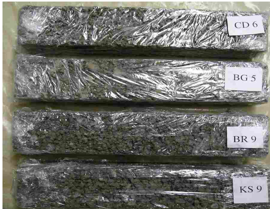
Figure H.10 Unclogged, unsaturated specimens after 28-day cure and 200 freeze-thaw cycles.
