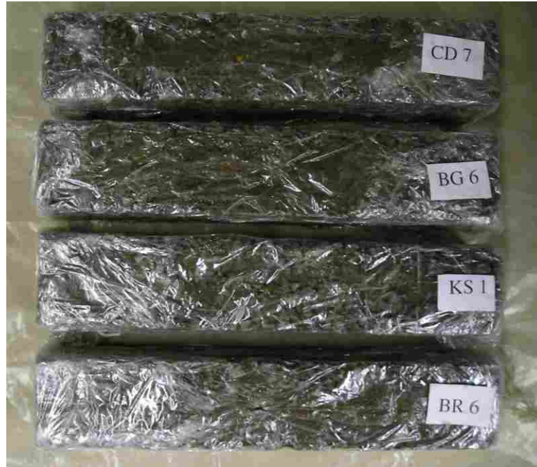
Figure J.13 Clogged, unsaturated specimens after 90-day cure and 260 freeze-thaw cycles.
