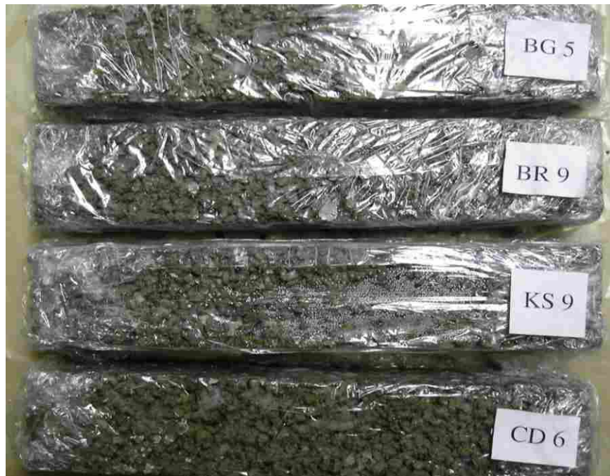
Figure H.6 Unclogged, unsaturated specimens after 28-day cure and 121 freeze-thaw cycles.
