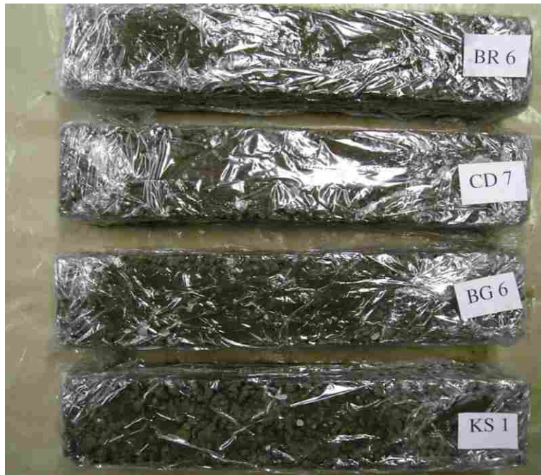
Figure J.3 Clogged, unsaturated specimens after 90-day cure and 60 freeze-thaw cycles.
