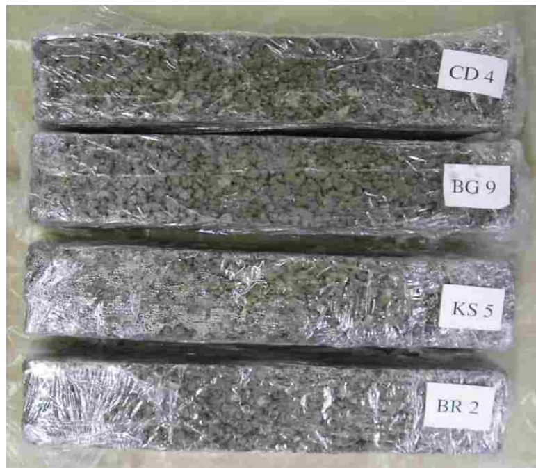
Figure L.14 Unclogged, unsaturated specimens after 90-day cure and 281 freeze-thaw cycles.
