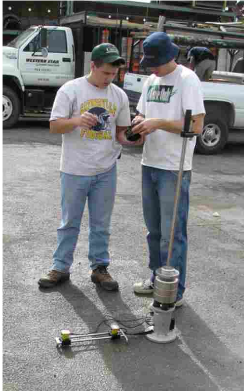
FIGURE 3.11 Field stiffness testing setup.
