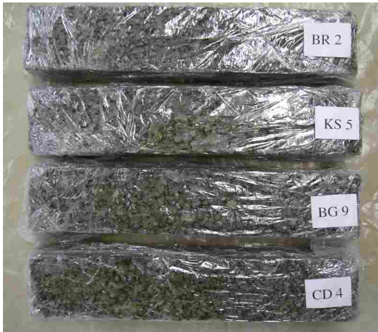
Figure L.15 Unclogged, unsaturated specimens after 90-day cure and 306 freeze-thaw cycles.
