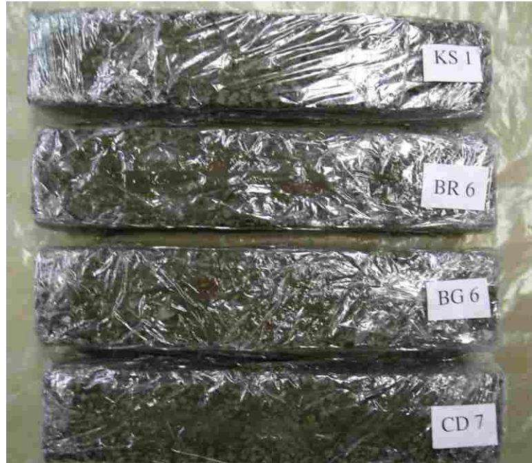
Figure J.5 Clogged, unsaturated specimens after 90-day cure and 100 freeze-thaw cycles.
