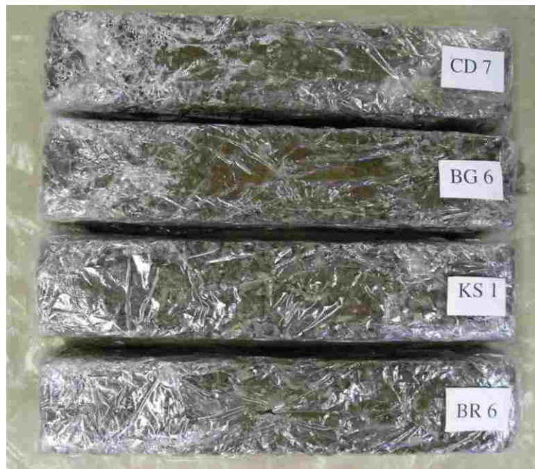
Figure J.14 Clogged, unsaturated specimens after 90-day cure and 281 freeze-thaw cycles.
