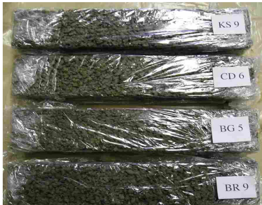
Figure H.2 Unclogged, unsaturated specimens after 28-day cure and 40 freeze-thaw cycles.
