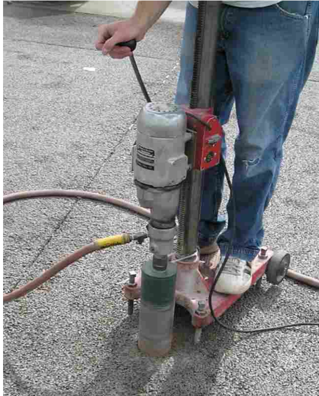
FIGURE 3.13 Field coring setup.
