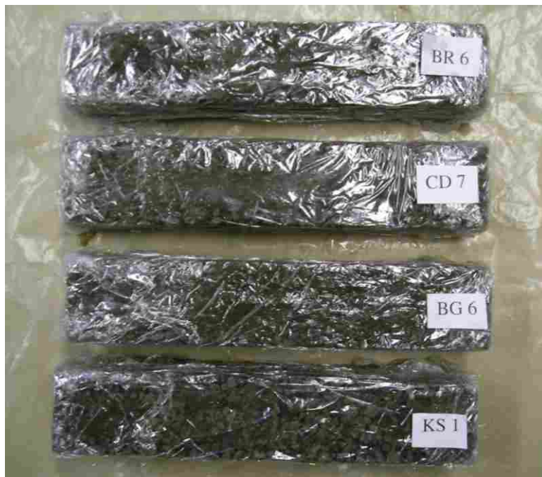
Figure J.4 Clogged, unsaturated specimens after 90-day cure and 80 freeze-thaw cycles.
