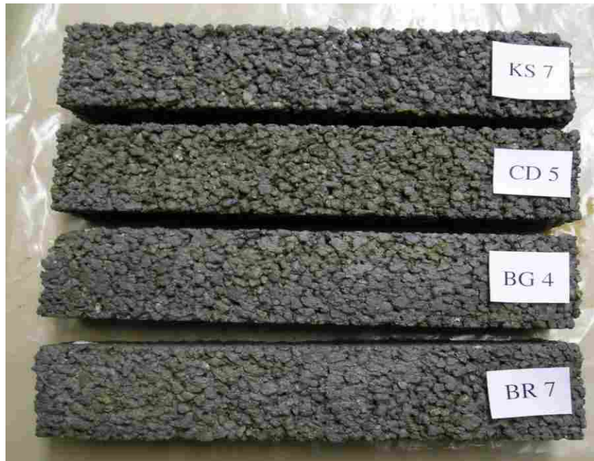
Figure G.2 Unclogged, saturated specimens after 28-day cure and 40 freeze-thaw cycles.
