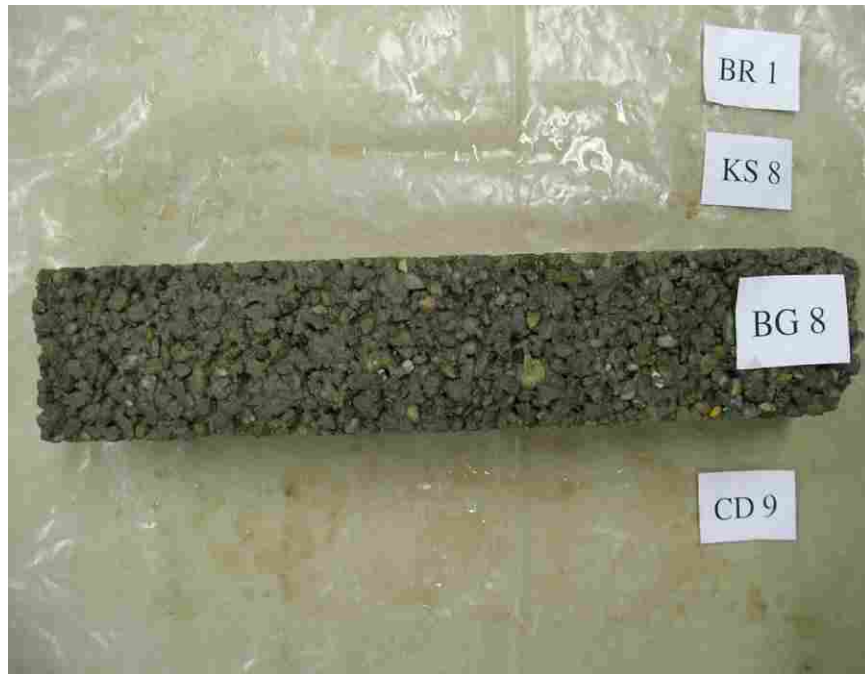
Figure K.7 Unclogged, saturated specimens after 90-day cure and 140 freeze-thaw cycles.
