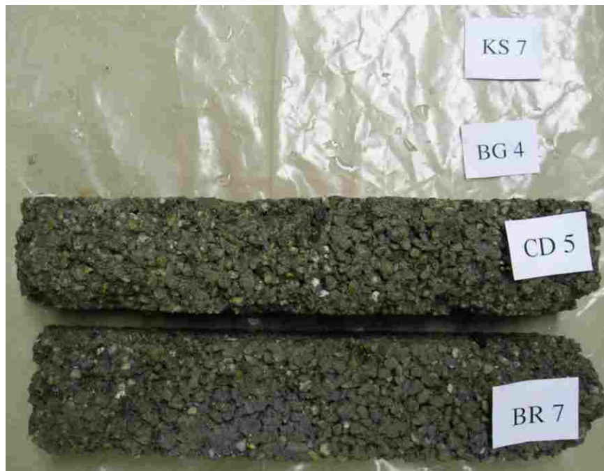
Figure G.12 Unclogged, saturated specimens after 28-day cure and 240 freeze-thaw cycles.
