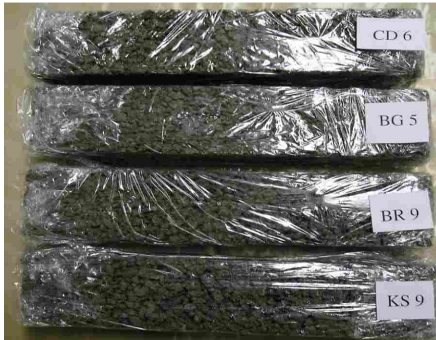
Figure H.3 Unclogged, unsaturated specimens after 28-day cure and 60 freeze-thaw cycles.
