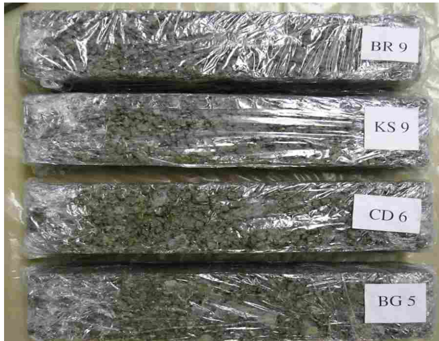
Figure H.12 Unclogged, unsaturated specimens after 28-day cure and 240 freeze-thaw cycles.
