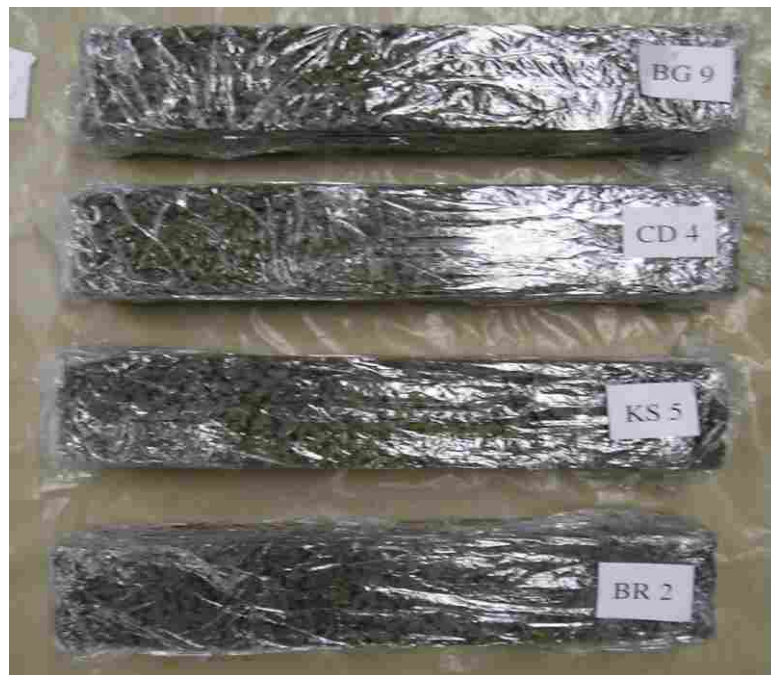
Figure L.2 Unclogged, unsaturated specimens after 90-day cure and 40 freeze-thaw cycles.
