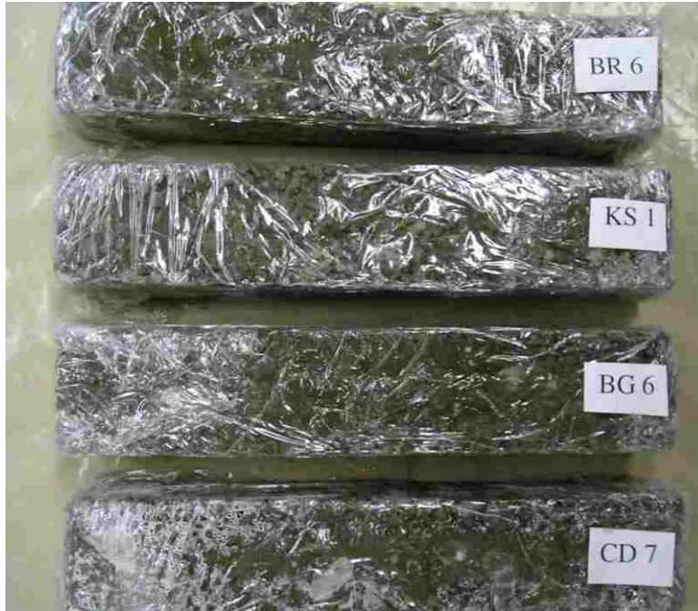
Figure J.7 Clogged, unsaturated specimens after 90-day cure and 140 freeze-thaw cycles.
