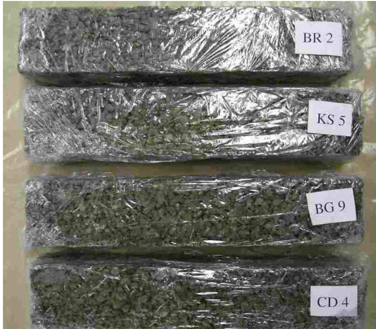
Figure L.7 Unclogged, unsaturated specimens after 90-day cure and 140 freeze-thaw cycles.
