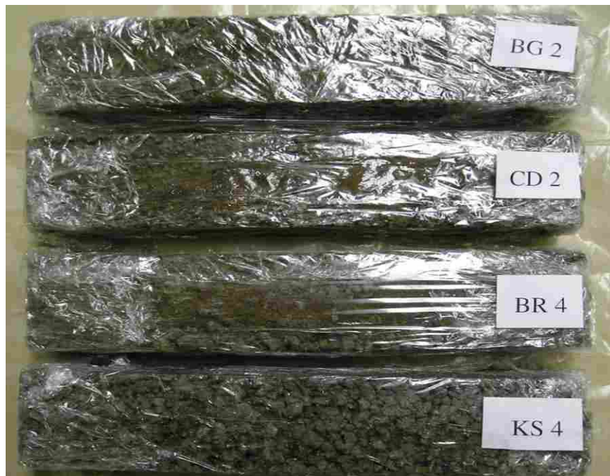
Figure F.4 Unsaturated, clogged specimens after 28-day cure and 81 freeze-thaw cycles.
