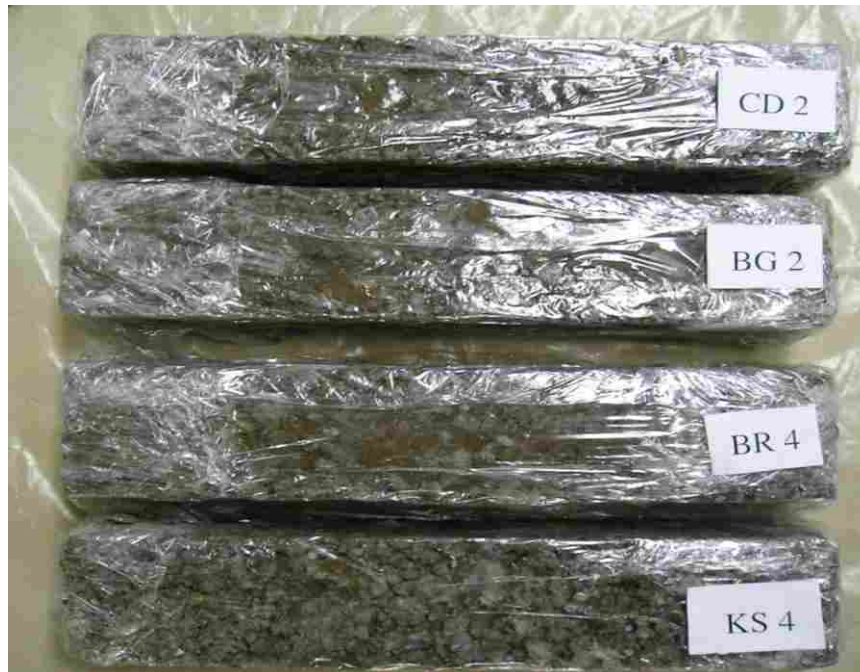
Figure F.9 Unsaturated, clogged specimens after 28-day cure and 186 freeze-thaw cycles.
