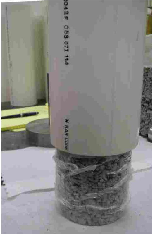
FIGURE 3.7 Use of silicone for sliding laboratory permeability test specimen into pipe.
