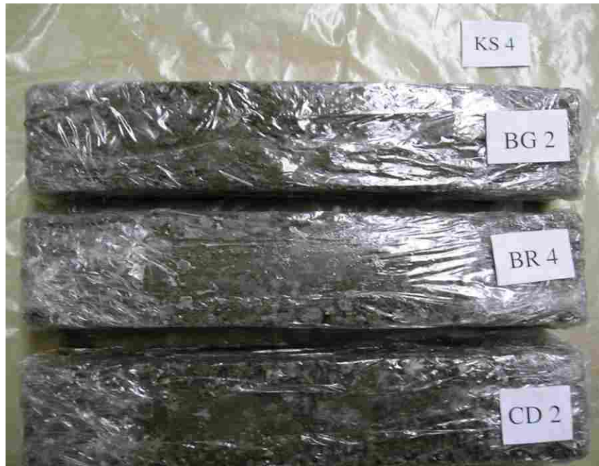
Figure F.11 Unsaturated, clogged specimens after 28-day cure and 220 freeze-thaw cycles.
