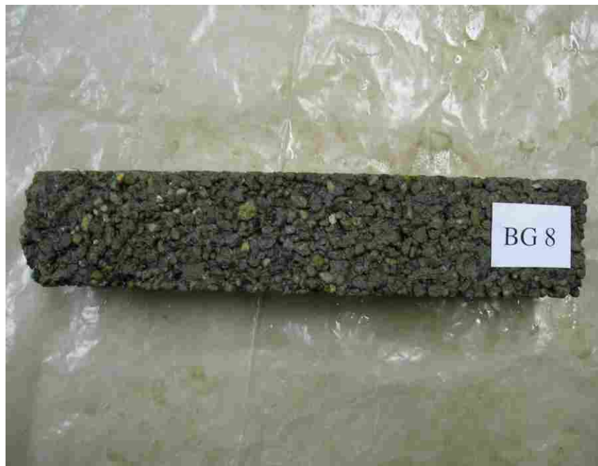
Figure K.8 Unclogged, saturated specimens after 90-day cure and 160 freeze-thaw cycles.
