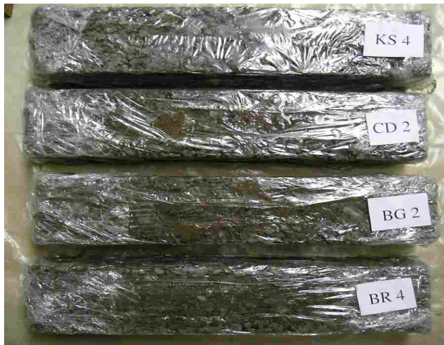
Figure F.8 Unsaturated, clogged specimens after 28-day cure and 161 freeze-thaw cycles.
