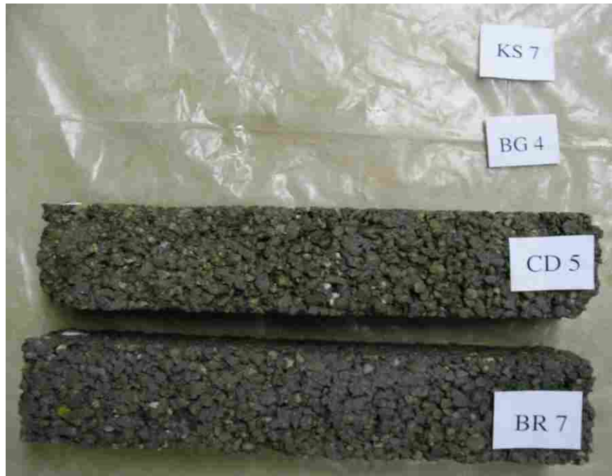
Figure G.9 Unclogged, saturated specimens after 28-day cure and 186 freeze-thaw cycles.
