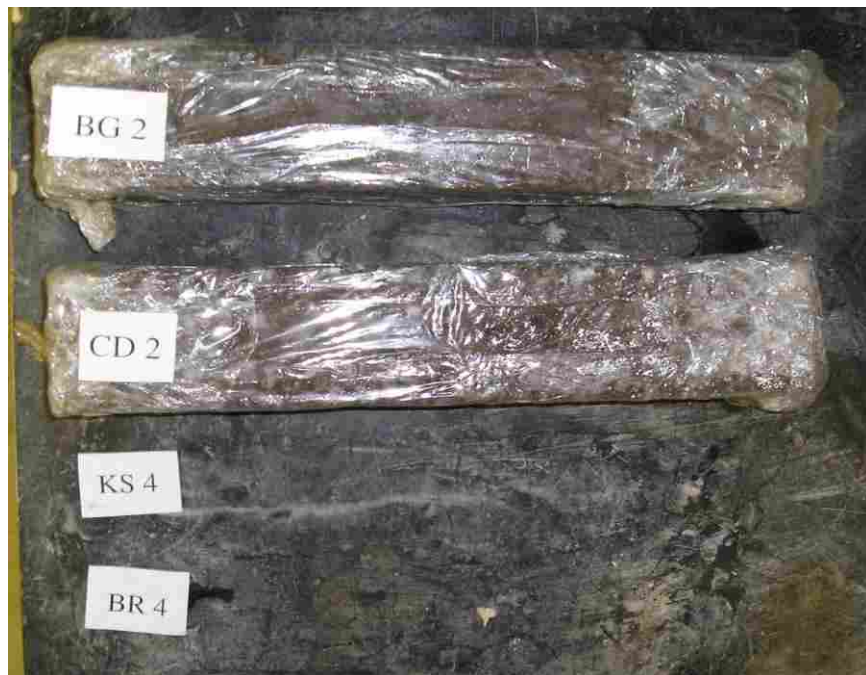
Figure F.14 Unsaturated, clogged specimens after 28-day cure and 280 freeze-thaw cycles.
