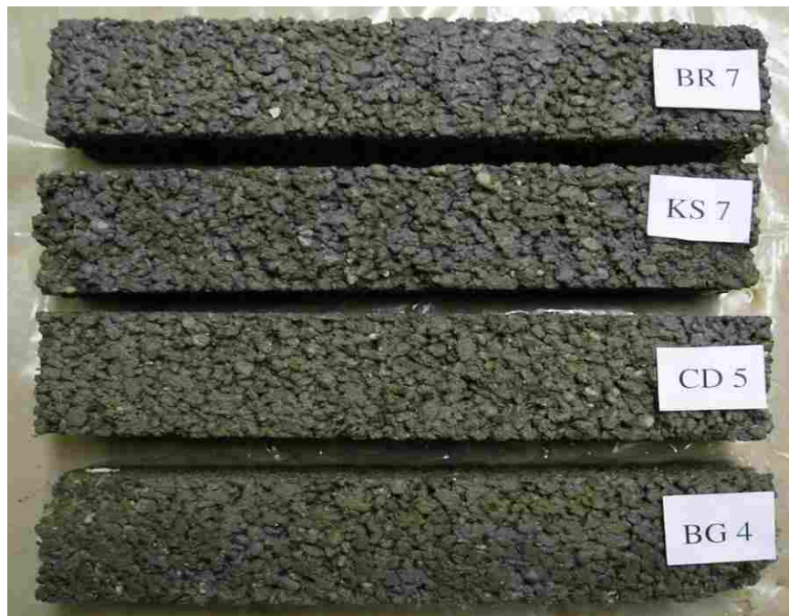
Figure G.4 Unclogged, saturated specimens after 28-day cure and 81 freeze-thaw cycles.
