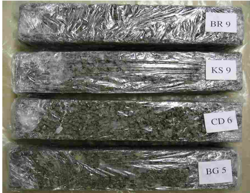
Figure H.13 Unclogged, unsaturated specimens after 28-day cure and 260 freeze-thaw cycles.
