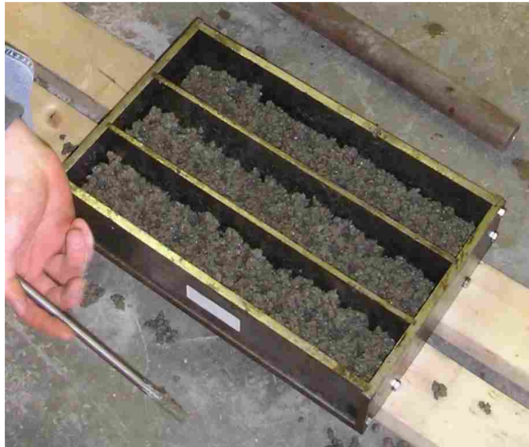
FIGURE 3.2 Mold for preparing laboratory beam specimens.
