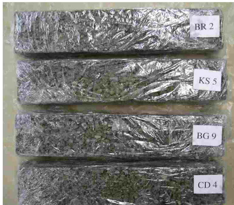
Figure L.10 Unclogged, unsaturated specimens after 90-day cure and 200 freeze-thaw cycles.
