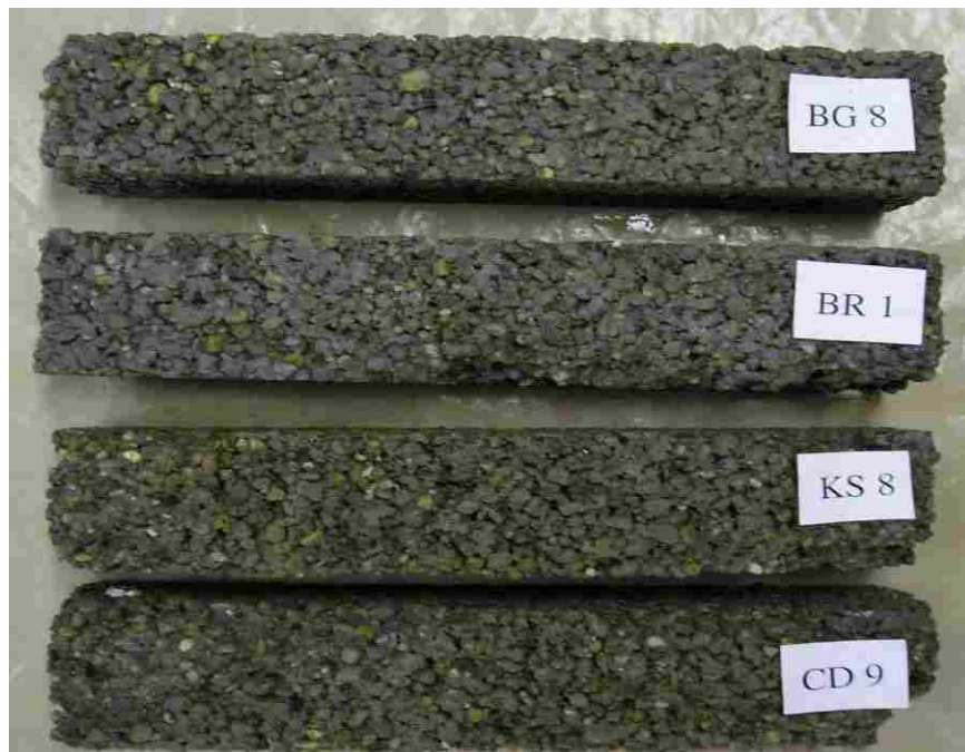
Figure K.6 Unclogged, saturated specimens after 90-day cure and 120 freeze-thaw cycles.
