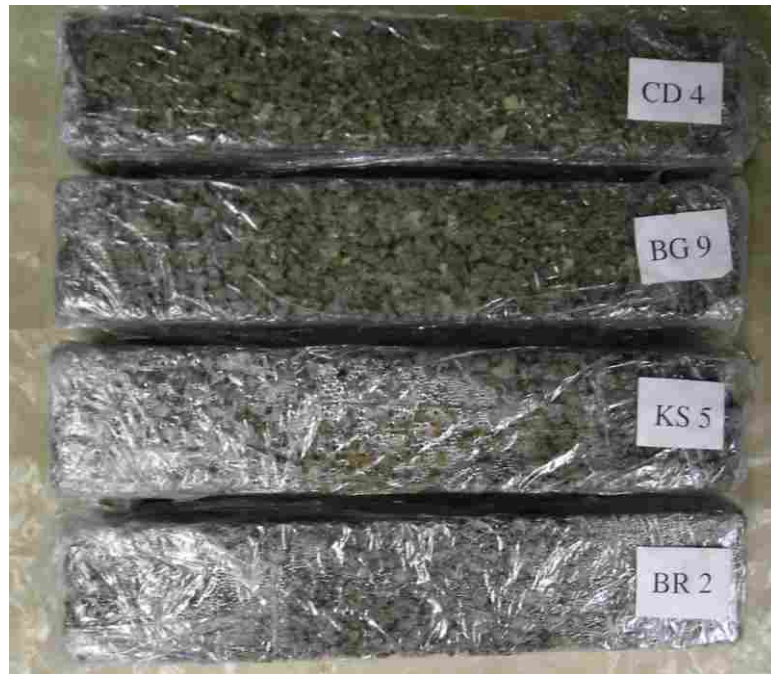
Figure L.13 Unclogged, unsaturated specimens after 90-day cure and 260 freeze-thaw cycles.
