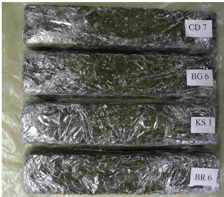
Figure J.12 Clogged, unsaturated specimens after 90-day cure and 240 freeze-thaw cycles.
