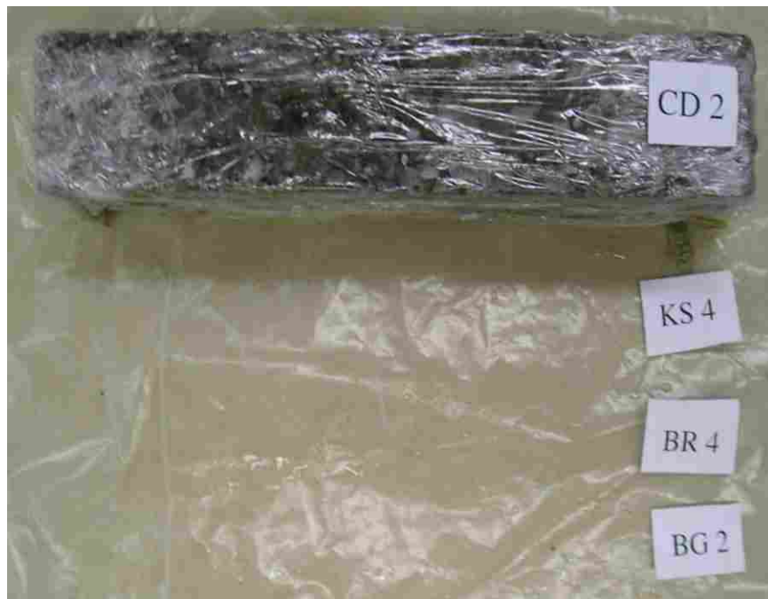
Figure F.15 Unsaturated, clogged specimens after 28-day cure and 300 freeze-thaw cycles.
