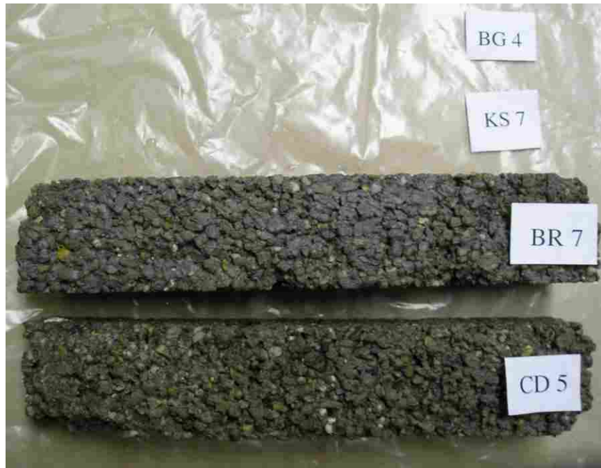
Figure G.11 Unclogged, saturated specimens after 28-day cure and 220 freeze-thaw cycles.
