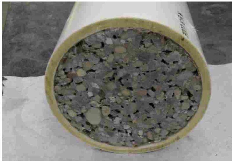
FIGURE 3.9 Laboratory permeability test specimen fully inserted into pipe.
