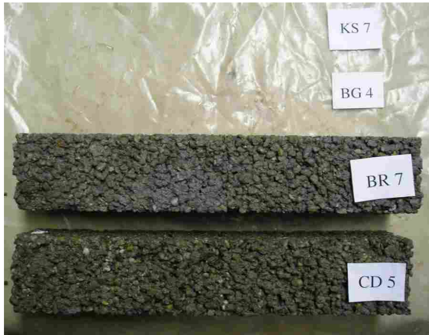
Figure G.7 Unclogged, saturated specimens after 28-day cure and 141 freeze-thaw cycles.
