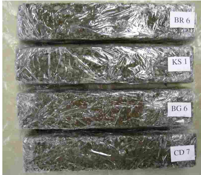
Figure J.9 Clogged, unsaturated specimens after 90-day cure and 180 freeze-thaw cycles.
