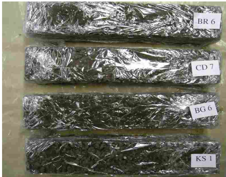
Figure J.15 Clogged, unsaturated specimens after 90-day cure and 306 freeze-thaw cycles.
