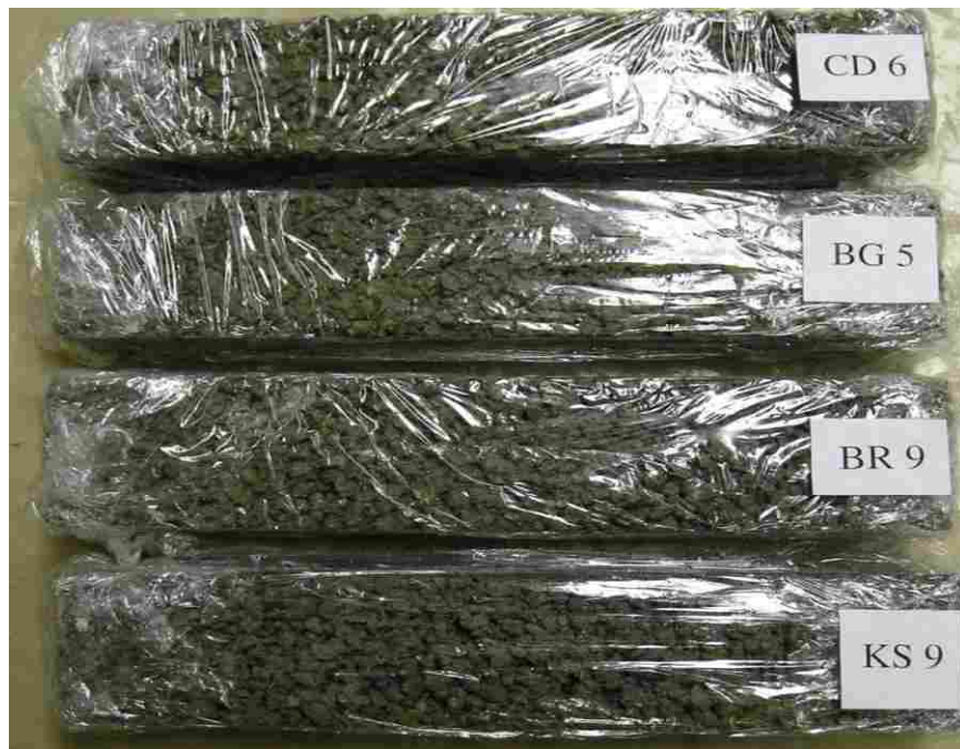
Figure H.4 Unclogged, unsaturated specimens after 28-day cure and 81 freeze-thaw cycles.
