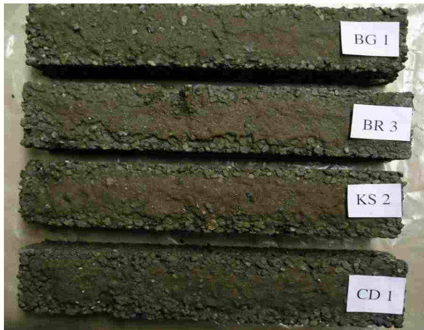
Figure E.6 Clogged, saturated specimens after 28-day cure and 121 freeze-thaw cycles.
