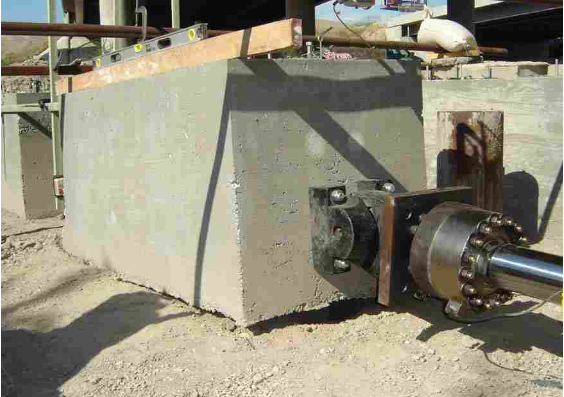
Figure 5-7 Photograph of Test Cap 1 at failure.
