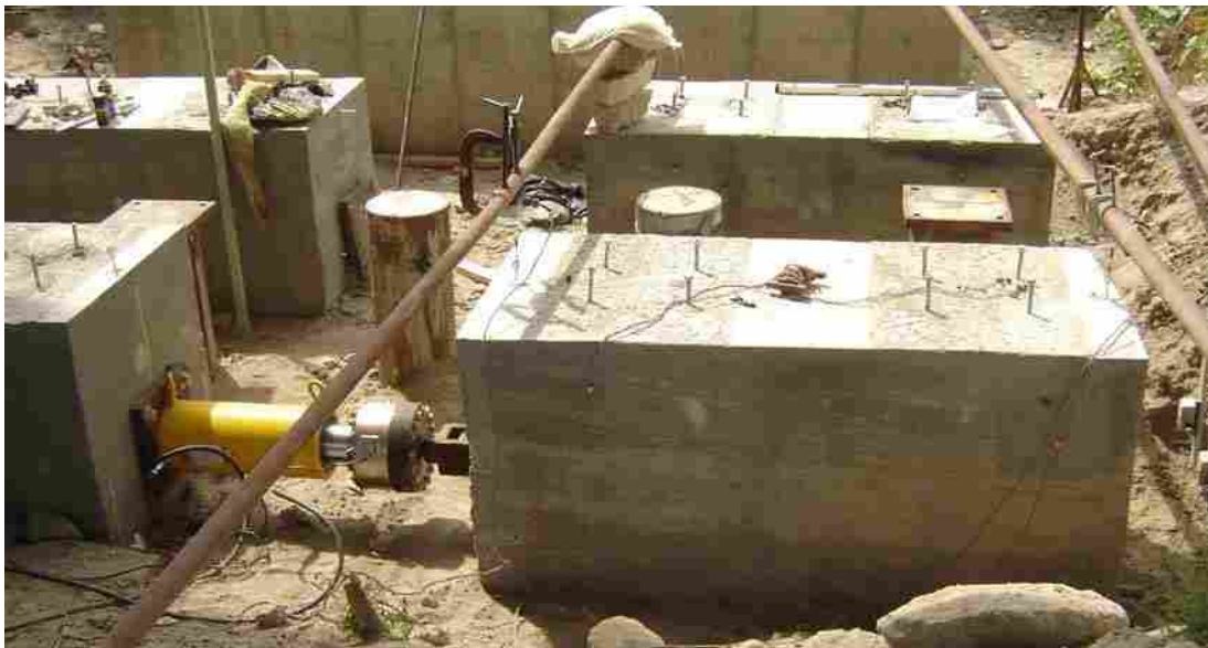
Figure 3-19 Side view of test setup prior to loading Pile Cap 3.
