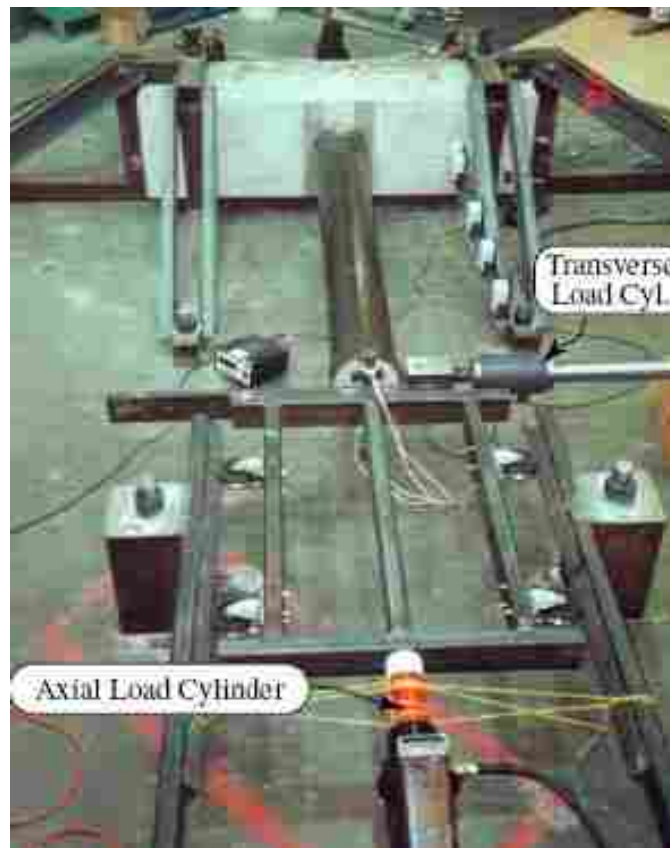
Figure 2-5 Pile and cap setup for testing at Montana State University.
