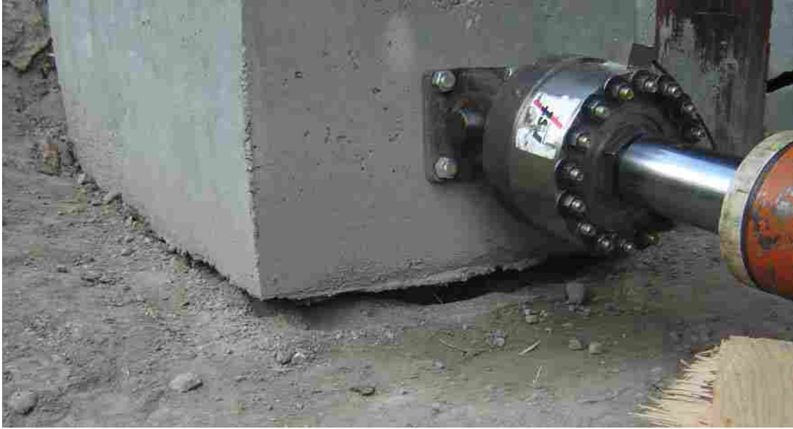
Figure 5-18 Test Cap 4 at failure.
