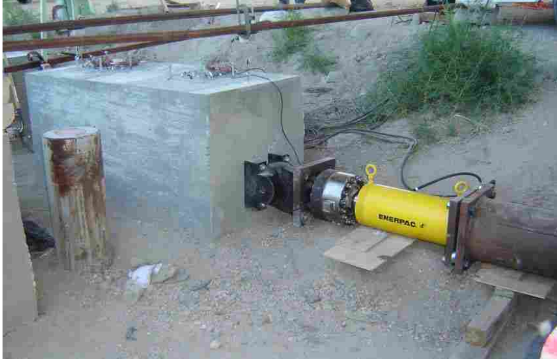
Figure 3-16 Photograph of test set-up for Pile Cap 2.
