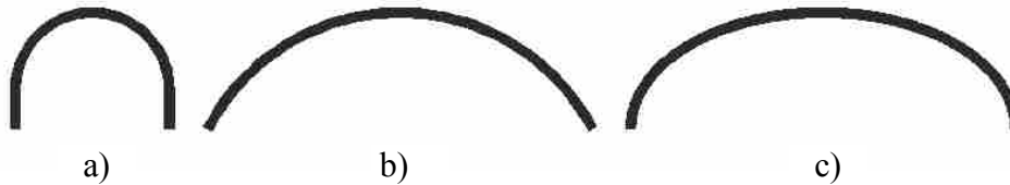
Figure 2-1 – Common arch types are a) semicircular, b) segmental, and c) elliptical
