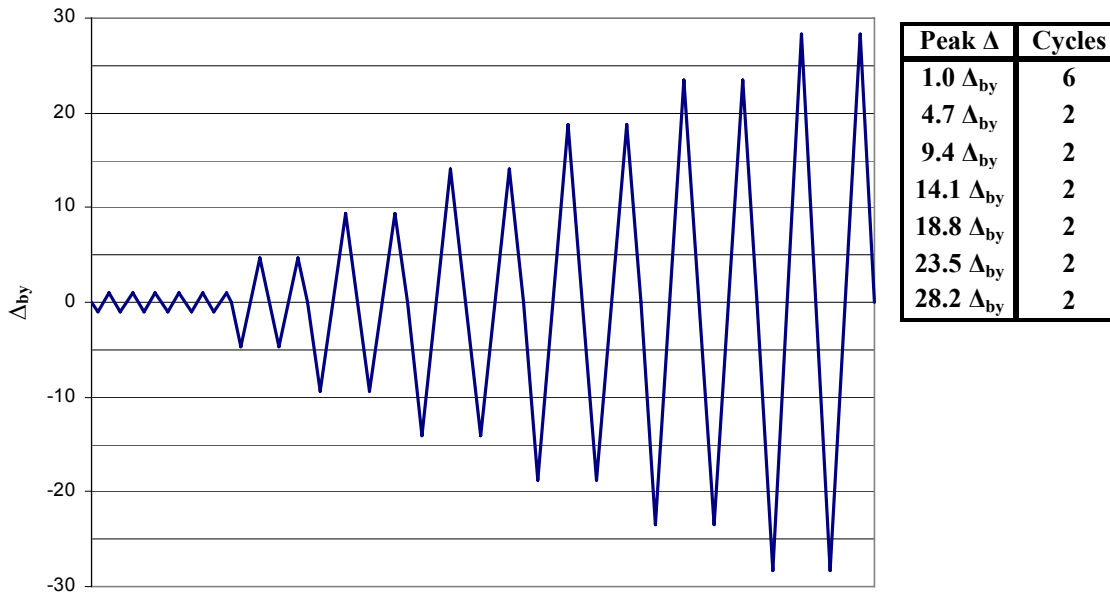
Figure 2-8 Specimen 1 – Loading Protocol with Respect to Yield Deformation
