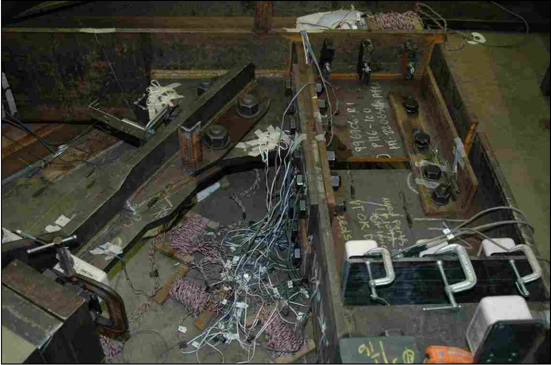
Figure 2-16 Specimen 1 – Gusset and Splice Plate Instrumentation
