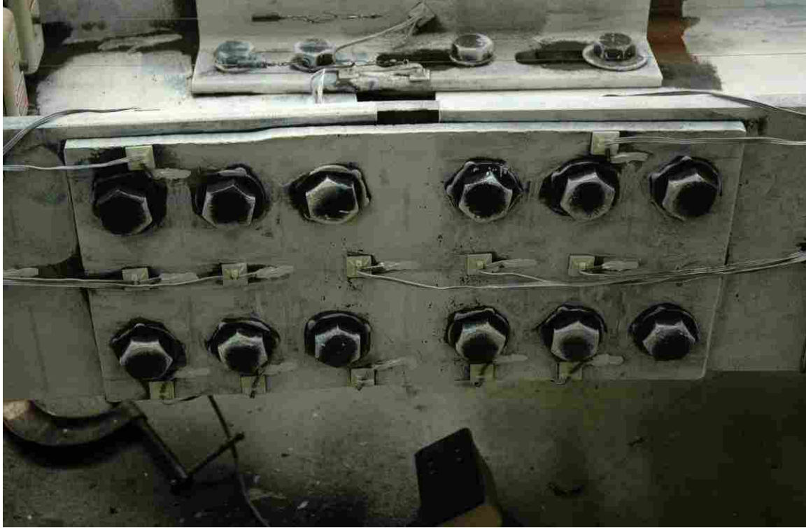
Figure 3-24 Specimen 2 – Minor Yielding of Outer Splice Plate (6.5% Drift)
