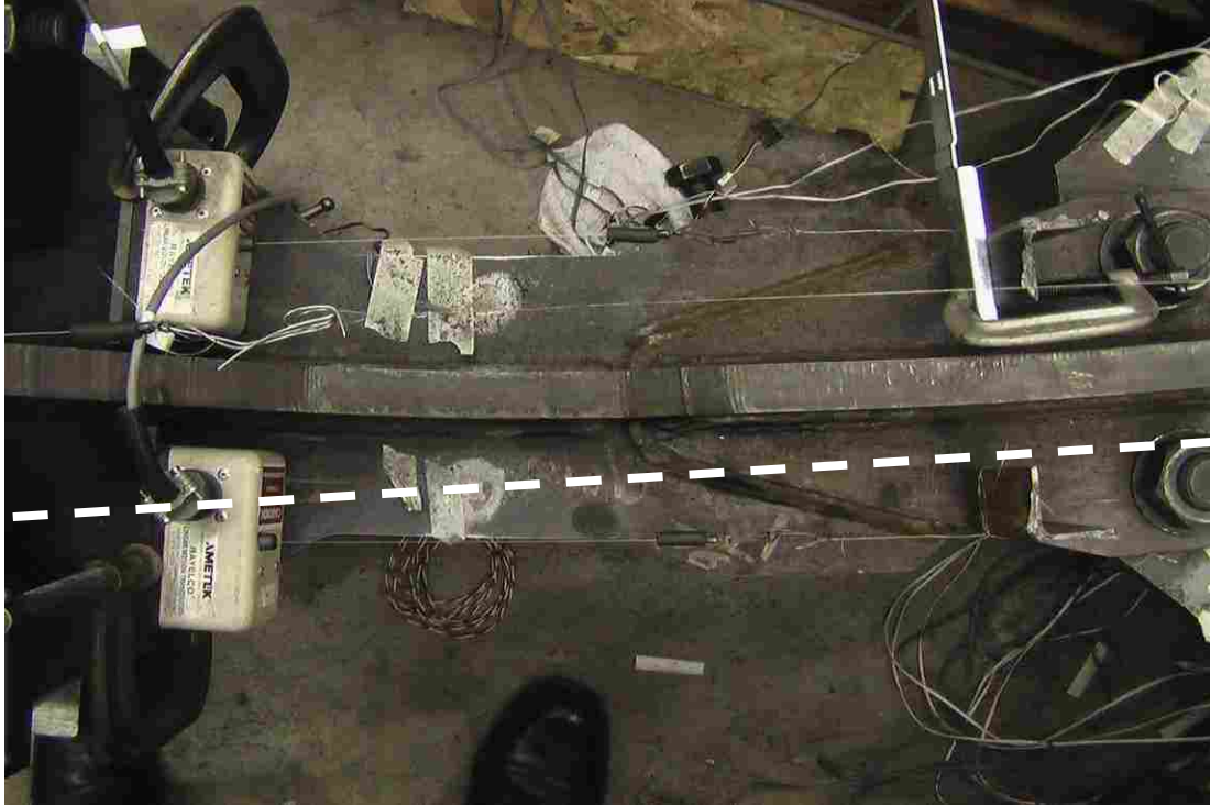
Figure 3-5 Specimen 1 – Core Extension Deformation Following Boundary Failure
