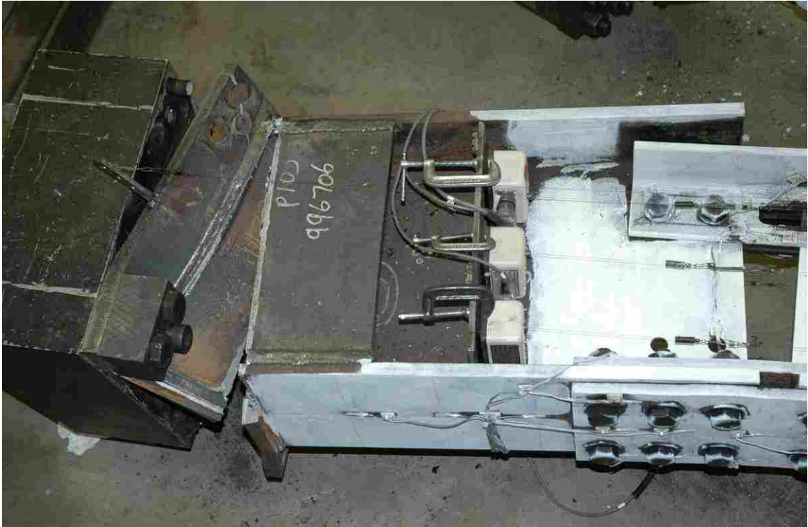
Figure 3-26 Specimen 2 – Boundary Plate Failure
