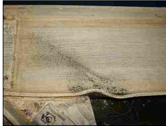
(b) Yielding and Buckling of Beam
