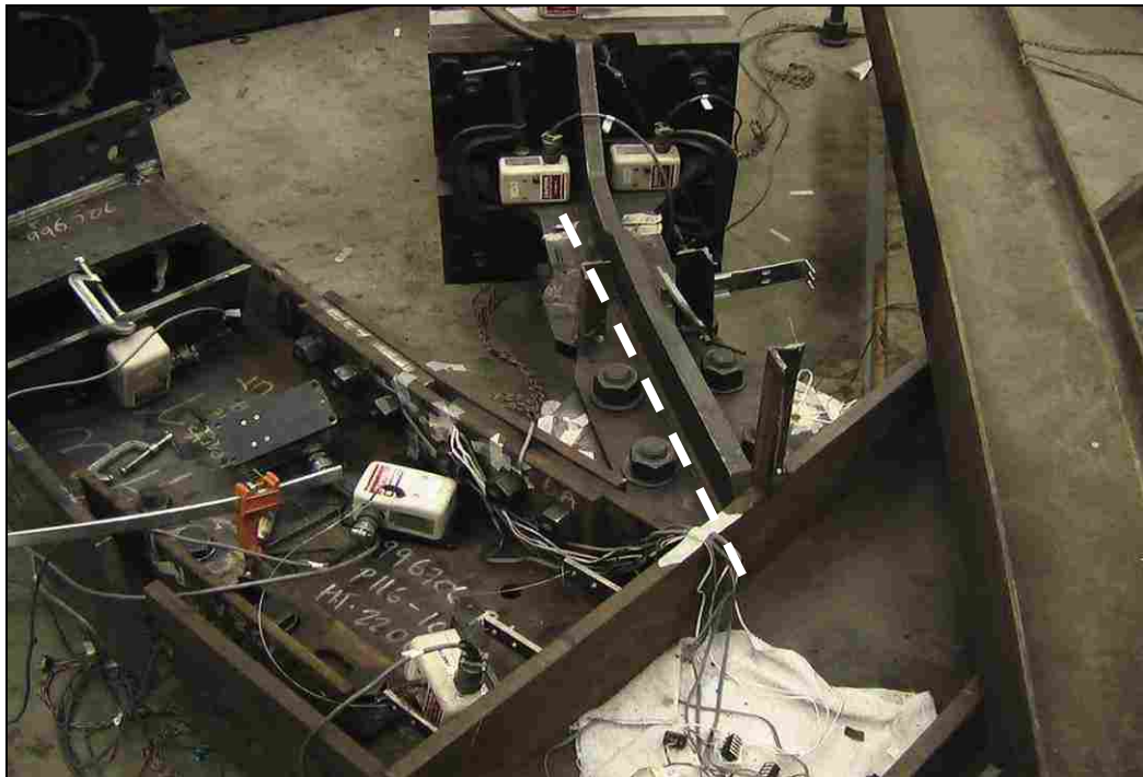
Figure 3-4 Specimen 1 – Connection Deformation Following Boundary Failure
