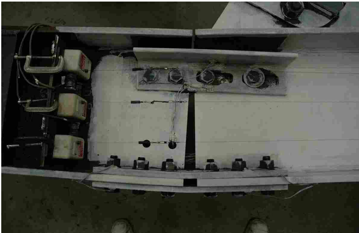
Figure 3-21 Specimen 2 – Deformation of Splice Plates (4% Drift)
