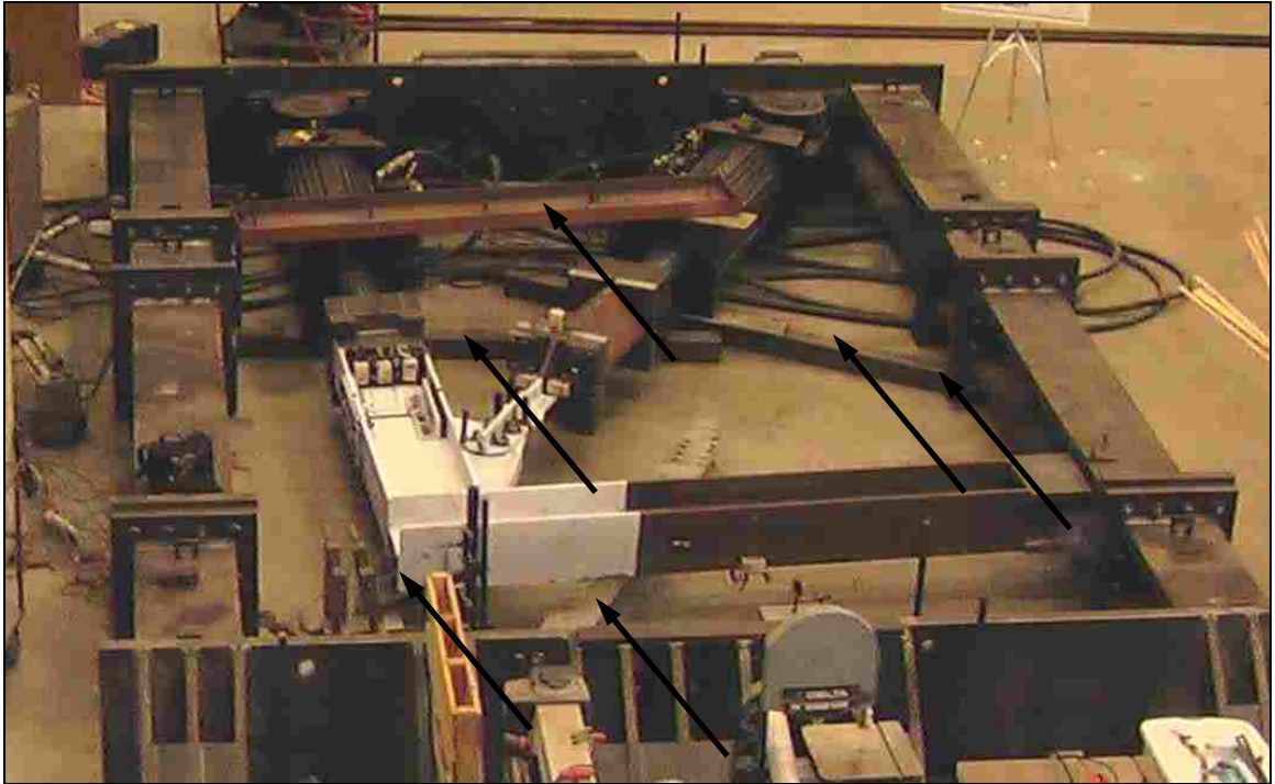
Figure 2-7 Specimen 2 – Out-of-Plane Bracing
