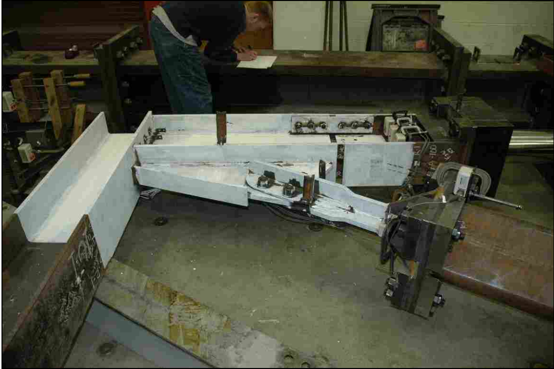
Figure 2-22 Specimen 2 –Instrumentation (Side View)
