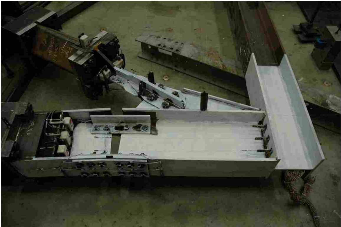
Figure 3-23 Specimen 2 – No Undesirable Failure Modes in Specimen (6.5% Drift)
