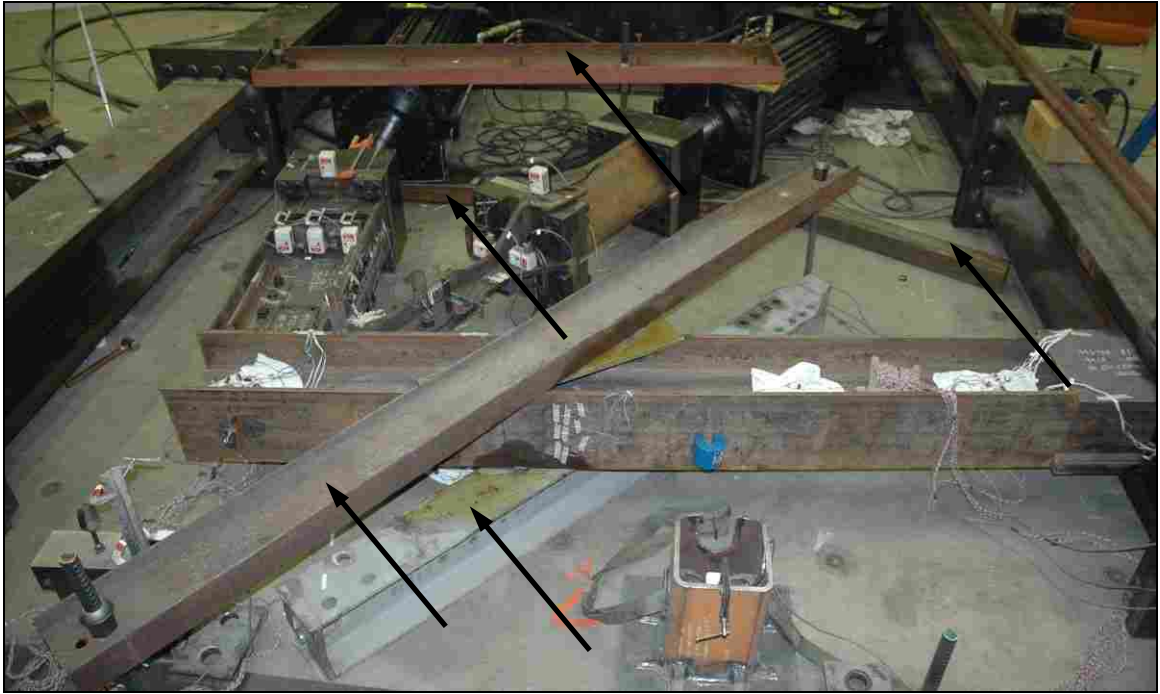
Figure 2-6 Specimen 1 – Out-of-Plane Bracing
