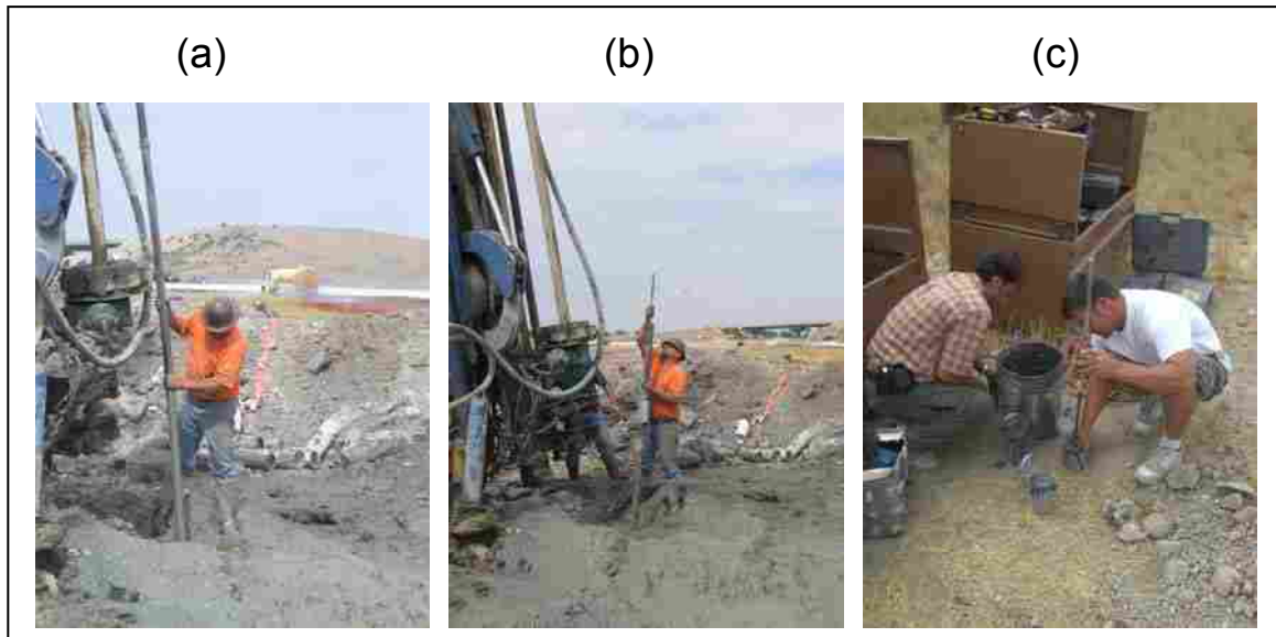
Figure 5-8 Photos taken during (a) insertion of sampling pipe to desired depth, (b) extrusion of small pipe connected to the sampling pipe plug , and (c) rodding of wet grab samples in plastic molds.
