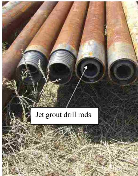
Figure 5-3 Jet grout drill rods with central pipe for cement slurry and annular space for compressed air.
