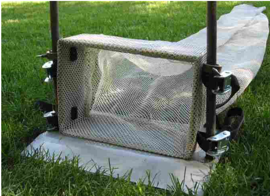
Figure 1-2. One of 12 Bunte-Abt traps built and deployed at sample Sites 1-4.
