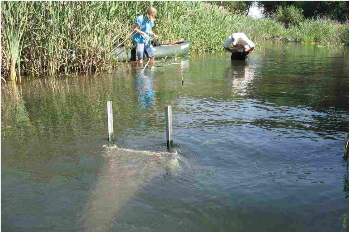
Figure F-2. Drift bead sample net halfway between the streambed and water surface. This is the net located 2.4 km downstream from the starting location.
