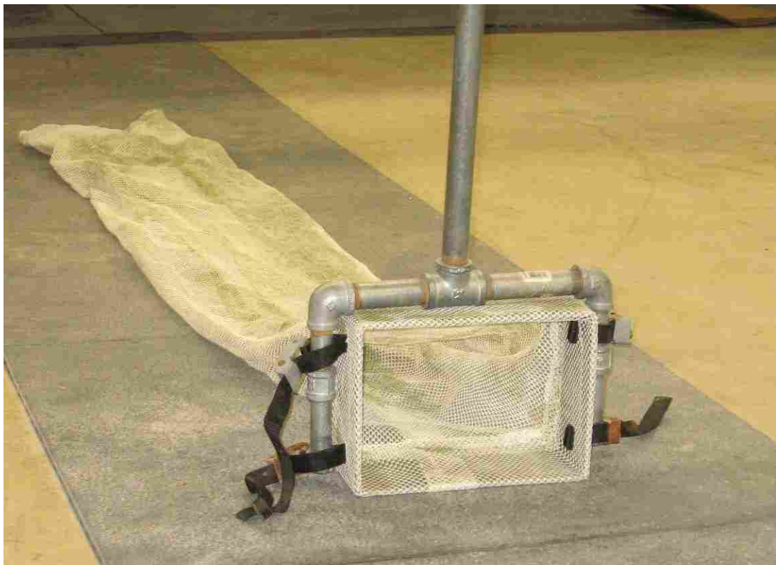
Figure 1-3. This hand-held variation of the Bunte-Abt trap requires no wading.
