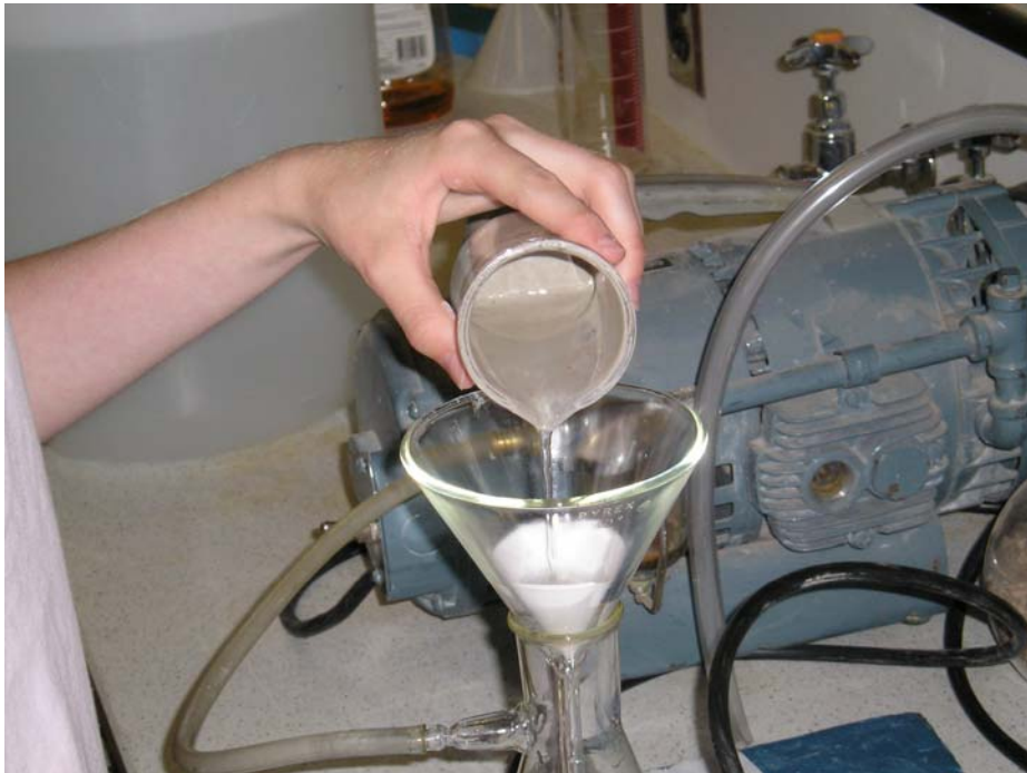
FIGURE 3.7 Filtering a chloride concentration sample.
