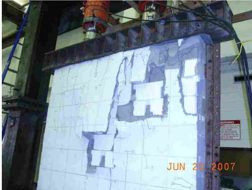
Figure 6.4 Wall #7 at Failure
