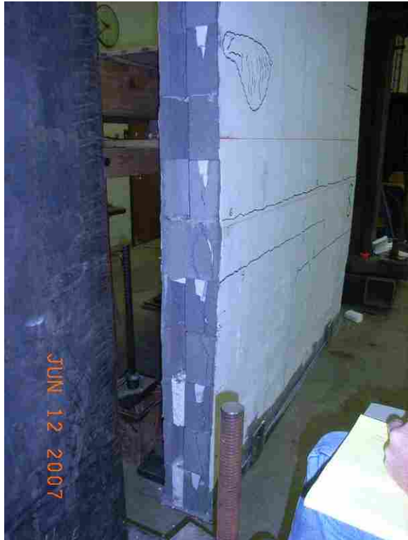
Cracking in the Sides of the Wall (wall #8)
