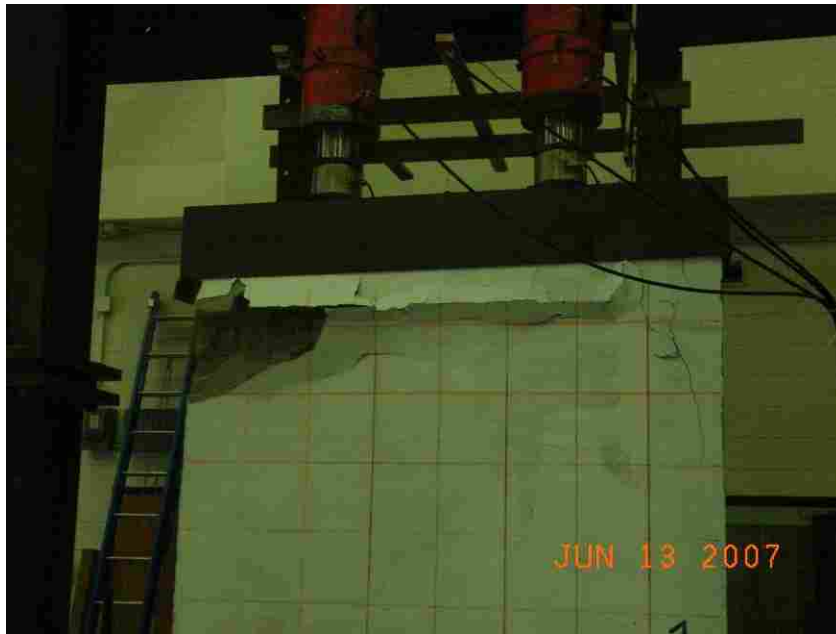
Figure 6.1 Wall #1 at Failure
