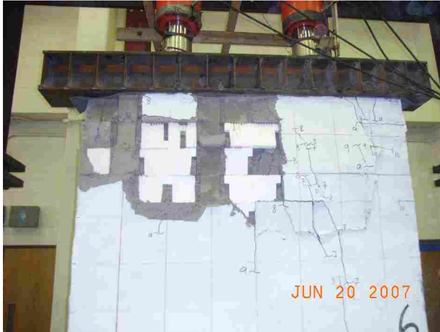
Figure 6.3 Wall #6 at Failure
