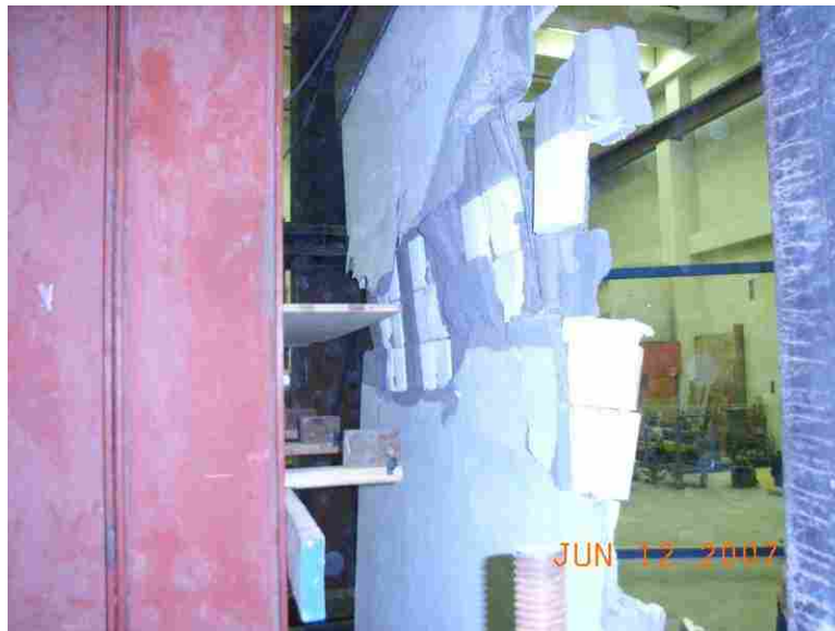
Buckling of Wall at Failure (wall #8)
