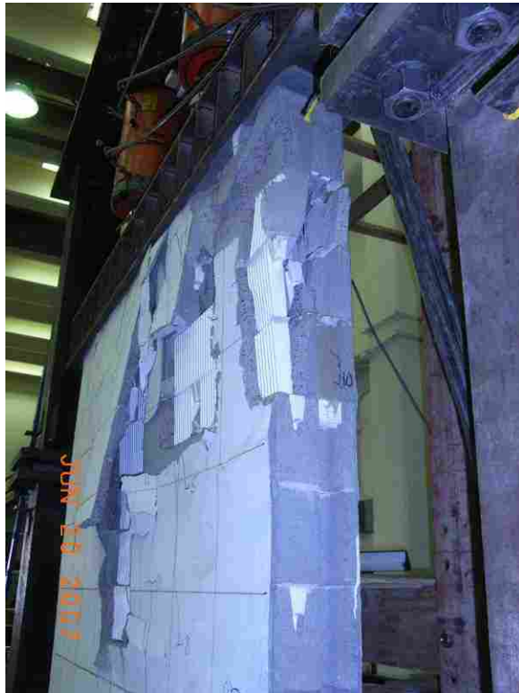
Close-up of Failure at West Side of Wall (wall #7)
