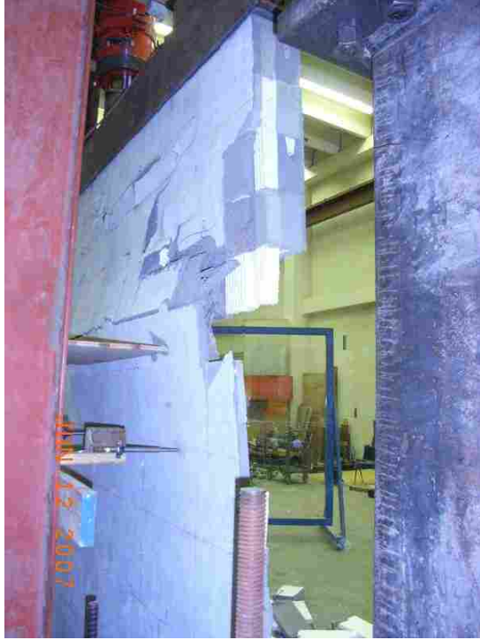
Buckling of Wall at Failure (wall #9)
