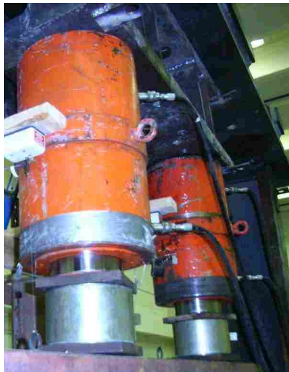
Figure 4.5 Hydraulic Jacks and Load Cells
