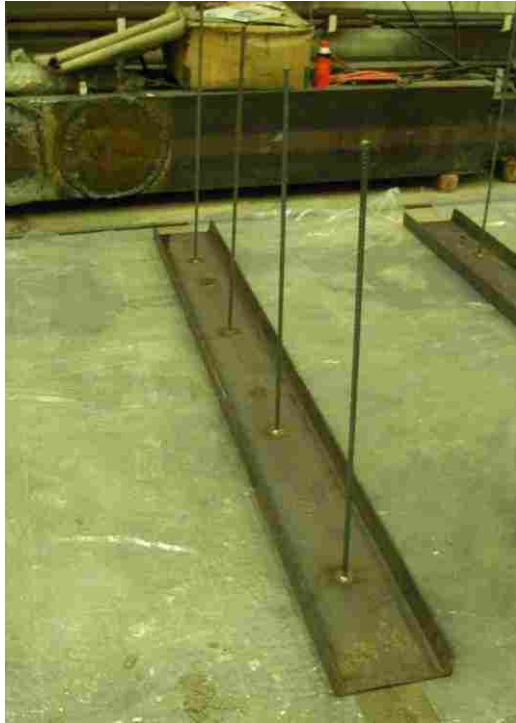
Figure 4.1 Rebar and Steel Channel
