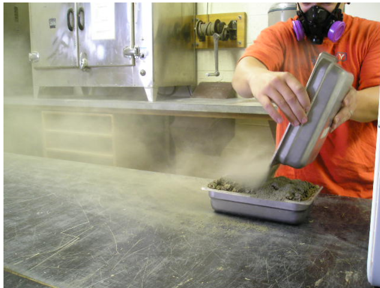
Figure 3.1 Cement powder dispersion during blow test.
