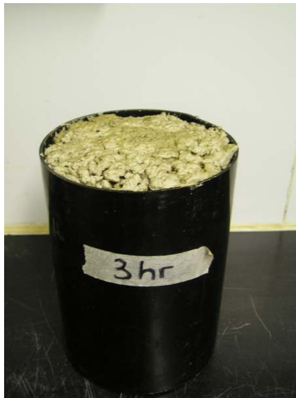
Figure 3.2 Specimen of base material prepared for conditioning.
