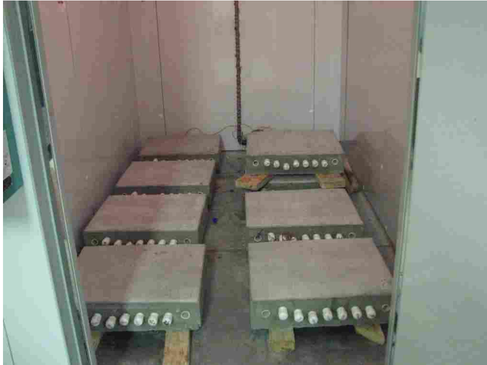
FIGURE 3.10 Slabs inside environmental chamber.
