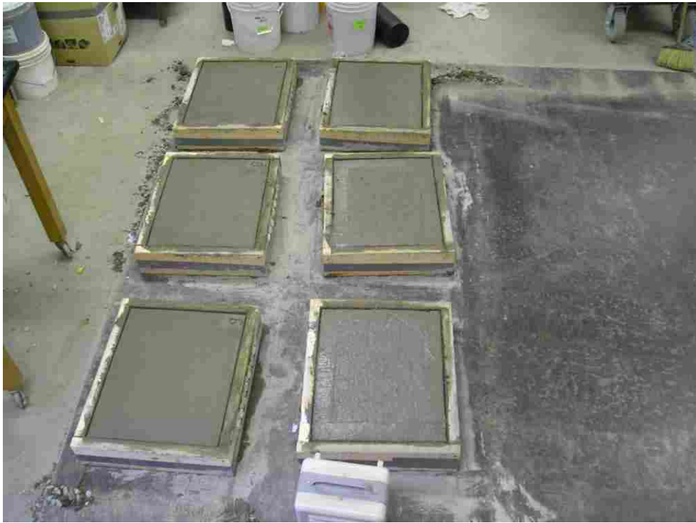
FIGURE 3.9 Slab casting layout.
