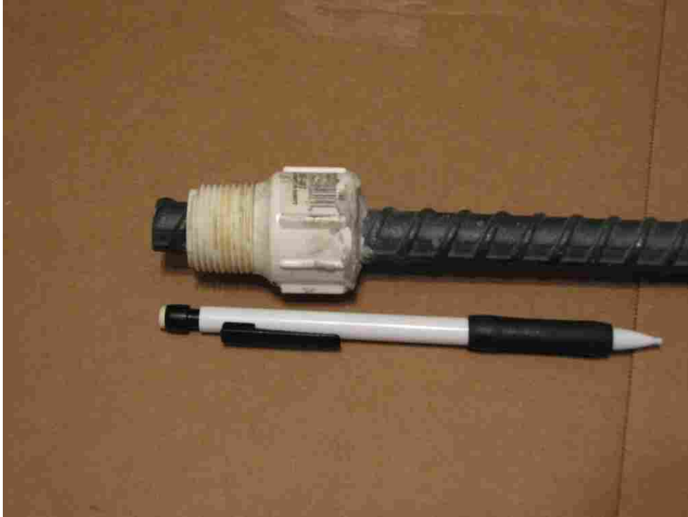
FIGURE 3.5 PVC fitting bonded to a length of rebar.
