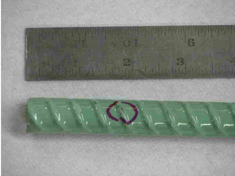
FIGURE 3.3 Epoxy-coated rebar with damage from pliers strike.
