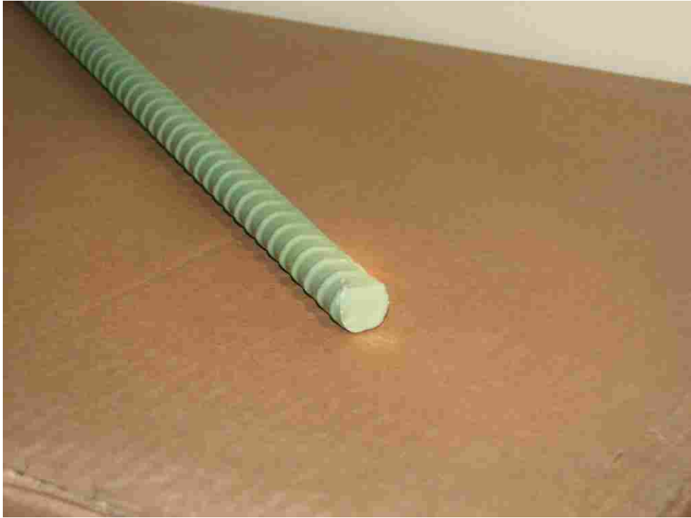
FIGURE 3.1 Epoxy-coated rebar with repaired end cut.
