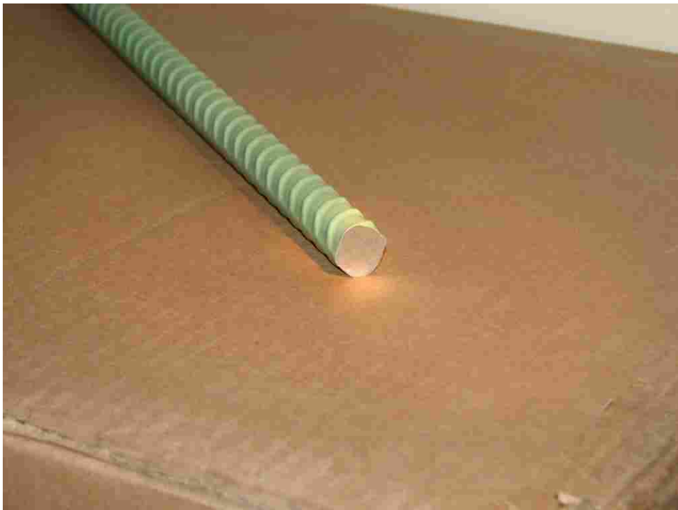
FIGURE 3.2 Epoxy-coated rebar with end cut not repaired.
