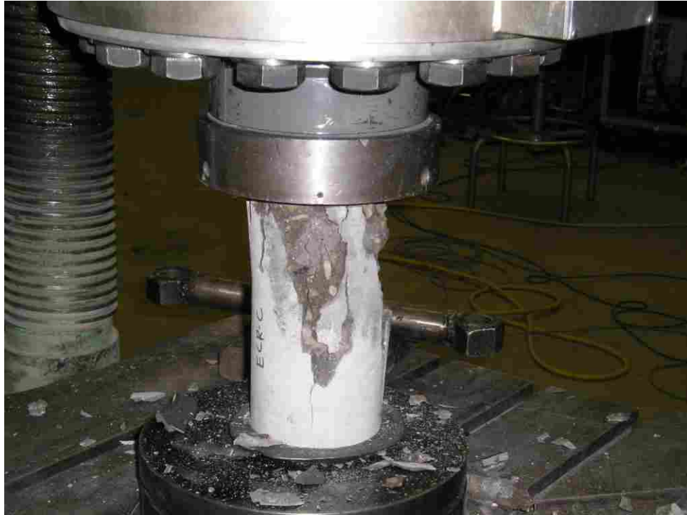
FIGURE 3.15 Compressive strength testing.
