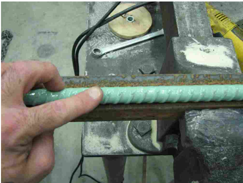
FIGURE 3.4 Epoxy-coated rebar with damage from rib scrape.
