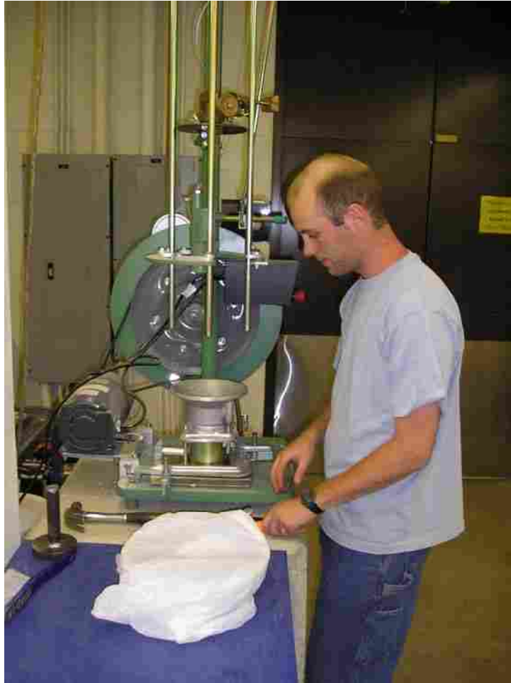
FIGURE 3.12 Compacting a sample.
