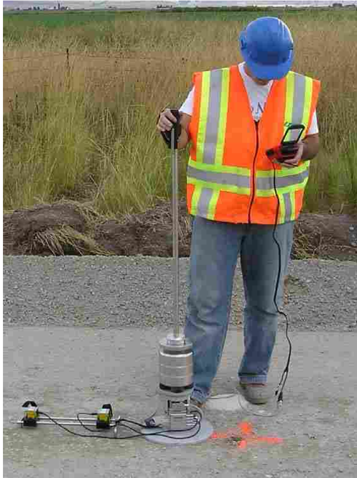
FIGURE 2.4 Portable falling-weight deflectometer.
