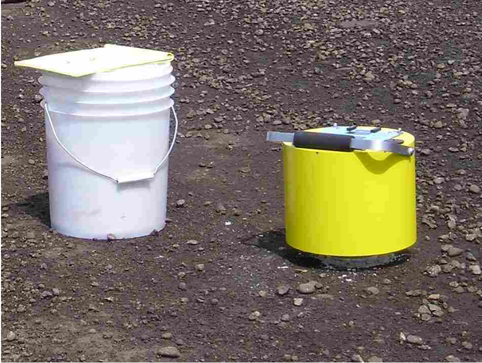
FIGURE 2.1 Soil stiffness gauge with bucket of moist sand.
