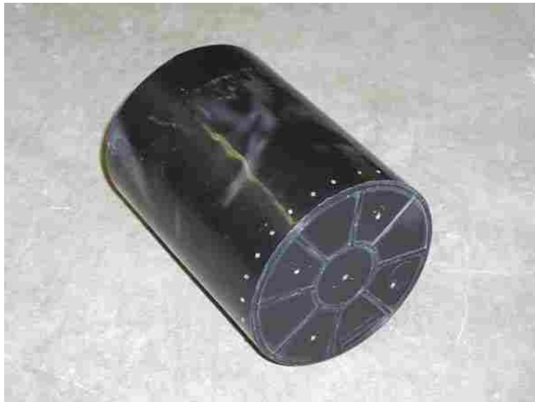
Figure 3.12 Plastic mold used for tube suction test.
