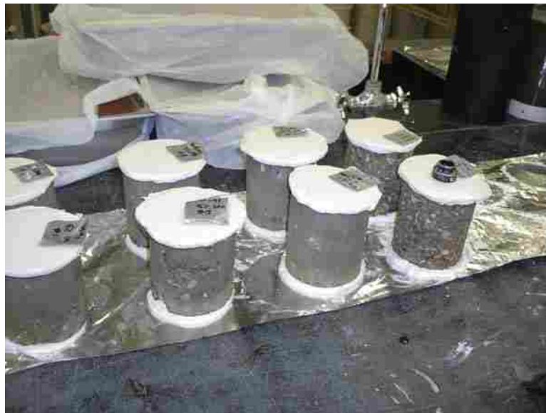
Figure 3.3 Specimens capped for UCS testing.
