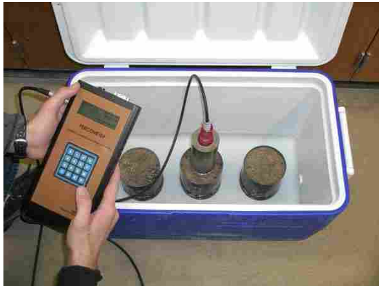
Figure 3.13 Tube suction test configuration.
