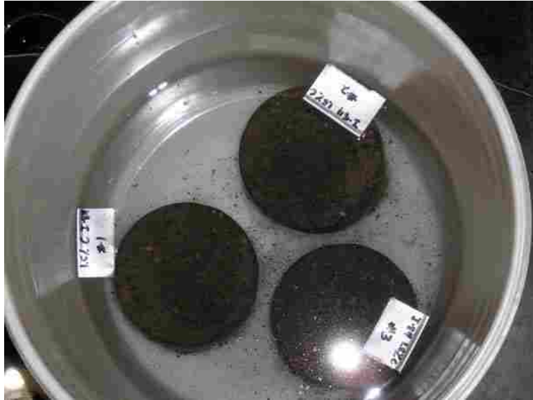
Figure 3.9 Soaking configuration for freeze-thaw testing.
