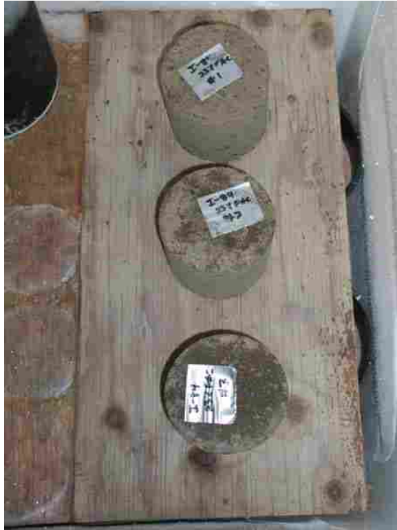
Figure 3.7 Freezing configuration for freeze-thaw testing.
