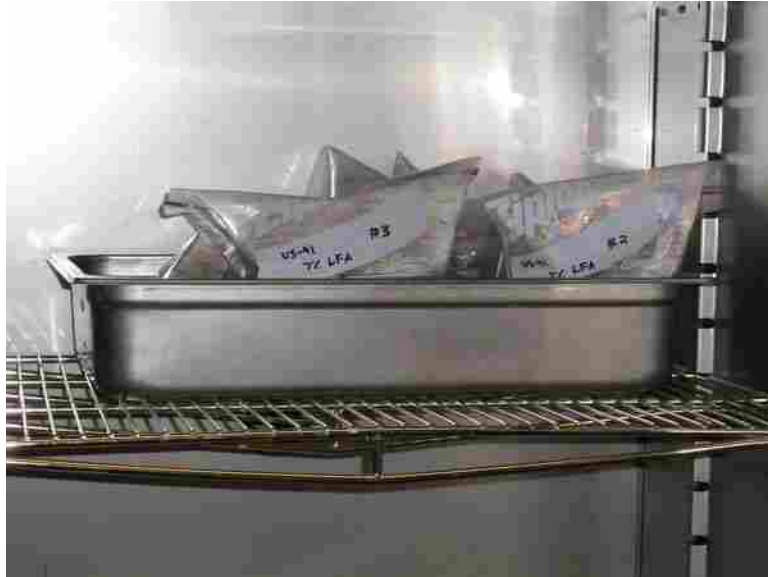
Figure 3.5 Curing conditions for specimens treated with Class C fly ash and lime-fly ash.
