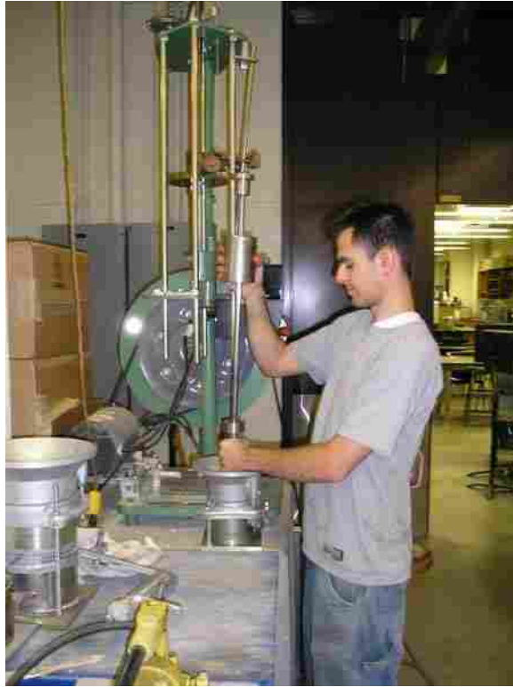
Figure 3.1 Compaction apparatus and finishing tool.
