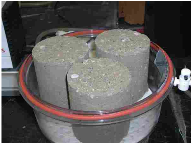
Figure 3.10 Vacuum chamber used for vacuum saturation test.
