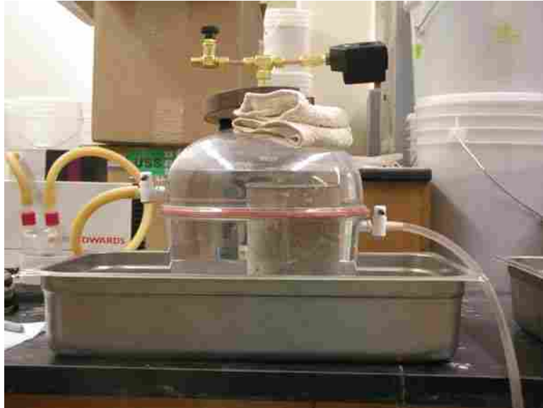
Figure 3.11 Vacuum saturation test configuration.
