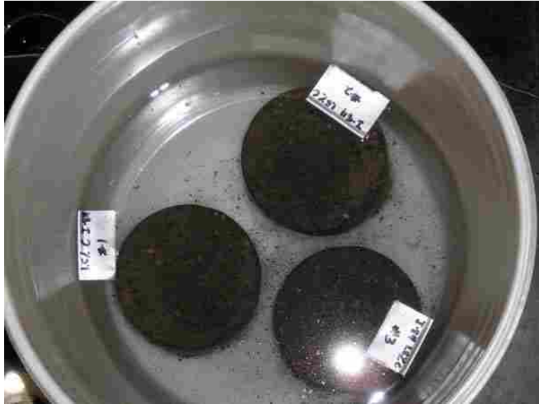
Figure 3.6 Specimens soaking prior to UCS testing.
