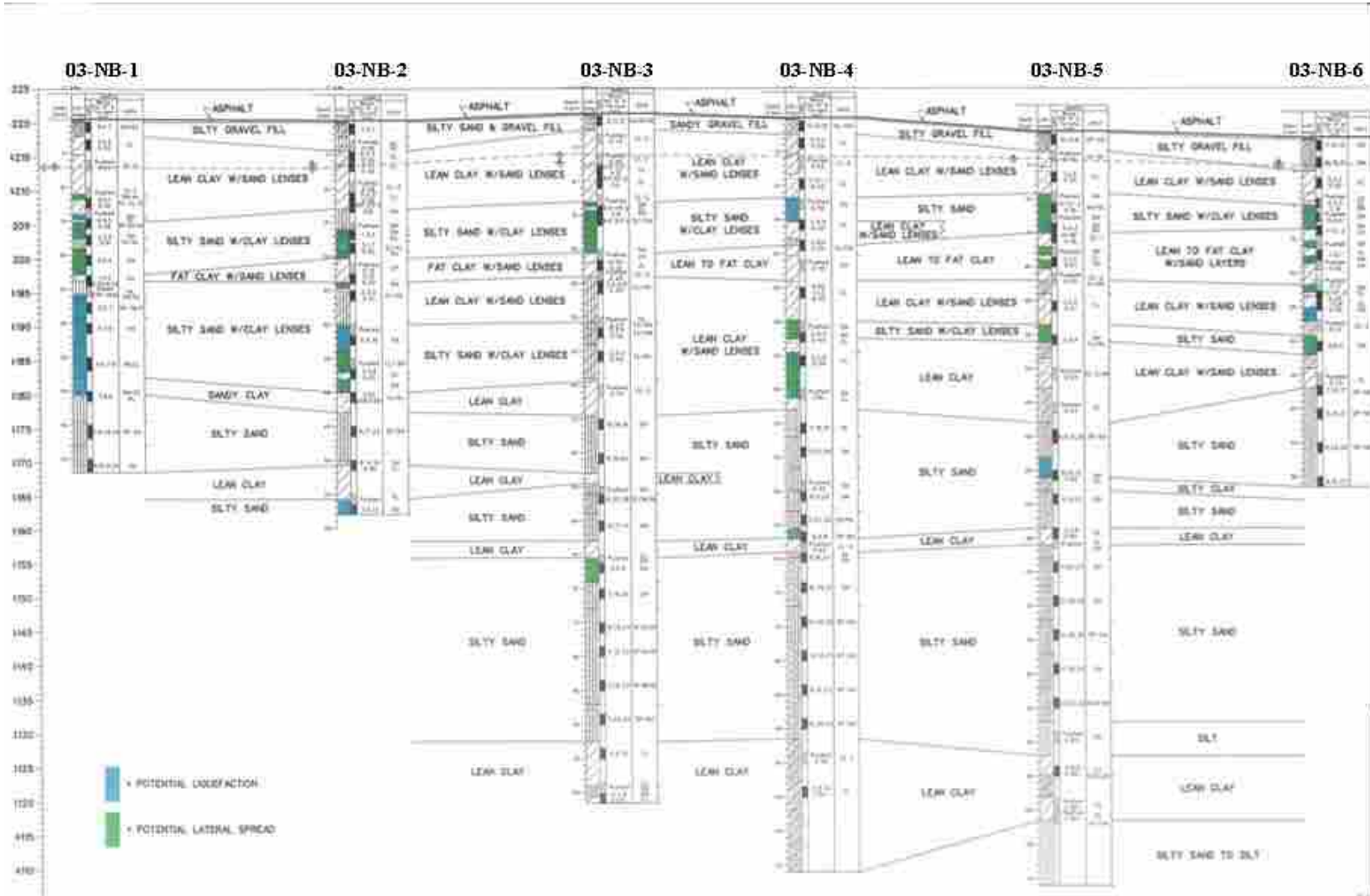
Figure 3-14 Fence Diagram of Borehole Logs Near Test Site
