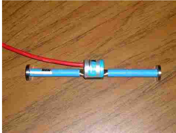
Figure 4-5 Vibrating Wire Strain Gauge Model 4200 used for Installations in Salt Lake City, UT
