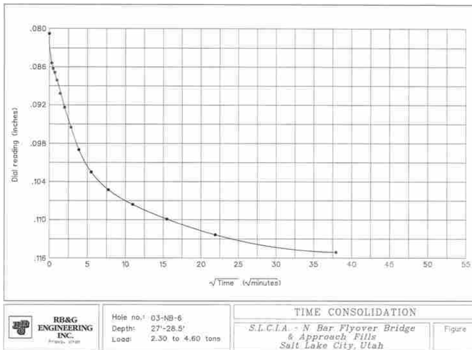
Figure A-33 Square Root of Time Series Curve for Sample from Boring 03-NB-6, 27' - 28.5', 2.3 to 4.6 Tons
