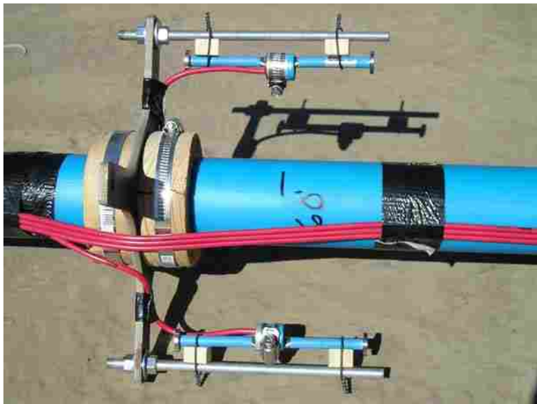
Figure 4-7 Completed Assembly of Star and Gauges Attached to Inclinometer Pipe for Installation
