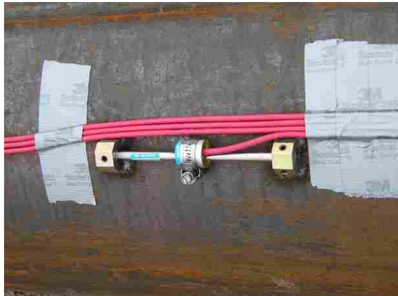
Figure 4-4 Placement of Gauge and Wires along Pile
