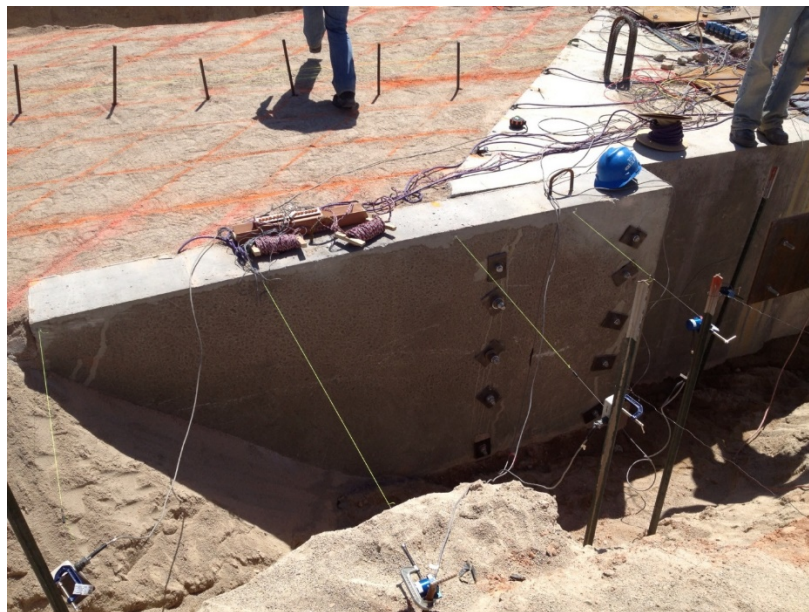
Figure 3.16. String potentiometers measuring lateral deflection (Smith 2014).
