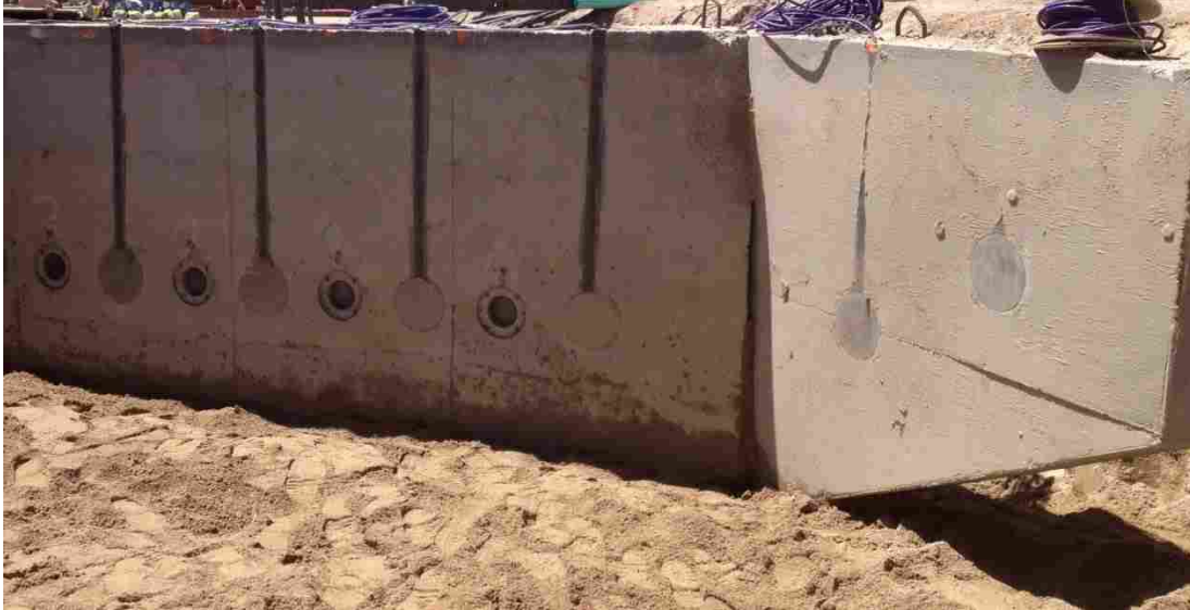
Figure 3.15. Geokon® pressure cell distribution along each wingwall (Smith 2014).
