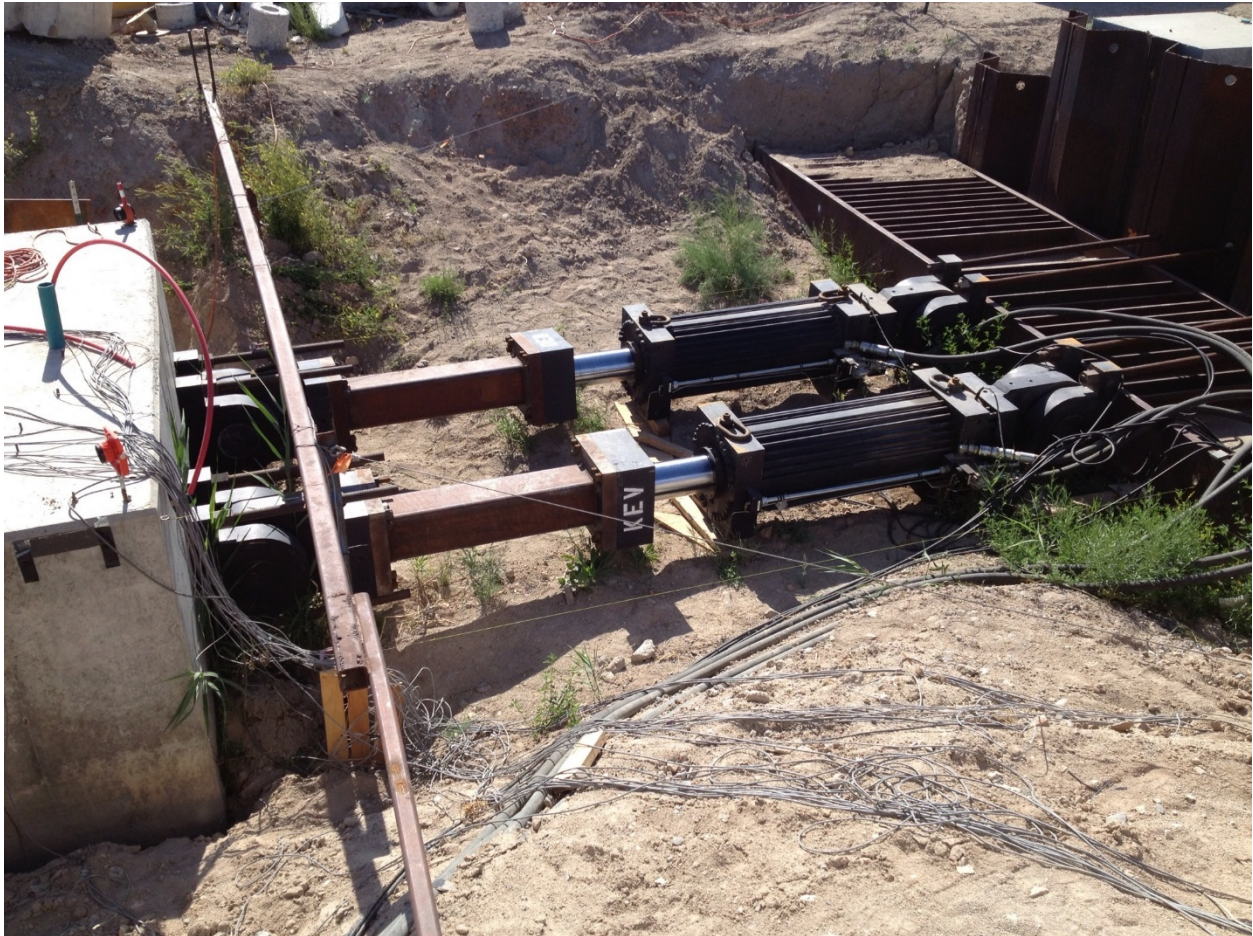
Figure 3.8. Two MTS actuators connecting the pile cap and reaction foundation.
