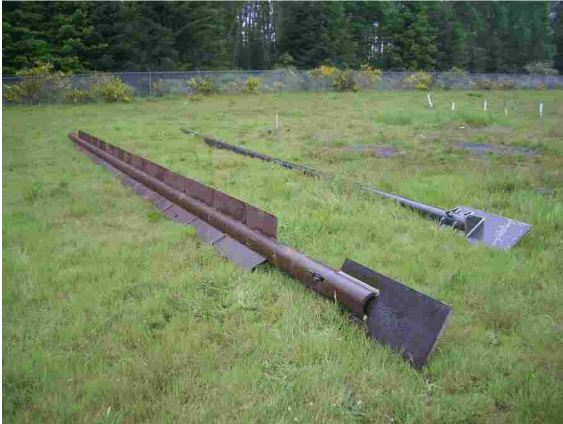
Figure 4.3 Mandrels used in EQDrain and blast hole installation. Mandrel on left has three “fins” designed to transfer vibrational energy to surrounding soil. Mandrel on right is smooth.
