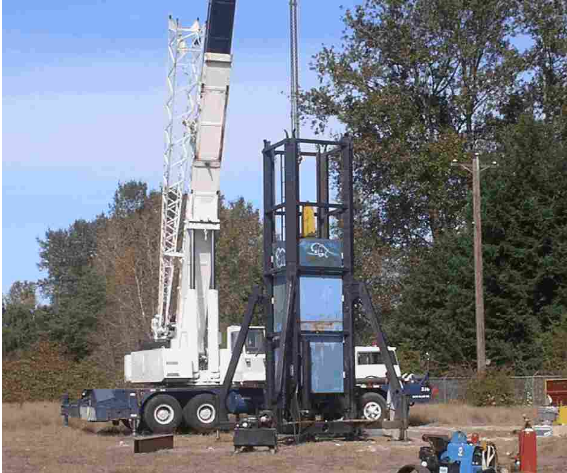
Figure 10.3 Photograph of the static testing apparatus installed at Site 4.
