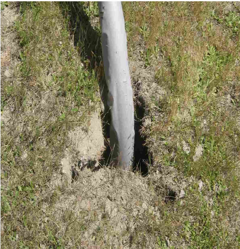
Figure 7.6 View of localized settlement surrounding an EQ Drain. Localized settlement immediately surrounding the drains commonly exceeded 300 mm.
