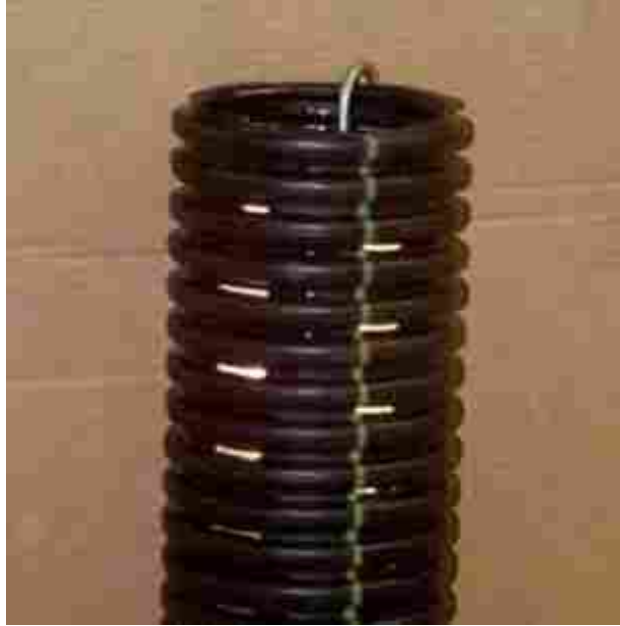
Figure 7.1 Section of EQ Drain; light suspended on the inside illuminates the slots (after Rollins and Anderson, 2002).
