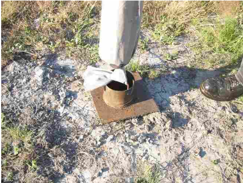
Figure 4.4 Photograph of an EQDrain tied to an anchor. Anchors measured 305 mm x 305 mm x 12.5 mm. Generally, the anchors had the corners bent over; this one did not.
