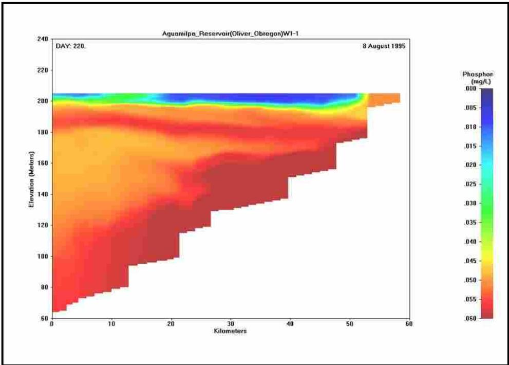
Figure 4-6: Phosphorous Example Simulation Branch 1 (Santiago River)
