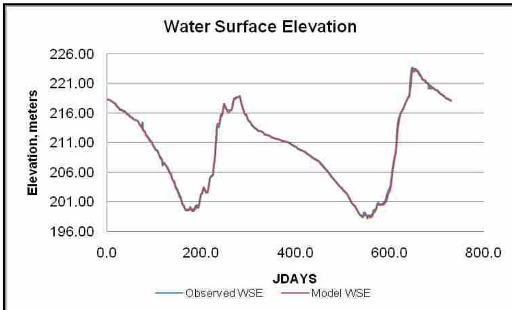
Figure 4-2: Water Balance Calibration of the Aguamilpa Reservoir
