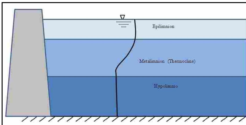
**Figure 2-5: Reservoir Stratification**
