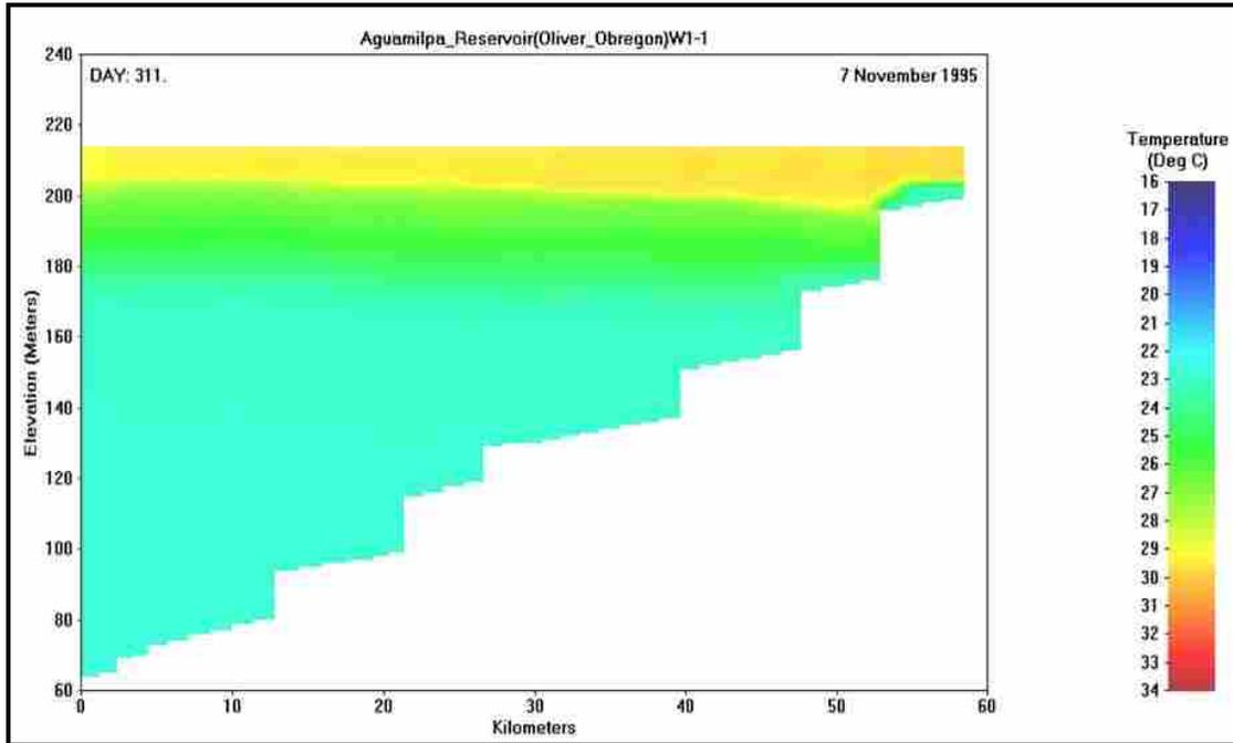
**Figure 4-3: Water Temperature Simulation for Branch 1 (Santiago River)**
