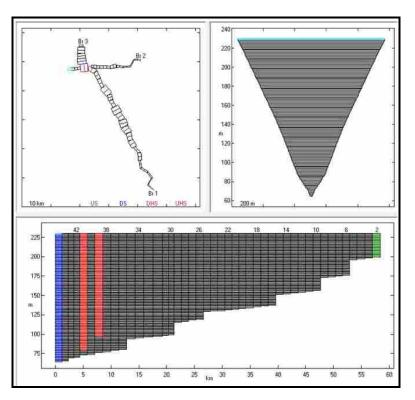
Figure 3-4: W2 Bathymetry Grid of Branch 1 (Santiago River)
