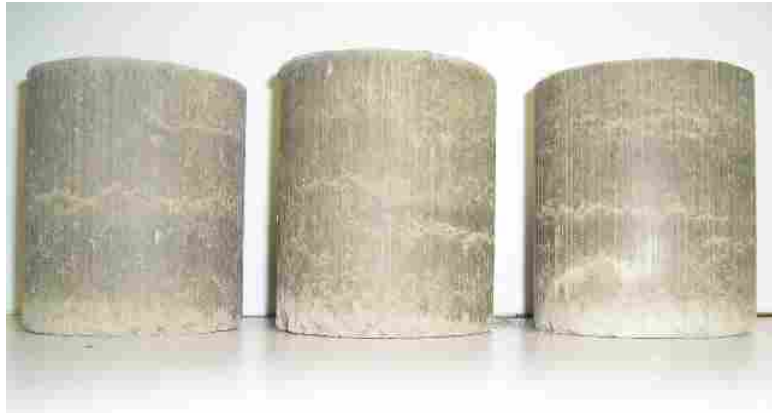
Figure B.13 Clay specimens treated with 10 percent Class C fly ash after 0 cycles of freeze-thaw testing.
