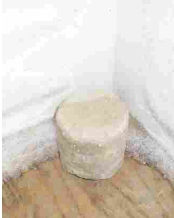
Figure 3.5 Freezing configuration for freeze-thaw testing.
