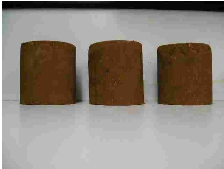
Figure 3.6 Thawing configuration for freeze-thaw testing.
