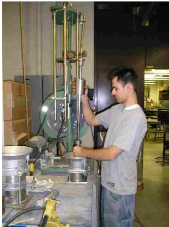
Figure 3.1 Compaction apparatus and finishing tool.
