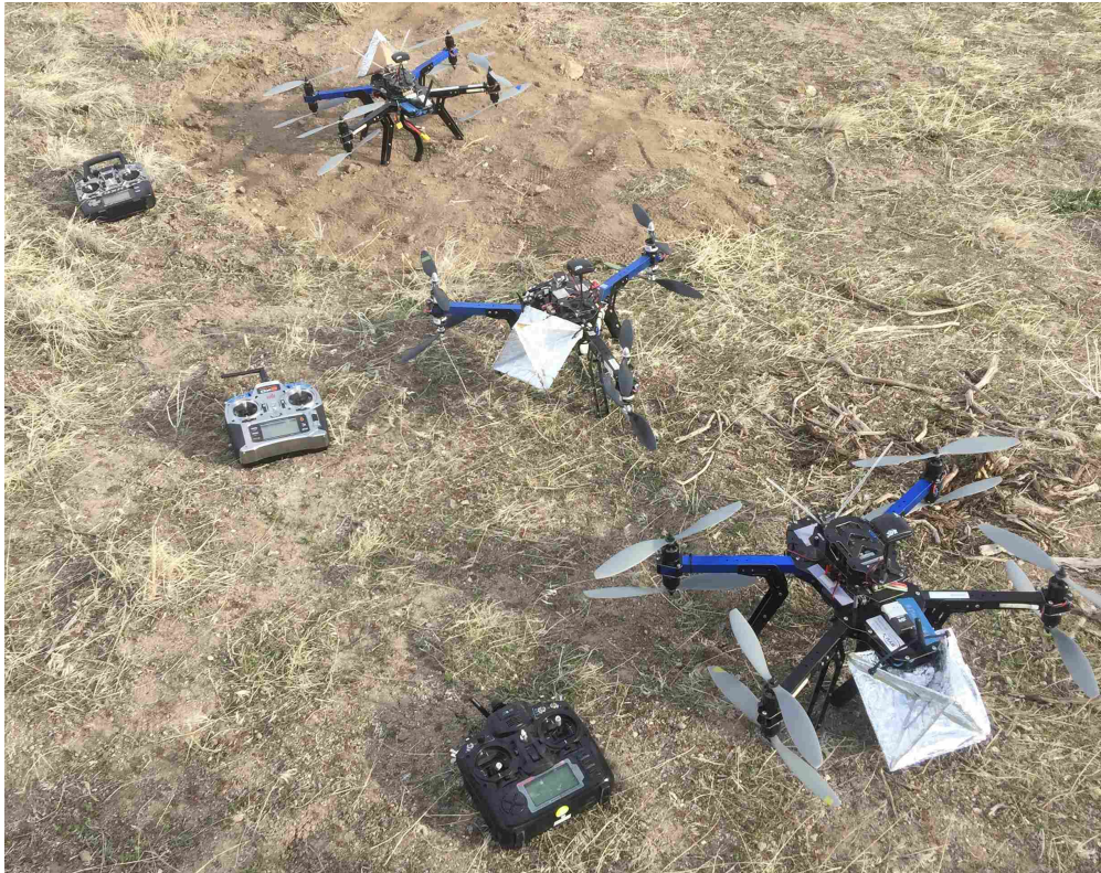
Figure 5.12: 3DR X8 and Y6 aircraft used in flight test with corner reflectors.
