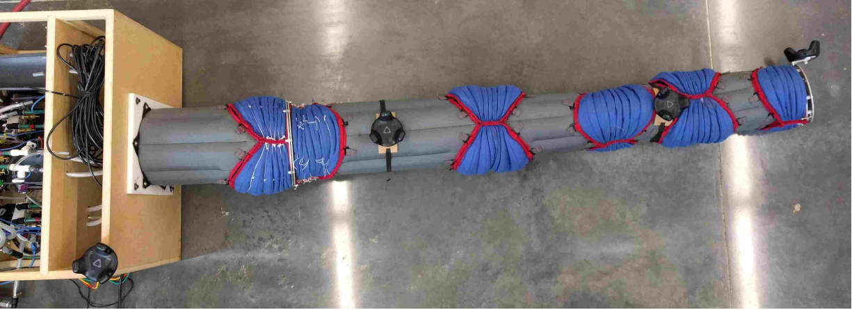
Figure 2.6: The Vive trackers are attached to Kaa as shown here and are used for estimating joint angles and end effector pose.
