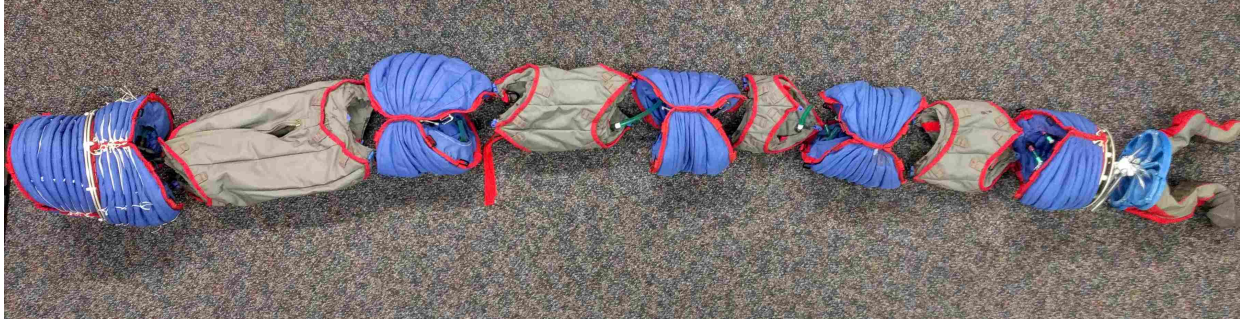
Figure 4.2: We disassembled Kaa to weigh each joint and link for mass and center of mass calculations.
