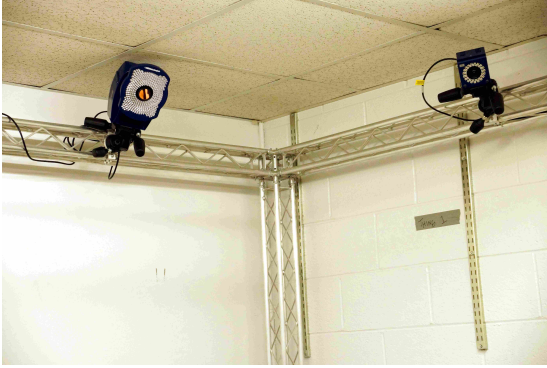
Figure 2.1: Two of the MOCAP cameras used for tracking are shown here (Kestrel on the right and Raptor on the left).
