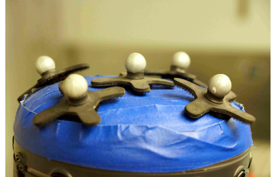
Figure 2.2: IR reflective markers are used to make MOCAP frames.
