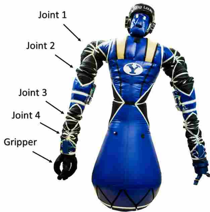
Figure 2.7: This is the inflatable humanoid robot named King Louie used in this work.
