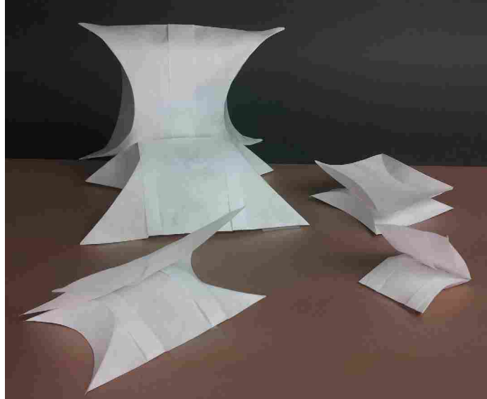
Figure 4.14: Tyvek® models of Configuration 1 with varying values of \alpha and \Theta and a common radius, R , of 5 cm.
