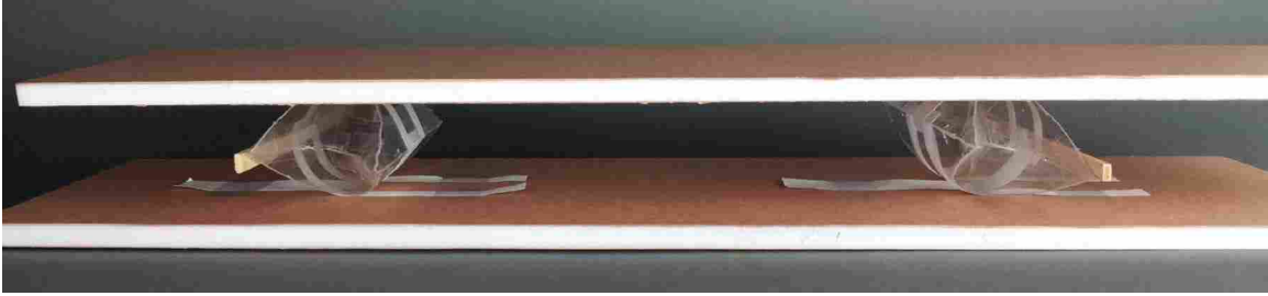
Figure 4.18: Translating platform constructed of polycarbonate cams attached to translating panels via Tyvek® flexible bands.
