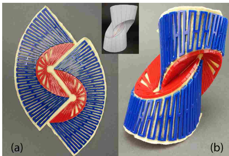
Figure 2.16: Crashing Volcanoes transitioned from paper (origami model is shown in the inset) to acrylic with a fabric backing in its (a) flat state and (b) deployed state.
