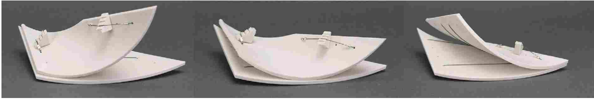
Figure 6.15: 3D printed tangent developable rolling-contact mechanism in multiple positions demonstrating the range of motion.
