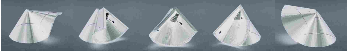
Figure 6.14: 3D printed generalized conical rolling-contact mechanism in multiple positions demonstrating the range of motion.
