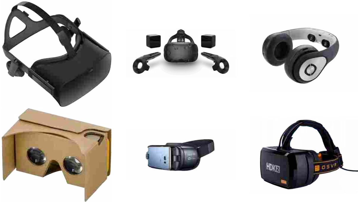
Figure 3.3: Images of various HMDs discussed in Section 3.3.1. Top Left to Right: Oculus Rift, Steam VR/HTC Vive, Avegant Glyph. Bottom Left to Right: Google Cardboard, Samsung Gear VR by Oculus, OSVR HDK. (Images courtesy of Oculus, HTC, Avegant, & OSVR.)
