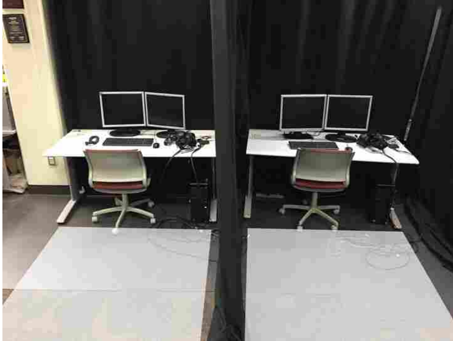
Figure 5.9: The experimental setup used for the study. When using Skype, participants would sit at the computers. When using the VE, participants would stand and walk around in the white areas. A curtain between the two computers was used to block the line of sight between participants.
