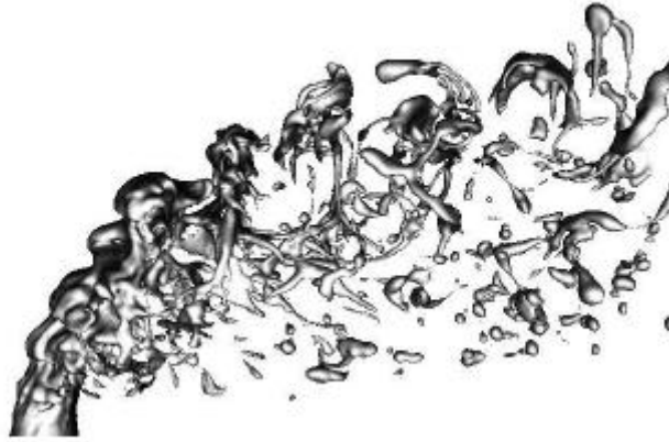
Figure 1-7. Detailed simulation of a jet in crossflow by Pai et al. [43]. It shows the column breaks up at 2-3 diameters downstream of the orifice
