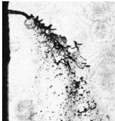
Figure 1-4. Spray image at We=71 , q=7.7 ; Adopted from Wu et al. (1997)
