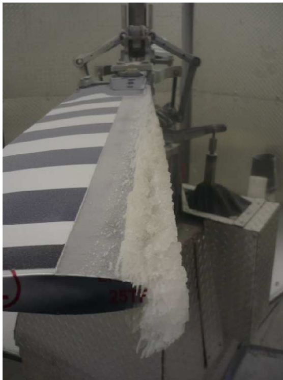
b) Ice shape on Rotor Blade
