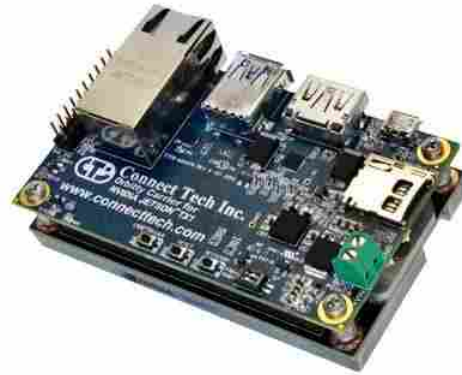
Figure 2.4: NVIDIA Jetson TX2 with an Orbitty carrier board attached [15].
