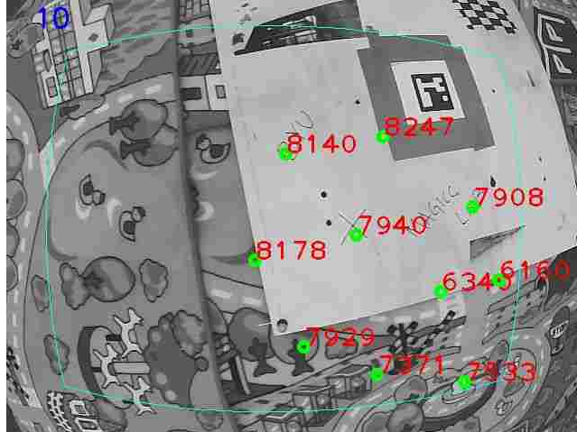
Figure 3.4: A processed camera image from the multirotor UAV’s camera where the landing target vehicle occupies the entire image. The ArUco marker is pictured in the top, right corner of the image. Each green circle shows the tracked location of a visual feature used by the estimator. The red number associated with each visual feature is the unique integer ID assigned by the feature tracker.
