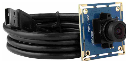
Figure 2.5: ELP USB Camera with a 2.1 mm lens [16].
