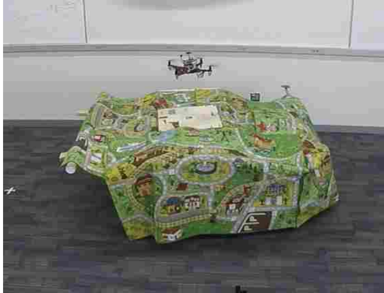
Figure 3.5: Multirotor UAV shown autonomously tracking the landing target vehicle.
